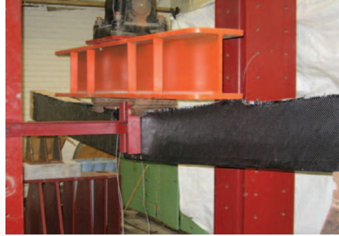
Figure 2: Test setup showing the retrofitted beam approaching failure
