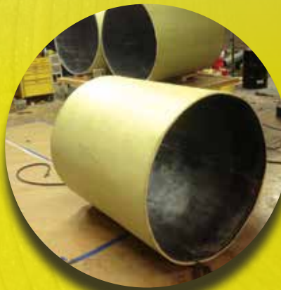
For this pressure pipe repair project, StifPipe™ with an outside diameter of 47 ¼ inch (1200 mm) was constructed with carbon fabric. The pipe was used to slip line the 48 inch (1220 mm) corroded steel pipes with minimal loss of diameter.
