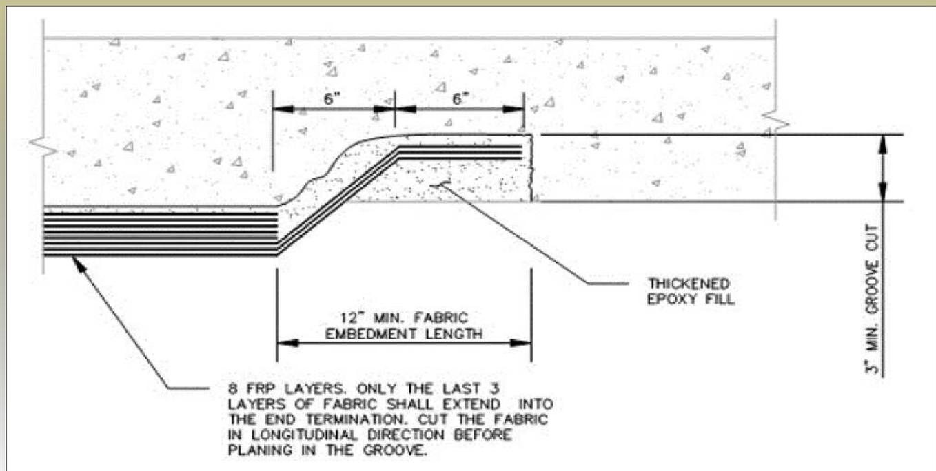
Figure 5. Termination detail for the 8-layer StifPipe® used for the I-35 tunnel repair.
