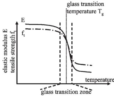
Figure 1 – schematic sketch of temperature-dependent tensile strength and elastic modulus of epoxy resin adhesives
