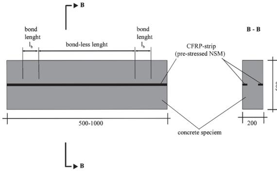
Figure 6 – test specimen for analyzing the structural behaviour of prestressed NSM reinforcement
