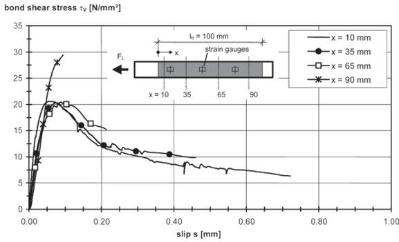
Figure 4 – shear-slip-relationships for different sections of the bond length (bond length  $l_b = 100$  mm, distance  $a_r = 150$  mm) (Blaschko 2003)
