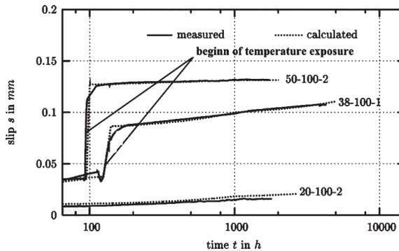
Figure 8 – total slip between strip and concrete at the inner end of the bond length – experiment and calculation
