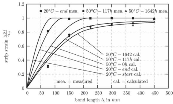
Figure 11 – strip strain along the bond length – experiment and calculation
