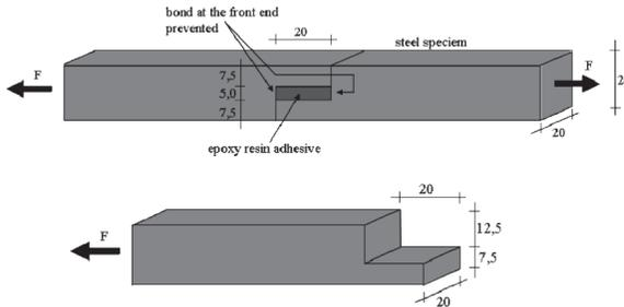
Figure 5 – lap shear test specimen according to DIN 54451-11.1978
