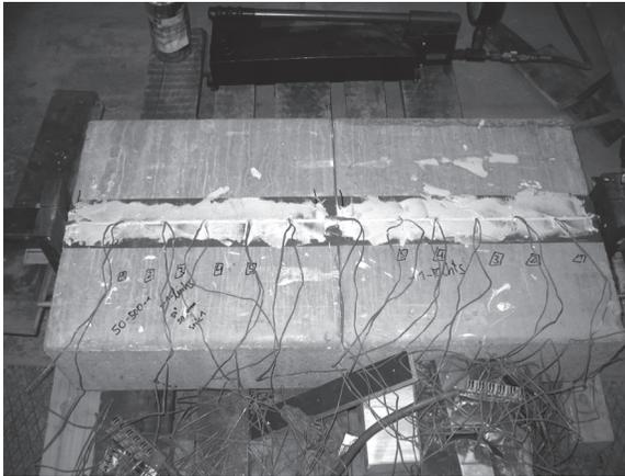
Figure 7 – test specimen with a bond length  $l_b$  of 450 mm with strain gauges within the bond length  $l_b$  – while curing
