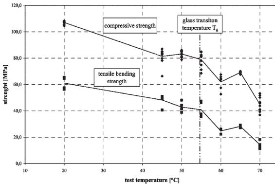
Figure 2 – compressive and tensile bending strength of epoxy resin with rising test temperature
