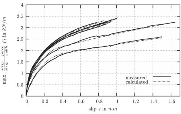
Figure 10 – strip-force-slip-relationship with varying geometrical parameters – experiment (Blaschko 2001) and calculation
