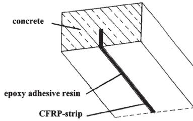
Figure 3 – near surface mounted CFRP strips glued into slits (Blaschko and Zilch 1999)
