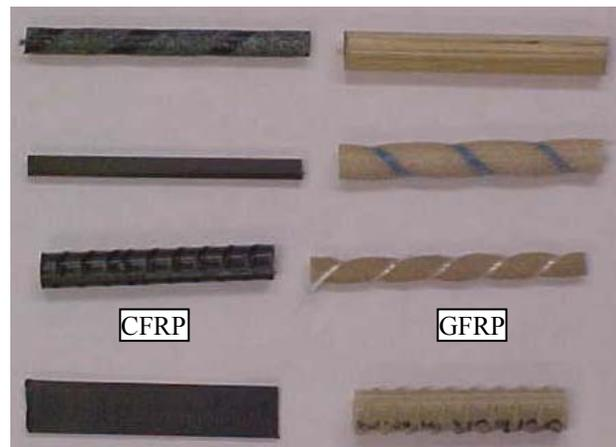
**Fig. 2 Carbon and Glass FRP Rods**
