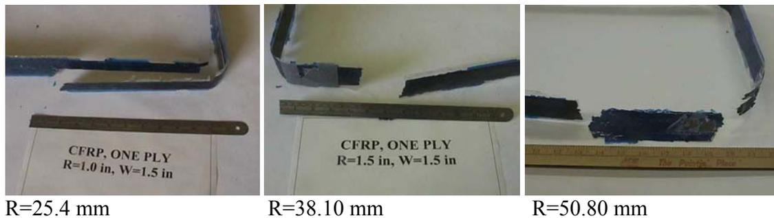
Fig. 7 Failure modes of CFRP laminates
