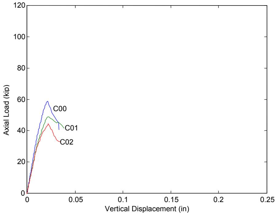
**Figure 3.** Load-Deflection Curves for Specimens without FPR Jacket
