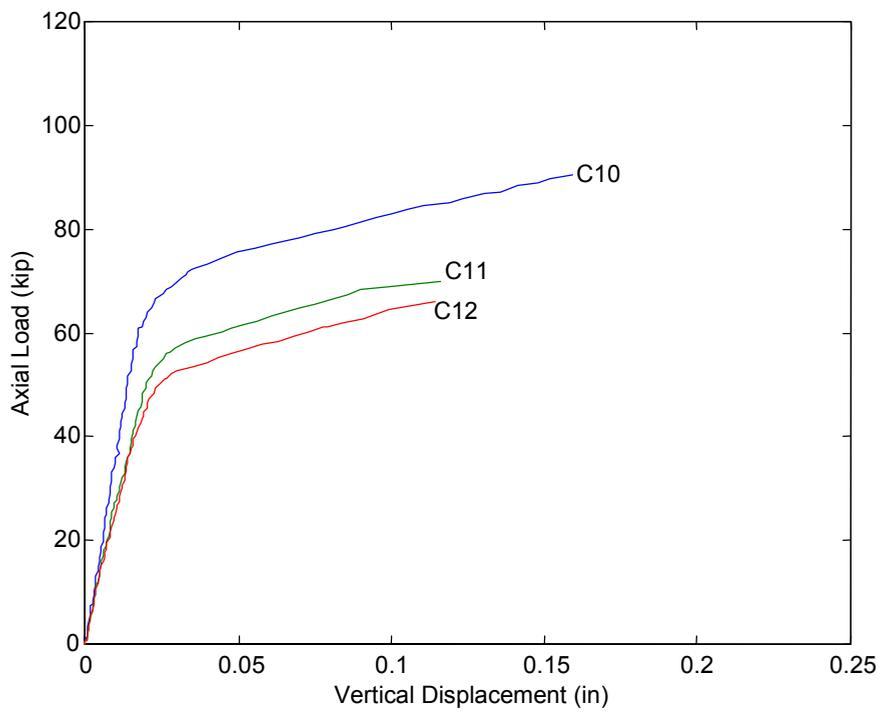
**Figure 4.** Load-Deflection Curves for Specimens with One Layer of FRP Jacket
