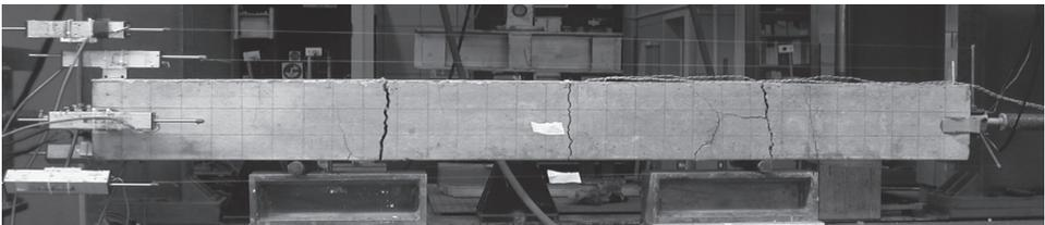
Figure 1— Testing arrangement of horizontally loaded tension member
