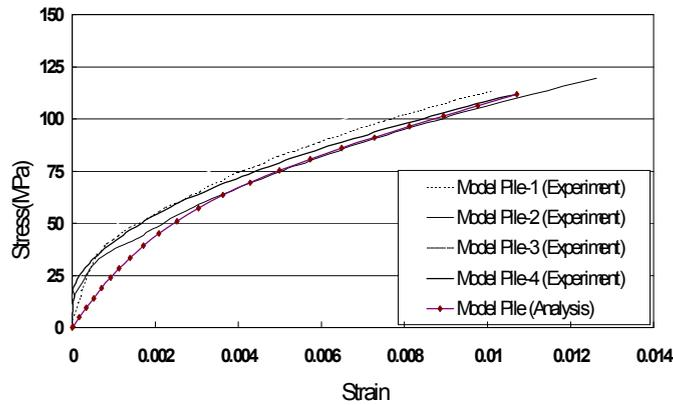
**Figure 13.** Predicted stress-strain relation compared with test results shown in Figure 3
