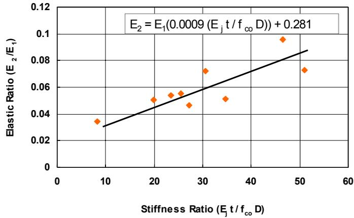
**Figure 12.** The relation between elastic modulus ratio and stiffness ratio
