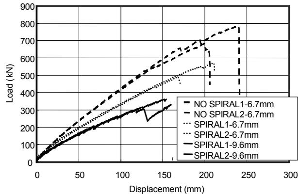
**Figure 19.** Load-displacement curves of test piles
