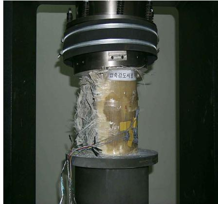
**Figure 2.** Test setup under compression for concrete-filled short composite tubes
