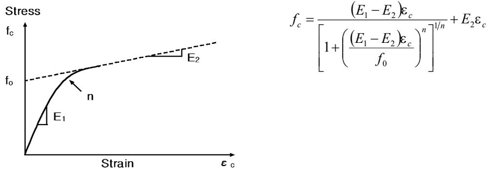
Figure 10. Constitutive model for FRP-encased concrete (Samaan et al., 1998)
