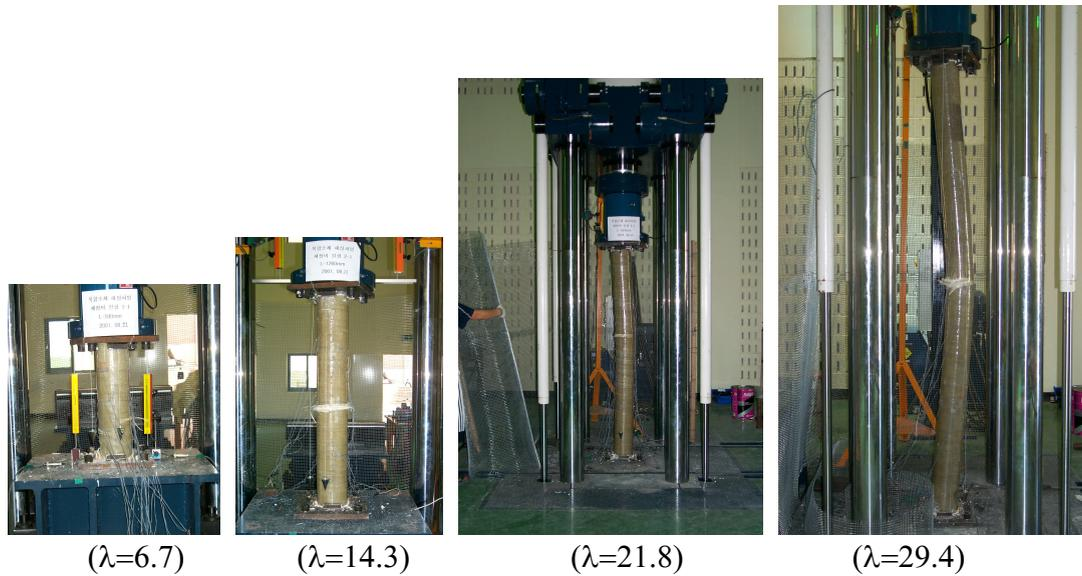
**Figure 15.** Typical failure pattern of a pile under buckling test
