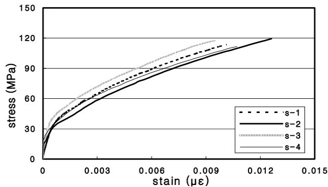
**Figure 3.** Stress-strain curves in axial direction
