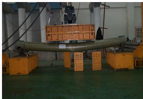
**Figure 18.** Experimental setup for large scale pile test
