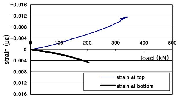
**Figure 9.** Load-strain curve (P-6)
