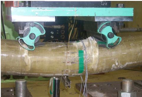
(a) Tension failure (P-1)
