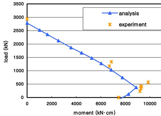
**Figure 14.** Computed P-M interaction diagram and experimental results
