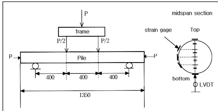
Figure 5. Pure flexural and axial-flexural test setup
