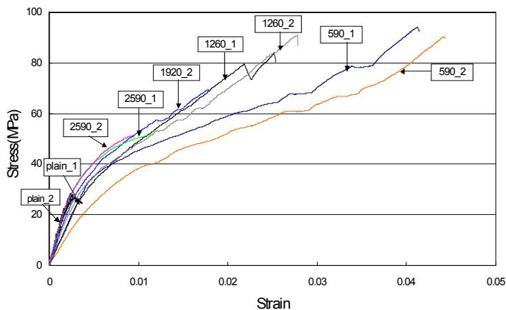
**Figure 16.** Stress-strain responses of piles
