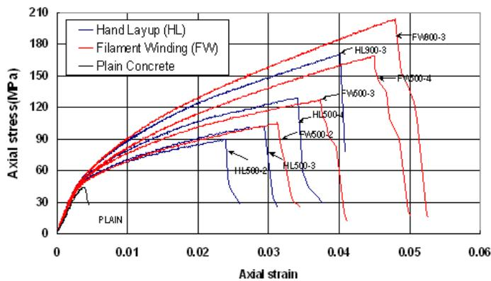
Figure 11. Stress-strain relations obtained by varying tube thickness
