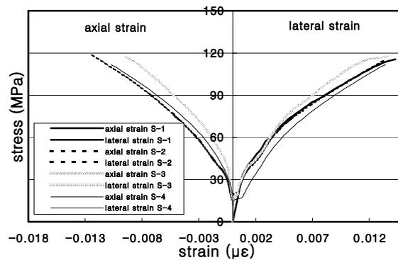
**Figure 4.** Strains in axial and lateral directions
