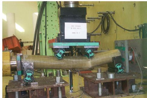
(b) Compression failure (P-6)
