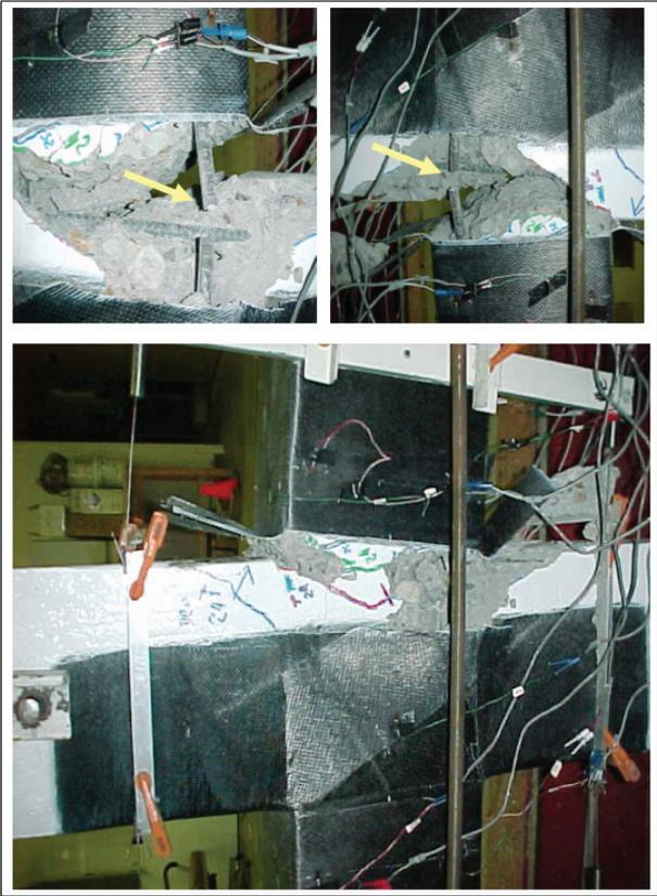
Figure 11— Ultimate Failure Mode of Carbon/Epoxy Retrofitted Specimen.
