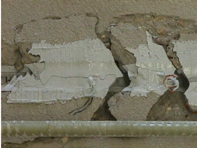
**Figure 3.43. Crack Pattern in Specimen G4D24c After Failure**
