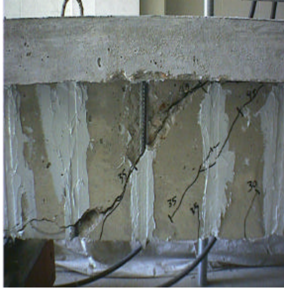
Figure 5.7. Failure of Beam B90-7
