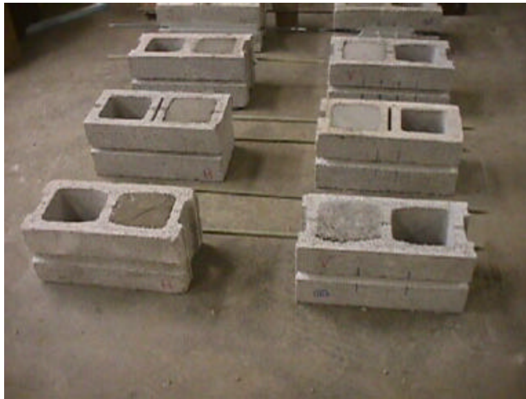
Figure 4.4. Concrete Blocks Before Preparation
