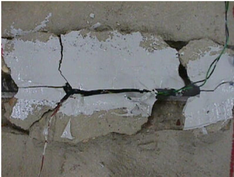
**Figure 3.44. Crack Pattern in Specimen C3D24b After Failure**
