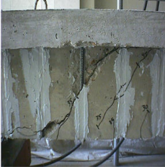
Figure 5.7. Failure of Beam B90-7
