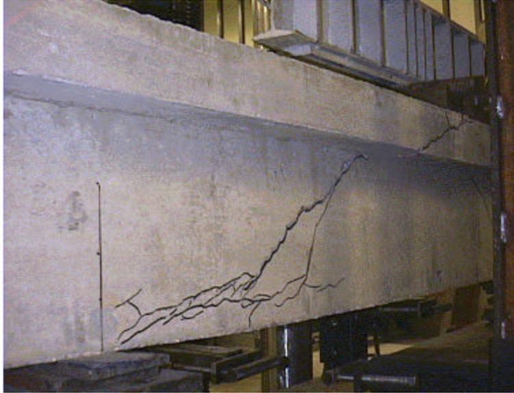
**Figure 5.6. Failure of Beam BV**
