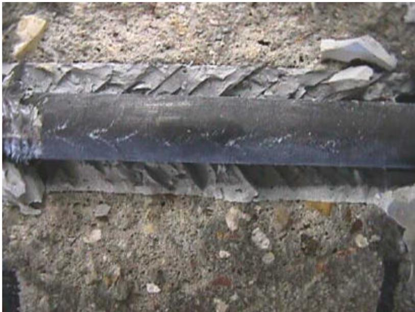
**Figure 3.42. Internal Cracks in Specimen C3S6a**
