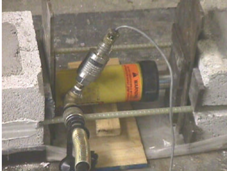
Figure 4.8. Detail of Hydraulic Jack and Pressure Transducer
