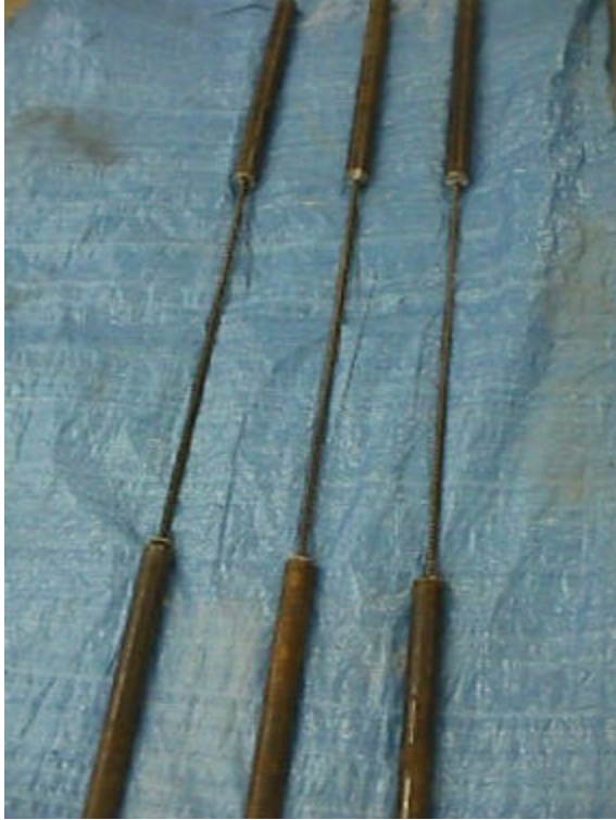
Figure 2.2. Specimens of CFRP Deformed Rods Ready for Testing
