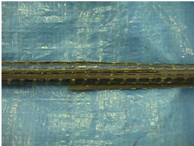
Figure 2.5. Tensile Failure of CFRP No. 3 Deformed Rods
