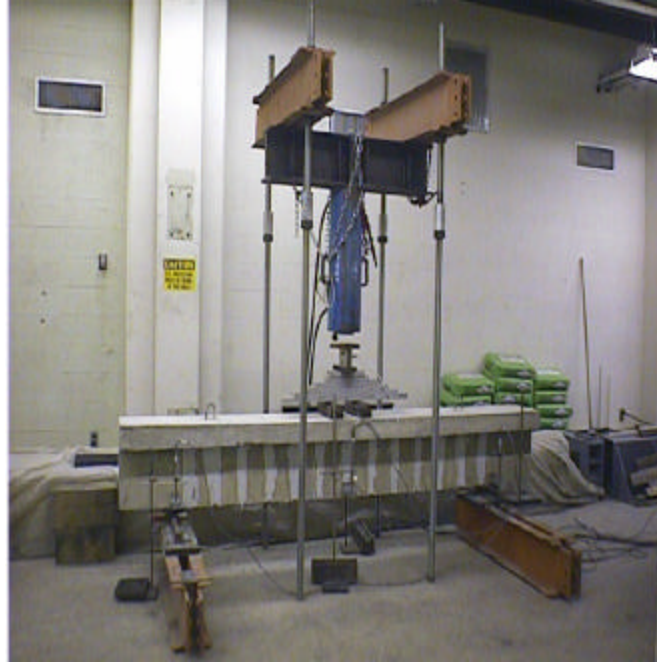
Figure 5.5. Test Setup of Beam B90-7
