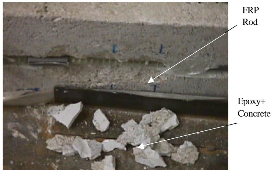
**Figure 4.10. Specimen After Splitting Failure**
