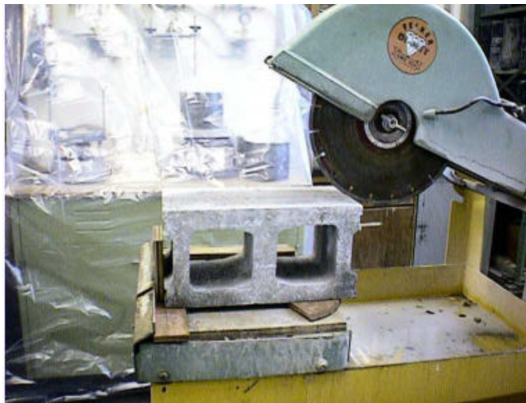
Figure 4.3. Cutting of the Grooves on the Concrete Blocks
