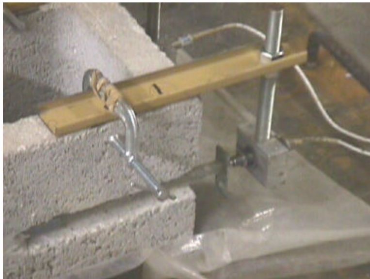
Figure 4.9. Detail of the LVDTs
