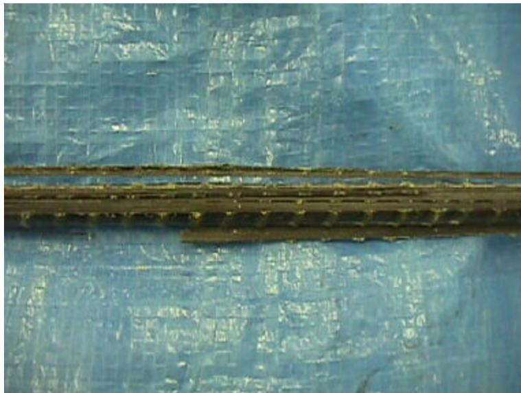
**Figure 2.5. Tensile Failure of CFRP No. 3 Deformed Rods**
