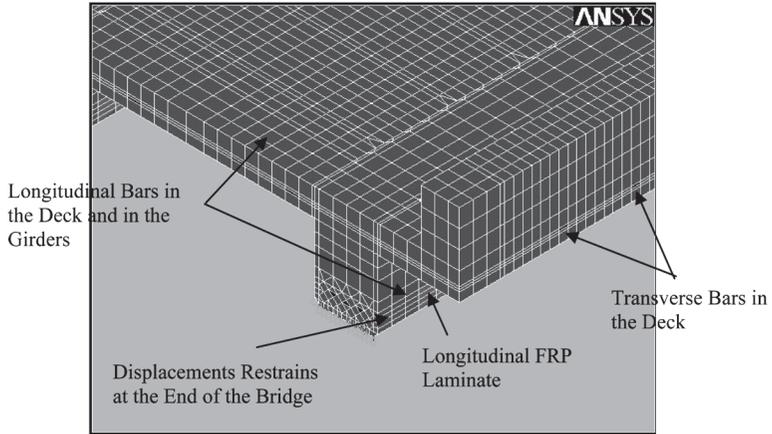
a) Details of the Steel Reinforcement and Boundary Conditions
