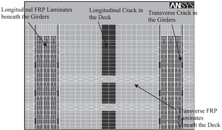
b) Details of the FRP Strengthening (Bottom View)
