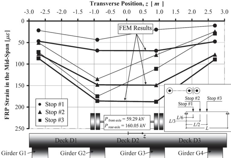
Fig. 13 — Mid-Span Strain in the FRP Fastened on the Bridge No. 1330005 Girders at Mid-Span, Pass #3 (Comparison of Experimental and Analytical Results)
