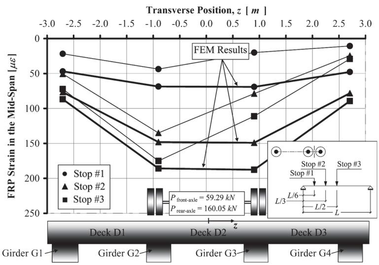
Fig. 13 — Mid-Span Strain in the FRP Fastened on the Bridge No. 1330005 Girders at Mid-Span, Pass #3 (Comparison of Experimental and Analytical Results)
