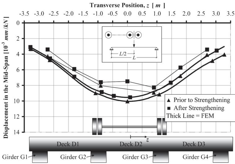
Fig. 12 — Mid-Span Displacement, Pass #3 and Rear Axle in the Mid-Span of Bridge No. 1330005 (Comparison of Experimental and Analytical Results)
