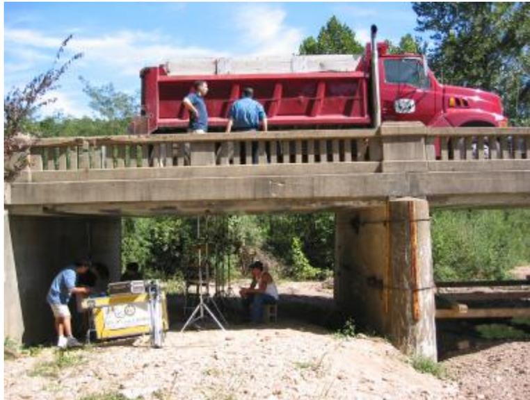
Figure 4-1 – Load Test with H20 Truck
