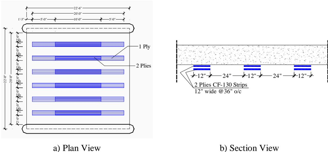
Figure 3-2 – Strengthening with Laminates on Span 1 and 3
