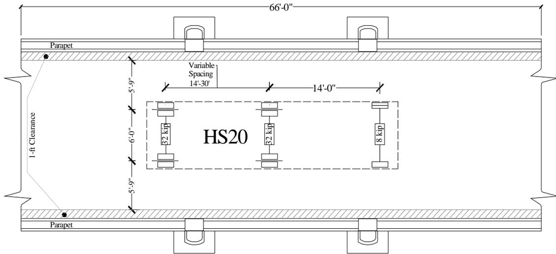
Figure 2-2 - Truck Load and Truck Lanes
