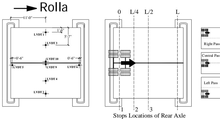
Figure 4-3 – LVDTs Positions and Truck Stops
