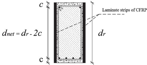
Figure 7 – Data for the near surface mounted shear strengthening technique
