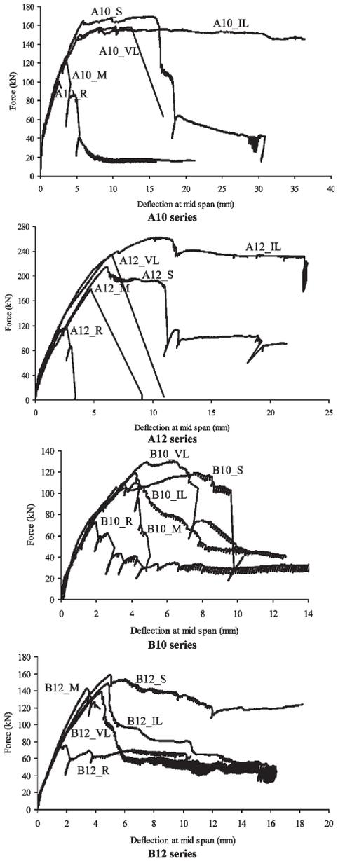
Figure 3 – Force-deflection relationship of the four tested beams series
