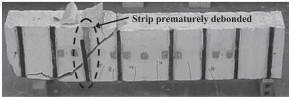
Figure 5 — Failure of A10\_M beam
