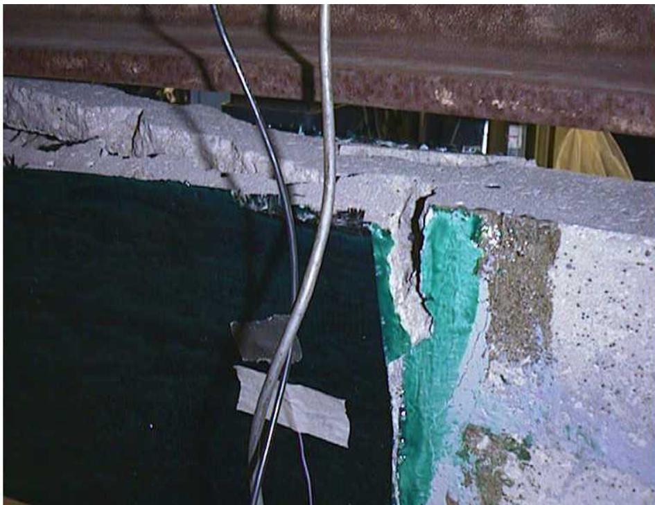
**Figure A-12.** Ultimate failure of Specimen B-CF3 (CFRP 90°/0°)
