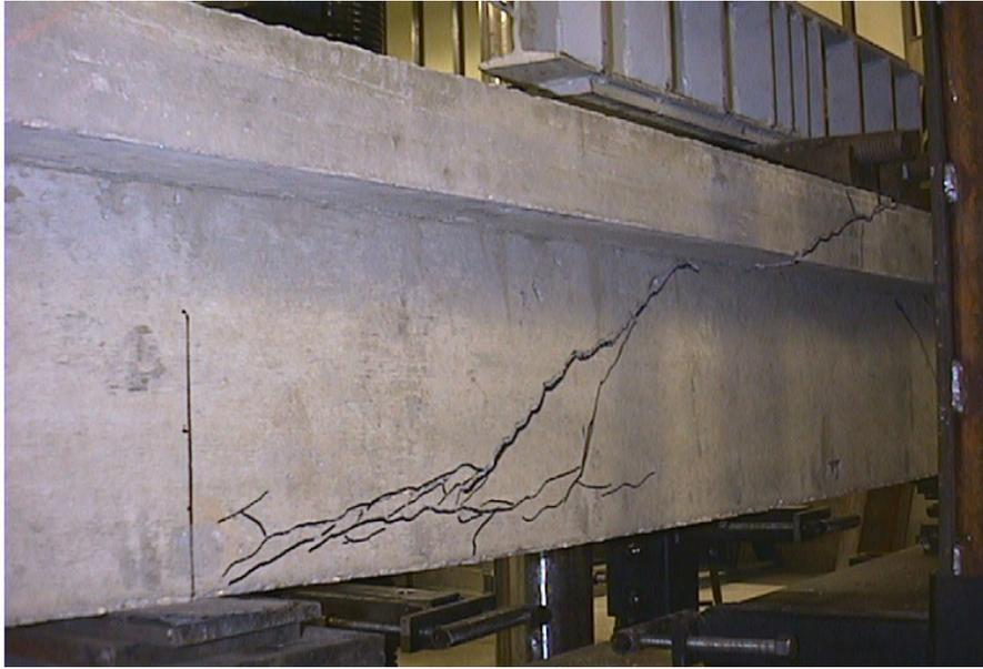
**Figure 4-22.** Ultimate failure of Specimen C-BT1
