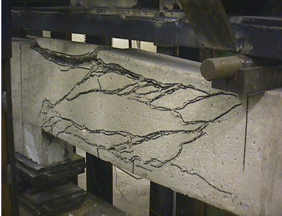
**Figure A-8.** Ultimate failure of Specimen B-CO1 (control specimen)
