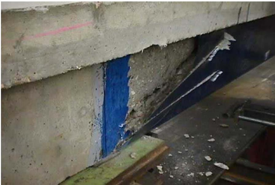
**Figure 4-23.** Ultimate failure of Specimen C-BT2
