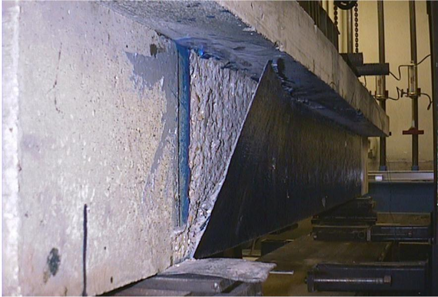
**Figure 4-25.** Ultimate failure of Specimen C-BT3
