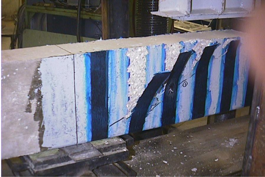
**Figure 4-7.** Ultimate failure of Specimen A-SO3-2
