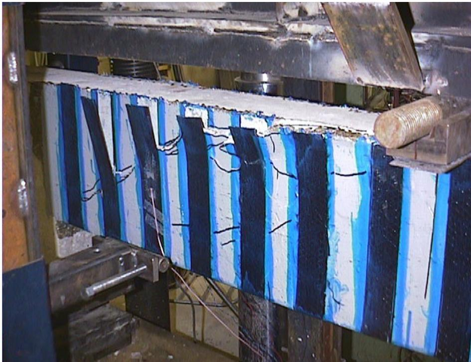
**Figure A-9.** Debonding failure of Specimen B-CO2 (U-wrap strips)
