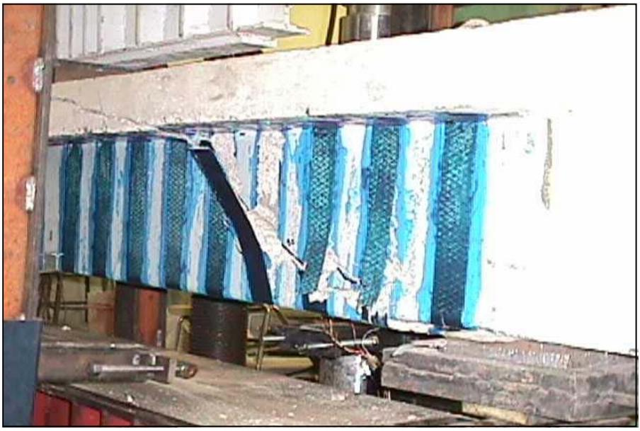
**Figure 4-26.** Ultimate failure of Specimen C-BT4
