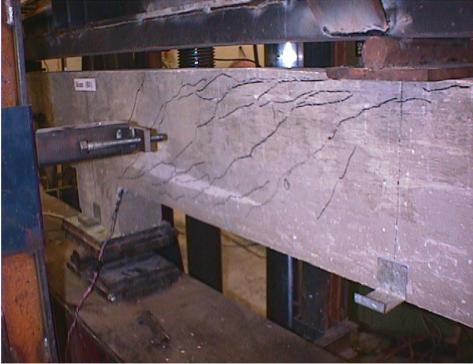
**Figure A-6.** Ultimate failure of Specimen B-CW1 (control specimen)
