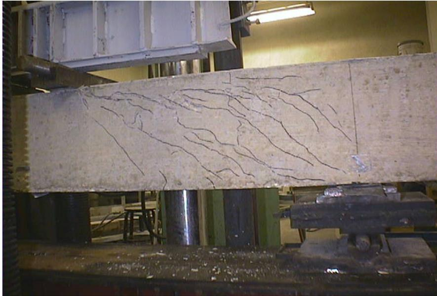
**Figure 4-1.** Crack pattern at ultimate failure of Specimen A-SW3-1
