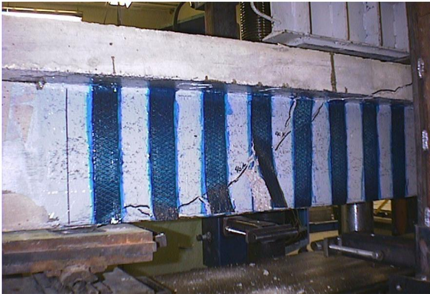
**Figure 4-28.** Ultimate failure of Specimen C-BT5
