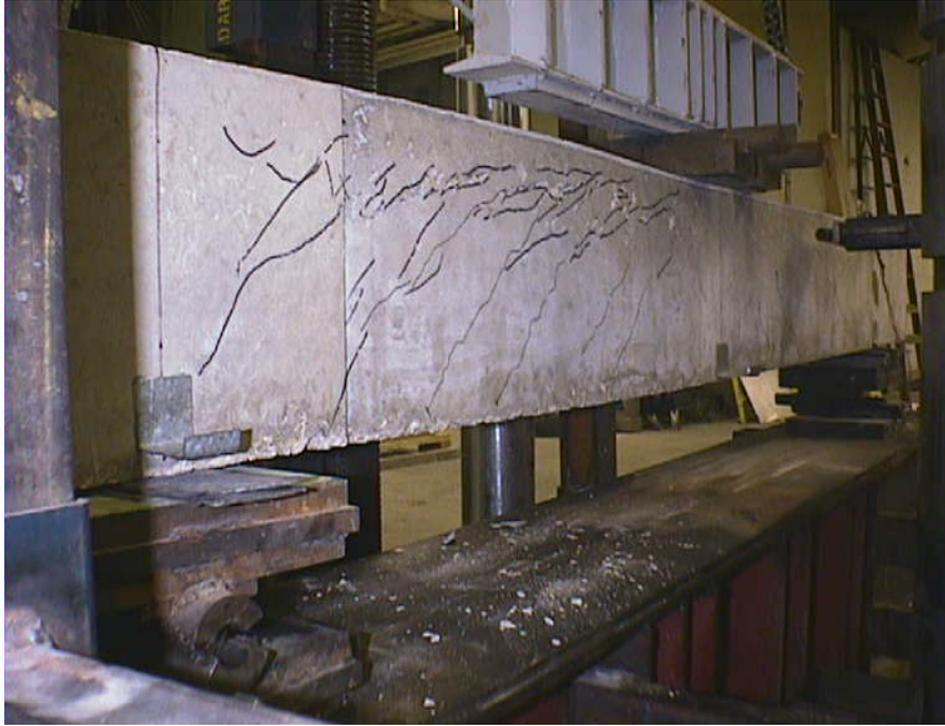
**Figure A-1.** Ultimate failure of Specimen A-SW4-1 (control specimen)
