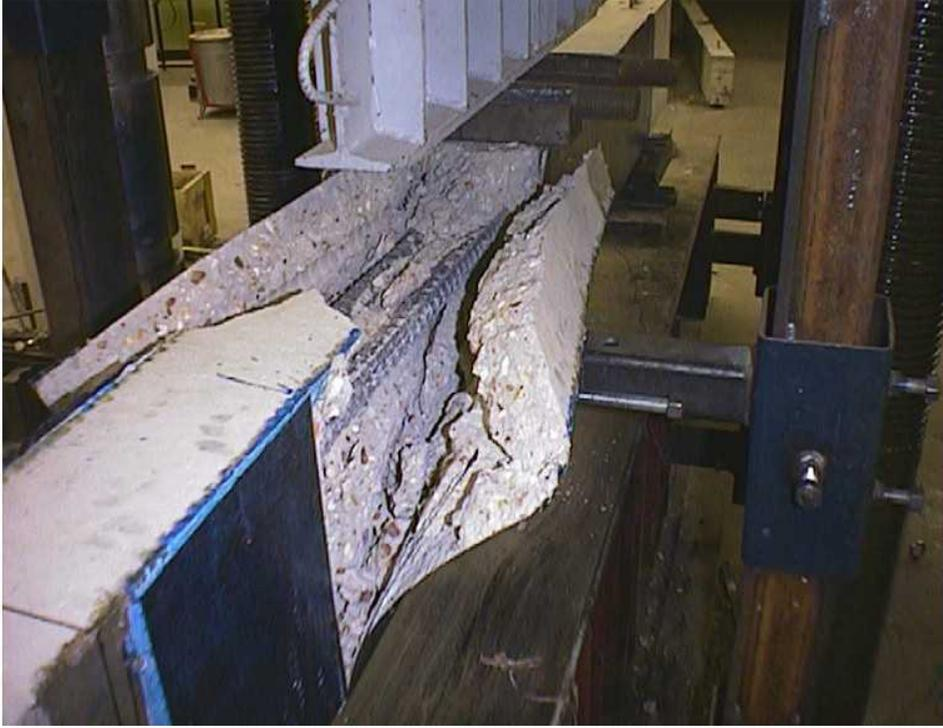
**Figure A-5.** Splitting failure of Specimen A-SO4-3 (Continuous U-wrap)
