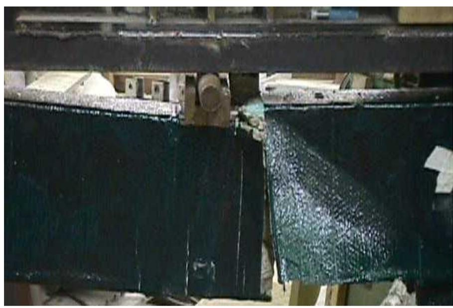
Figure 4-21. Ultimate failure of Specimen B-CF4
