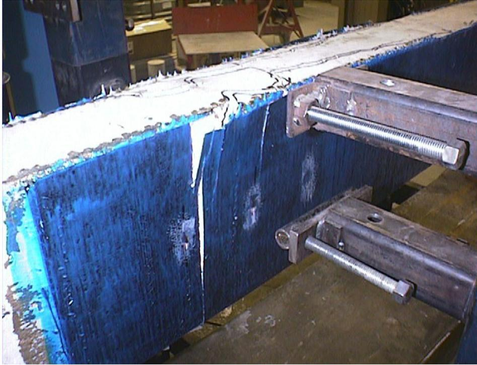
**Figure A-10.** Ultimate failure of Specimen B-CO3 (continuous U-wrap)
