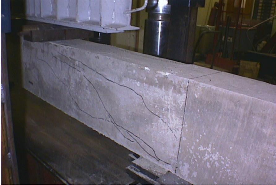
**Figure 4-6.** Crack pattern at ultimate failure of Specimen A-SO3-1
