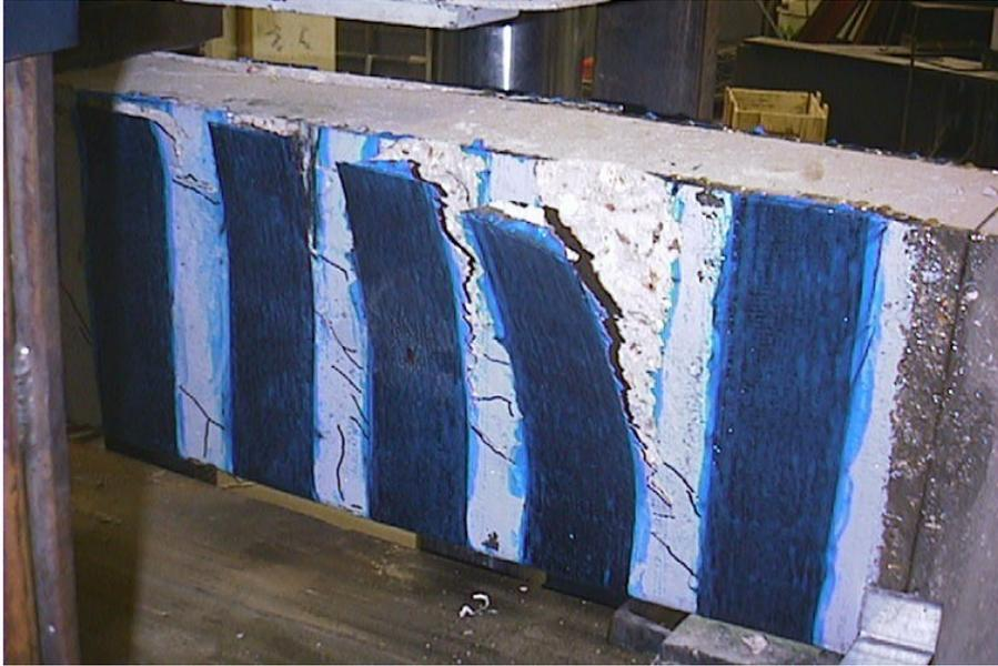
**Figure 4-9.** Ultimate failure of Specimen A-SO3-3
