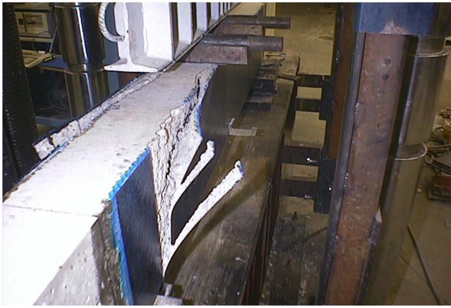
Figure 4-10. Ultimate failure of Specimen A-SO3-4
