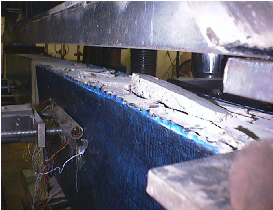
**Figure A-7.** Ultimate failure of Specimen B-CW2 (CFRP 90°/0°)
