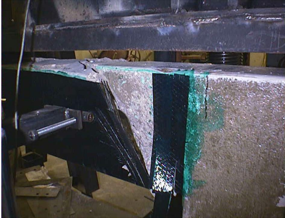
**Figure A-11.** Ultimate failure of Specimen B-CF2 (continuous U-wrap)
