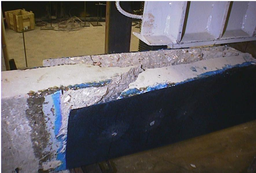
**Figure 4-12.** Splitting failure of Specimen A-SO3-5
