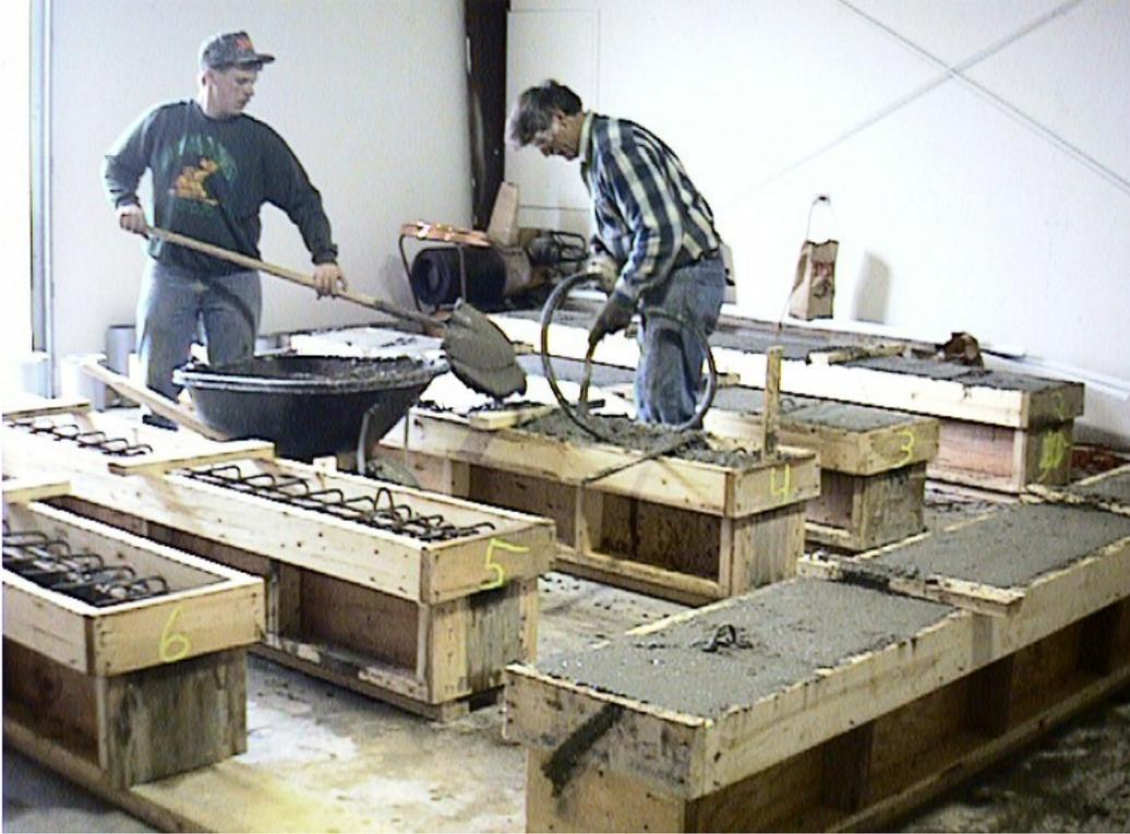
**Figure 3-10.** Casting of beam specimens of Series C
