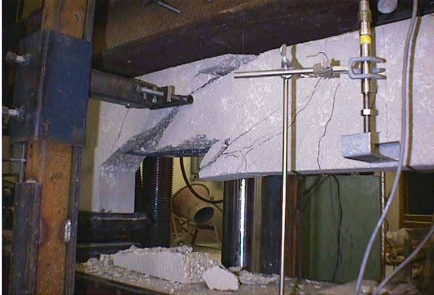
**Figure 4-19.** Ultimate failure of Specimen B-CF1
