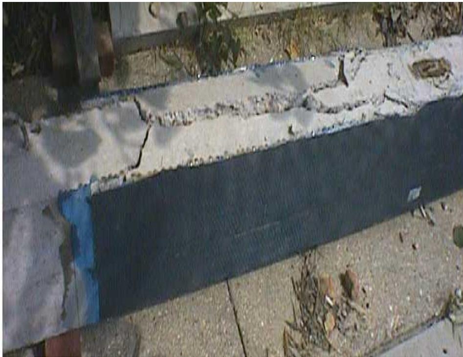
**Figure A-2.** Splitting failure of Specimen A-SW4-2 (CFRP 90°/0°)
