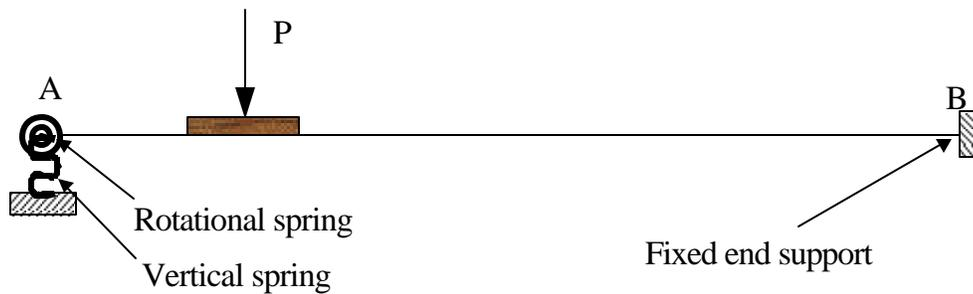
Figure 5.6: Typical Loading and Support Configuration for Design
