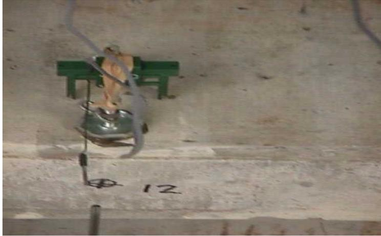
Figure 6.4: Extensometer
