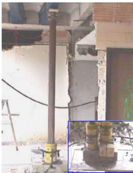
Figure 6.6: Load setup
