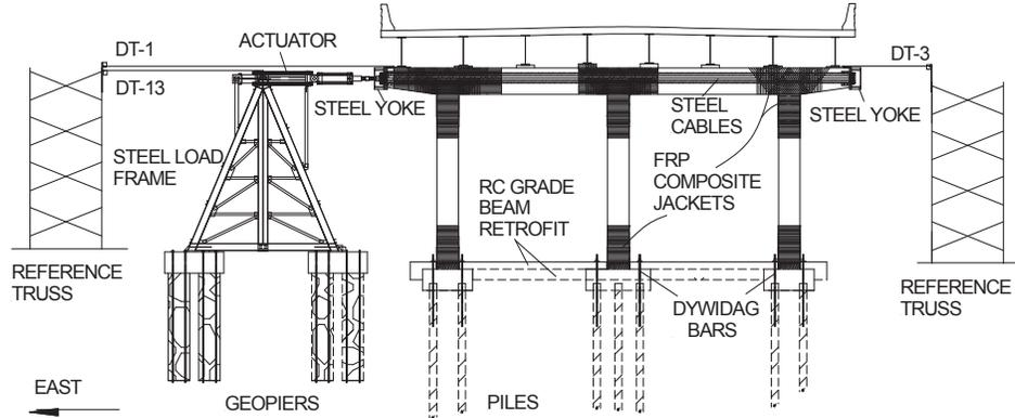
Figure 12 - Loading condition for typical bridge pier - 2000 tests.
