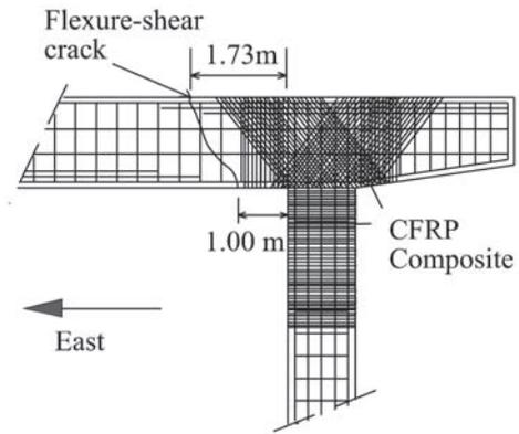
Figure 18 - Flexure-shear crack at cap beam of West column at 6% drift ratio – 2000 tests.
