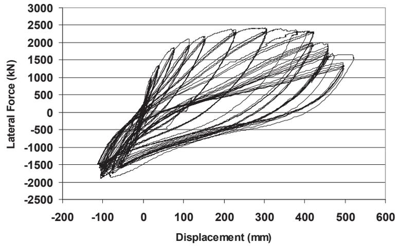
Figure 16 - Hysteresis loops for pier with RC grade beam and CFRP retrofit – 2000 tests.
