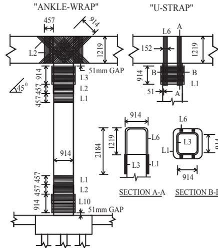
Figure 9 - Details of CFRP composite layout for retrofit of bridge pier – 1998 tests.
