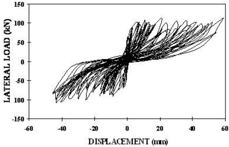
Figure 2 - Hysteresis for as-built beam-column joint.
