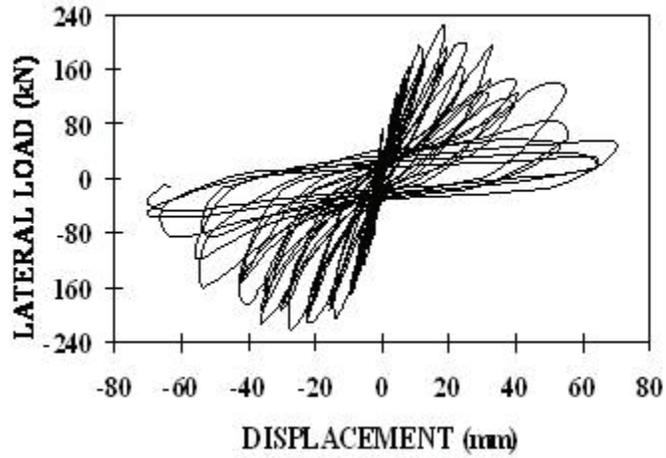
Figure 3 - Hysteresis for beam-column joint rehabilitated with CFRP composites.
