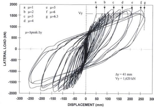
Figure 11 - Hysteresis for CFRP retrofitted pier - 1998 tests.
