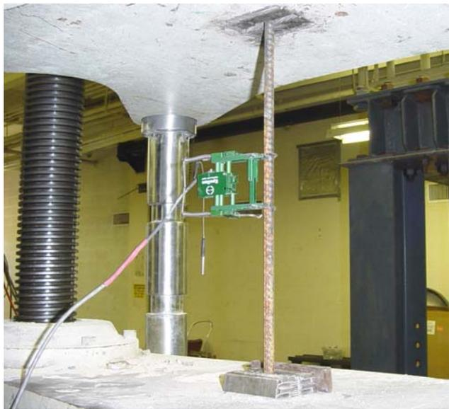
Figure 4.4. Steel Rebar Tensile Coupon Test
