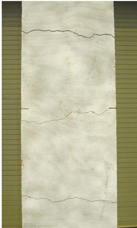
Figure 4.14. Phase II Typical Specimen Crack Pattern
