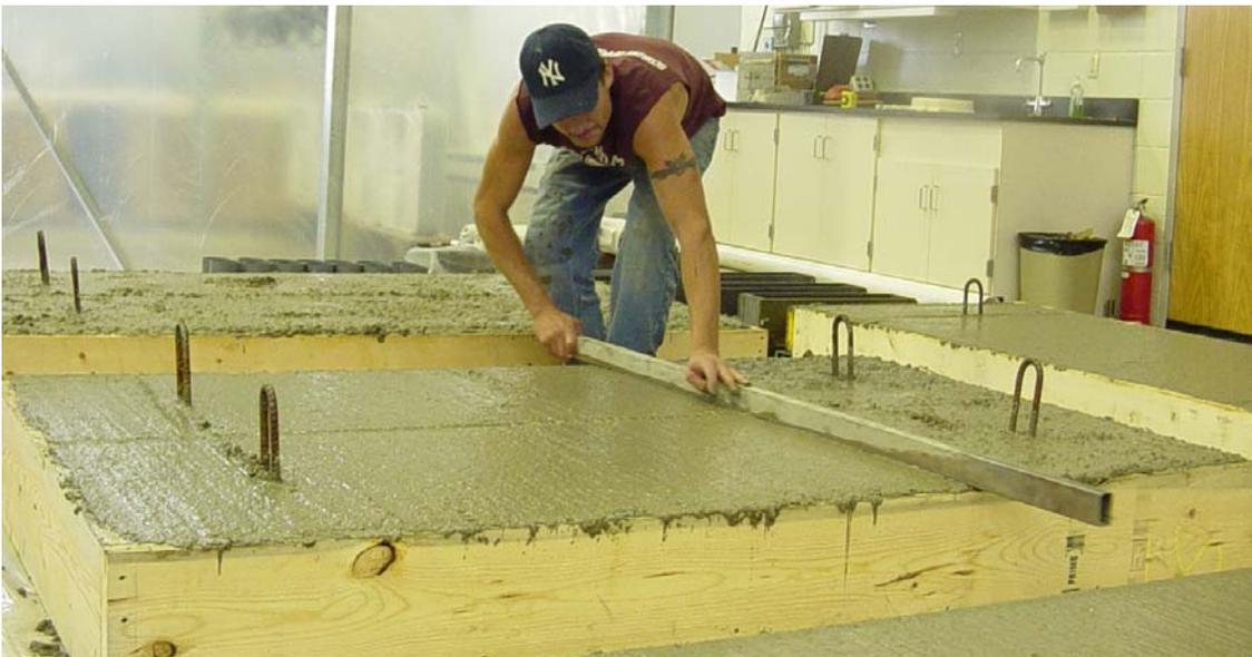
Figure 3.9. Specimen Leveling of Fresh Concrete
