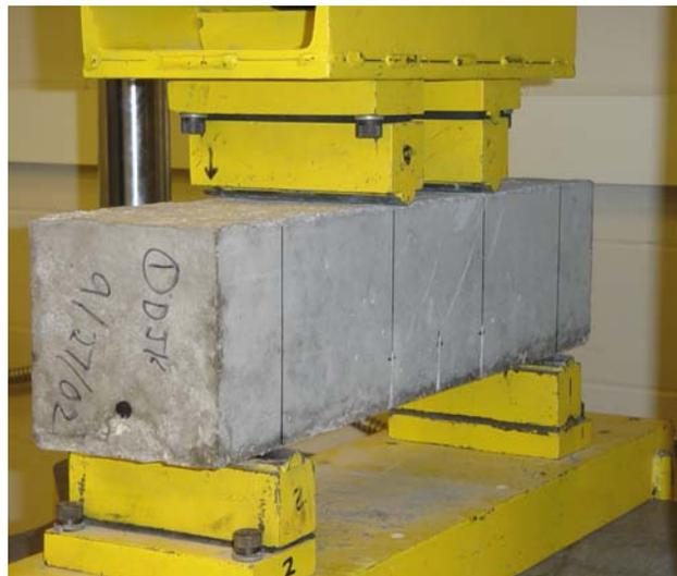
Figure 4.3. Third-Point Loading of Flexural Beam
