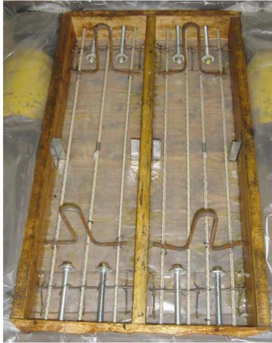
Figure 3.1. Common Phase I Specimens Before Concrete Placement
