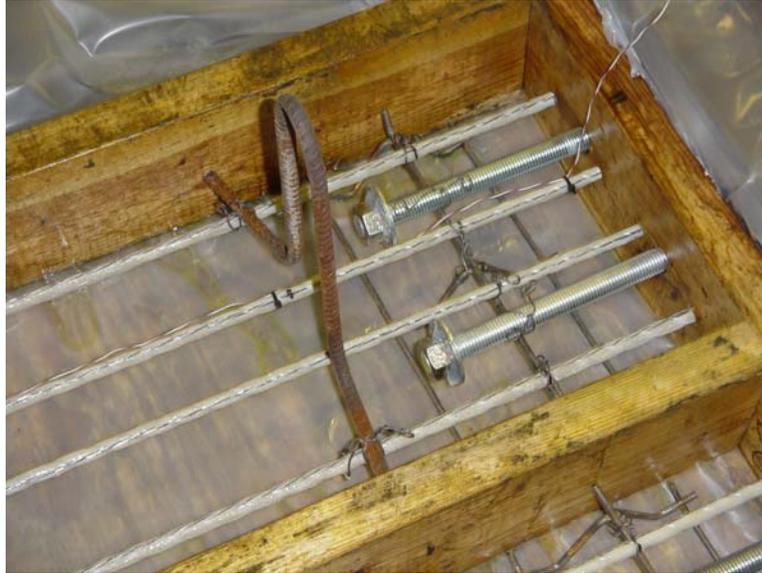
Figure 3.3. Embedded Threaded Rod with Hex Nut and Washer
