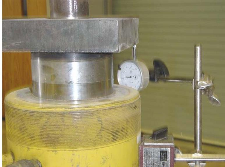
Figure 3.15. Phase II Method of Measuring Deformation
