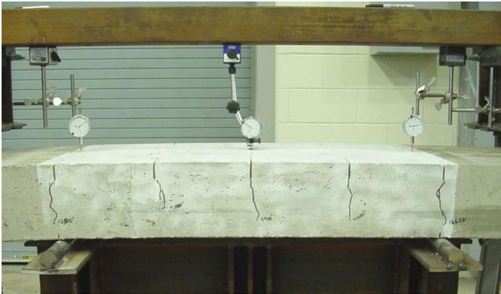
Figure 3.16. Phase III Method of Measuring Deflection
