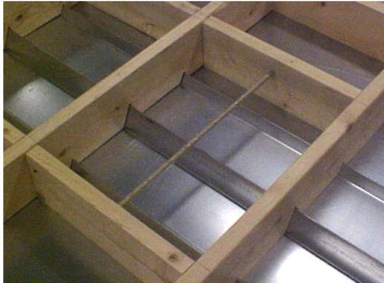
Figure 3.18. Specimen Forms to Investigate Plastic Shrinkage Cracks
