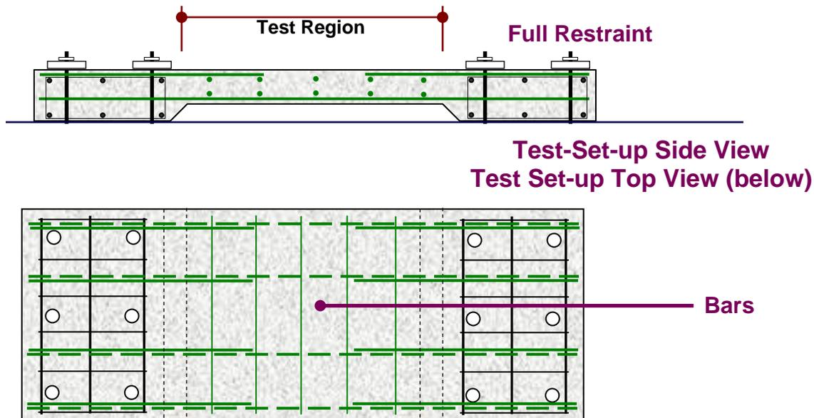
Figure 1. Test Set-Up for Restrained Panel Tests
