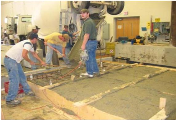
Figure 3. Series 1 Specimen Casting
