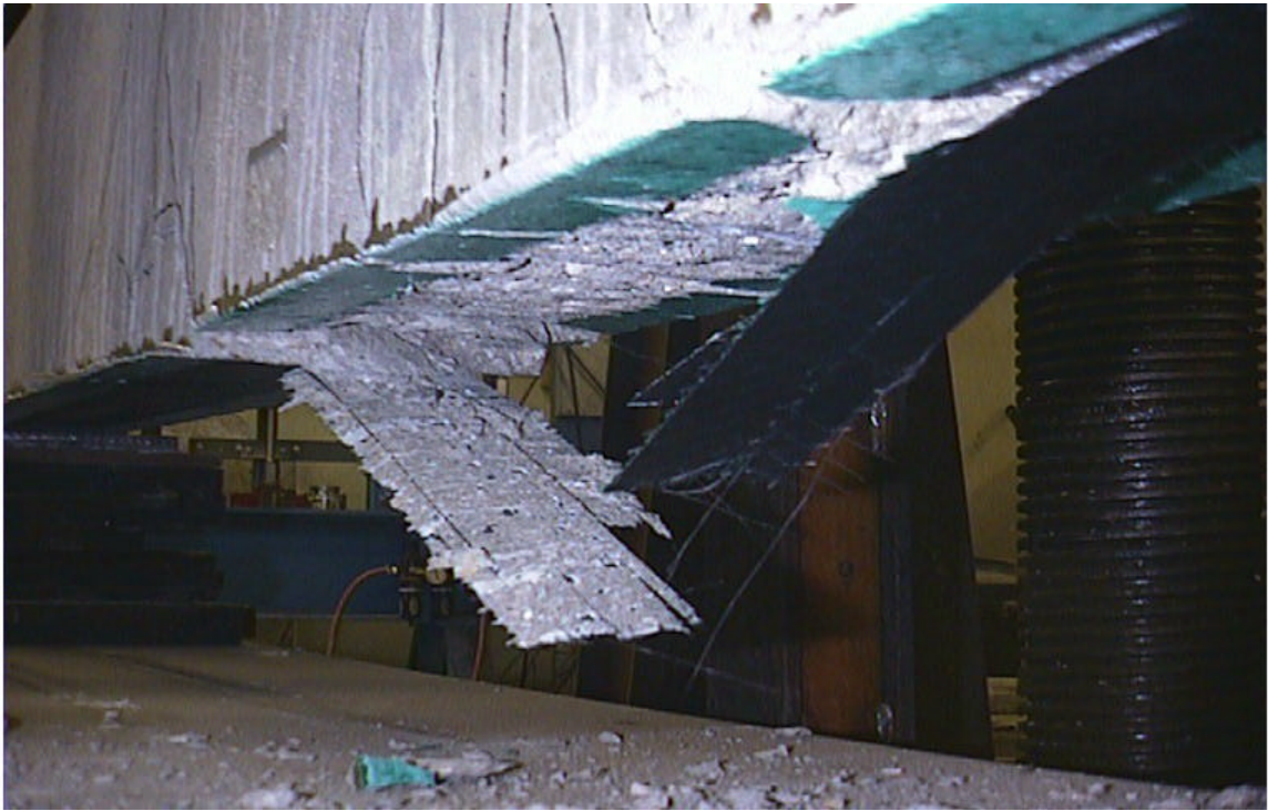
Figure B.7. Failure in Beam B2
