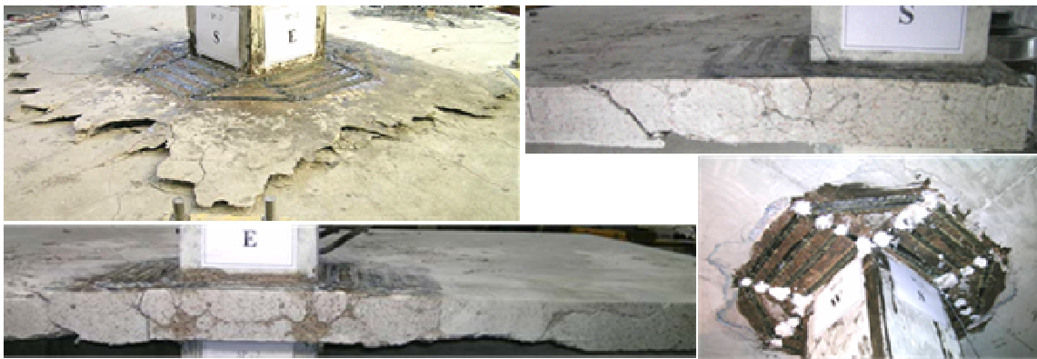
Figure 9. Failure surface of SP-2.
