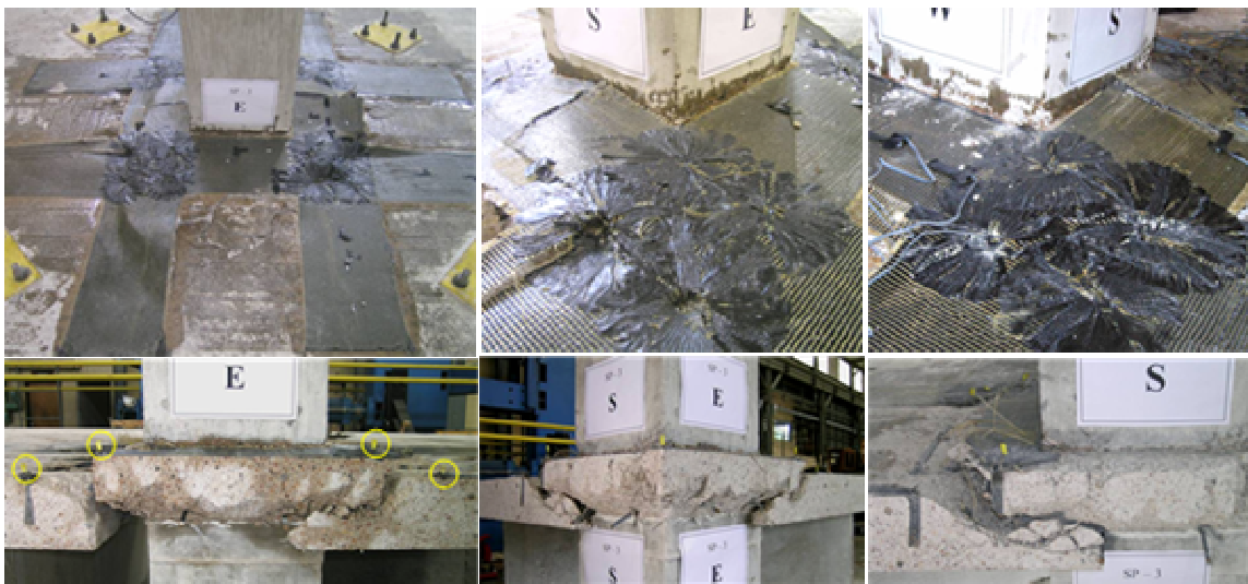
Figure 10. Failure surface of SP-3.
