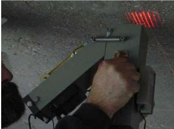
Figure 16. Laser Profilometer for surface roughness
