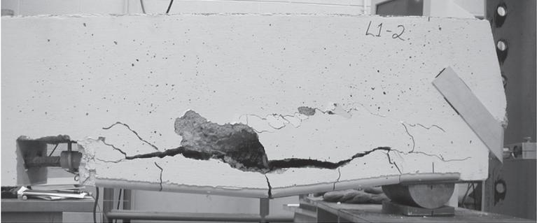
Figure 4 – Bond Splitting Failure Crack Pattern, Series L1
