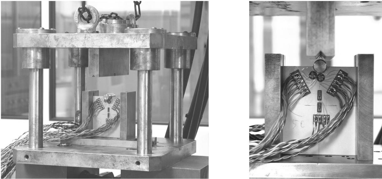
**Figure 1.** (a) Pin-bearing test rig with an unloaded specimen, (b) close-up of indenter, strain rosettes and anti-buckling support with a 0.2 mm clearance specimen.
