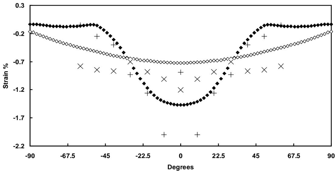
**Figure 9.** Comparison of strains for  $0^\circ$  material orientation.
