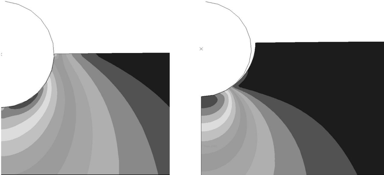
**Figure 5.** Minimum principal strain contour plots; left figure no clearance, right figure 1 mm clearance.
