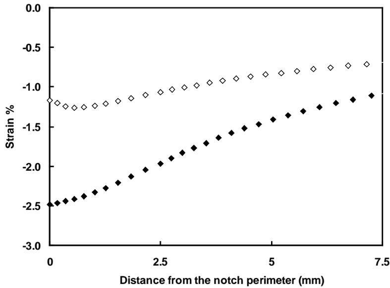
**Figure 8.** Minimum principal strains on bearing plane from notch perimeter.
