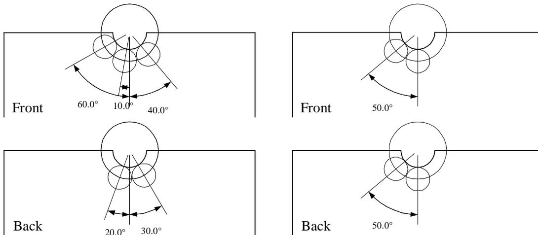
**Figure 2.** Locations of the 2 mm strain rosettes.
