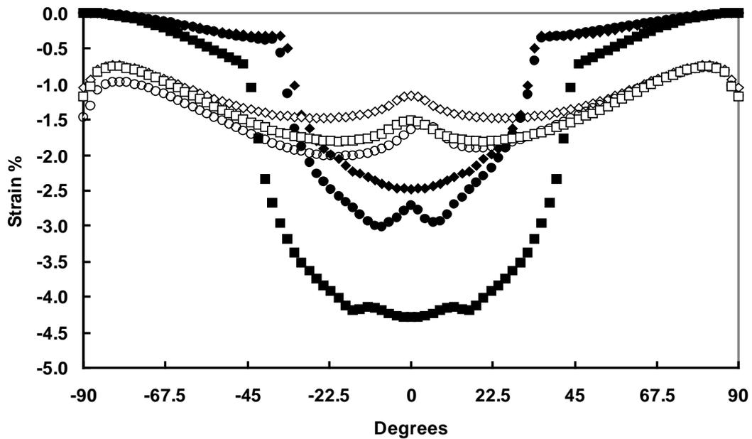
Figure 7. FEA minimum principal strains on notch perimeter.
