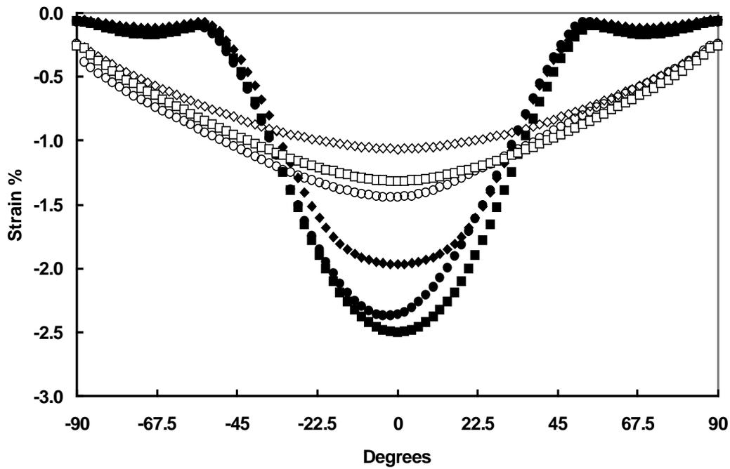
Figure 6. FEA minimum principal strains at 2.5 mm from notch perimeter.
