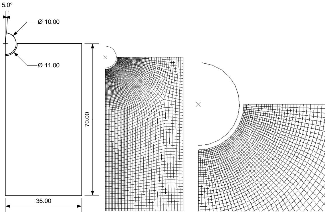
**Figure 3.** Dimensions and mesh specification for plate specimen.
