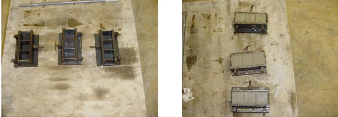
Figure 3.2. Casting of Mortar Cubes
