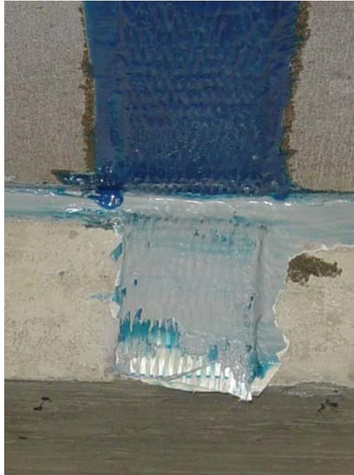
Figure 4.21. #2 GFRP Bar Inserted into Groove
