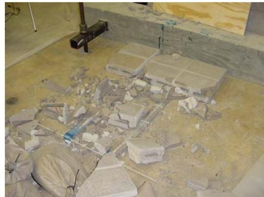
(f) Masonry Attached to Laminate
