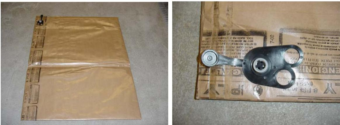
Figure 4.1. Airbag Used for Loading
