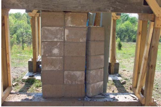
Figure 5.15. Wall #2 Failure
