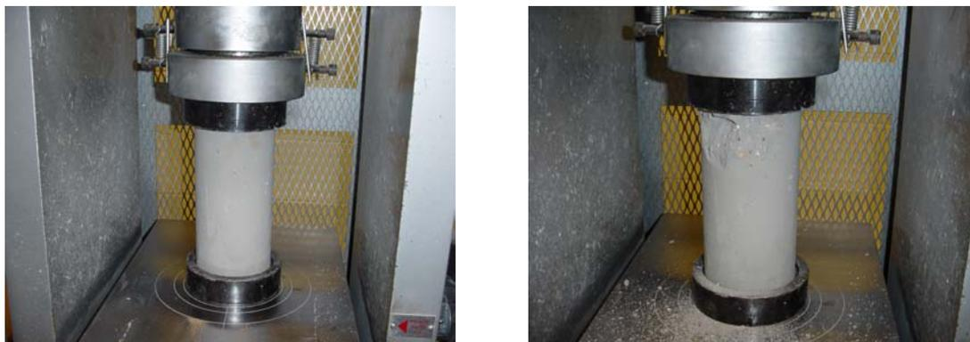
Figure 3.1. Testing of Concrete Cylinders
