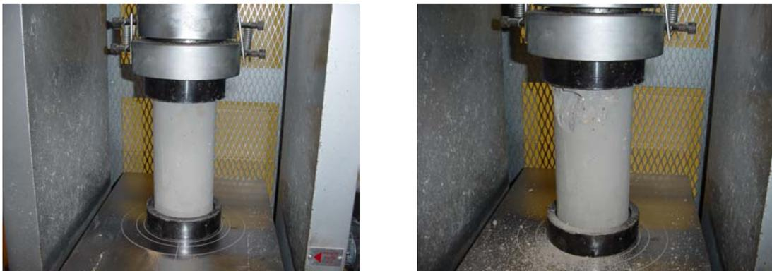
Figure 3.1. Testing of Concrete Cylinders
