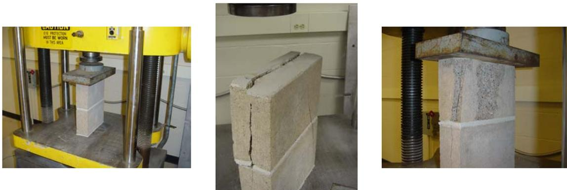
Figure 3.5. Testing of Masonry Prisms
