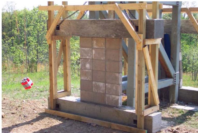
Figure 4.29. Suspension of Charge
