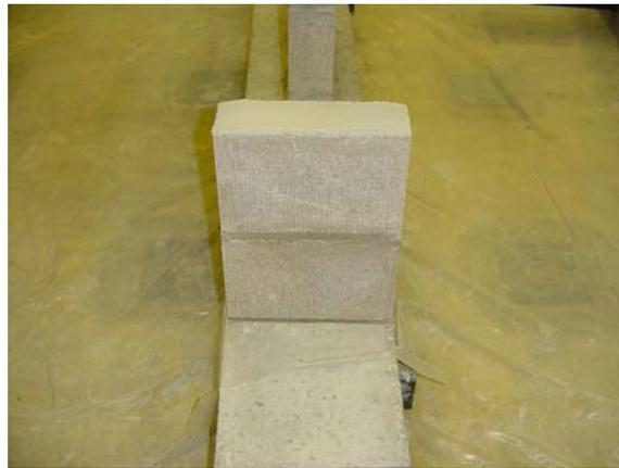
Figure 3.4. Masonry Prism
