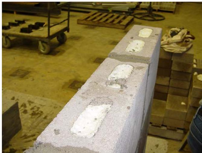
Figure 4.8. Injected Foam
