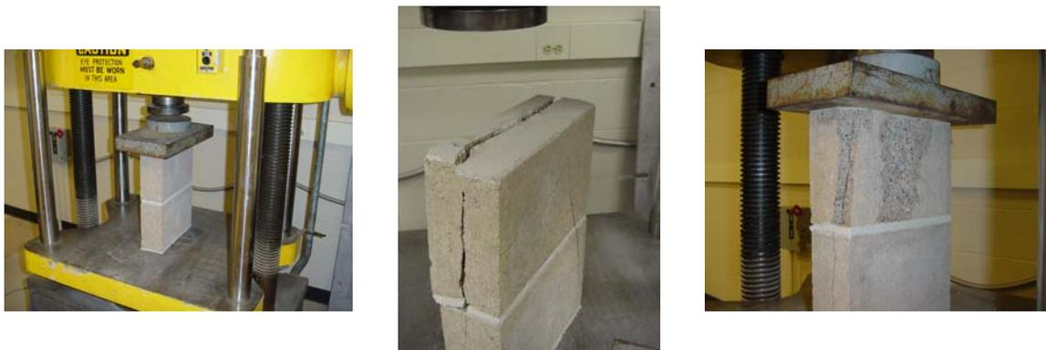
Figure 3.5. Testing of Masonry Prisms
