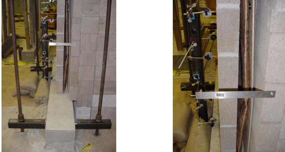
Figure 4.26. Precise Ruler for Deflection Measurement
