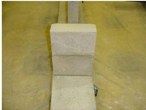
Figure 3.4. Masonry Prism
