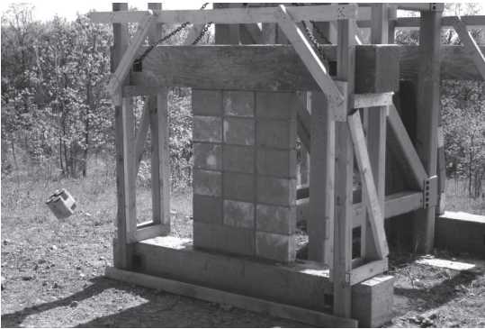
Figure 4 — Phase II Test Set-up with Suspension of Charge (Field)
