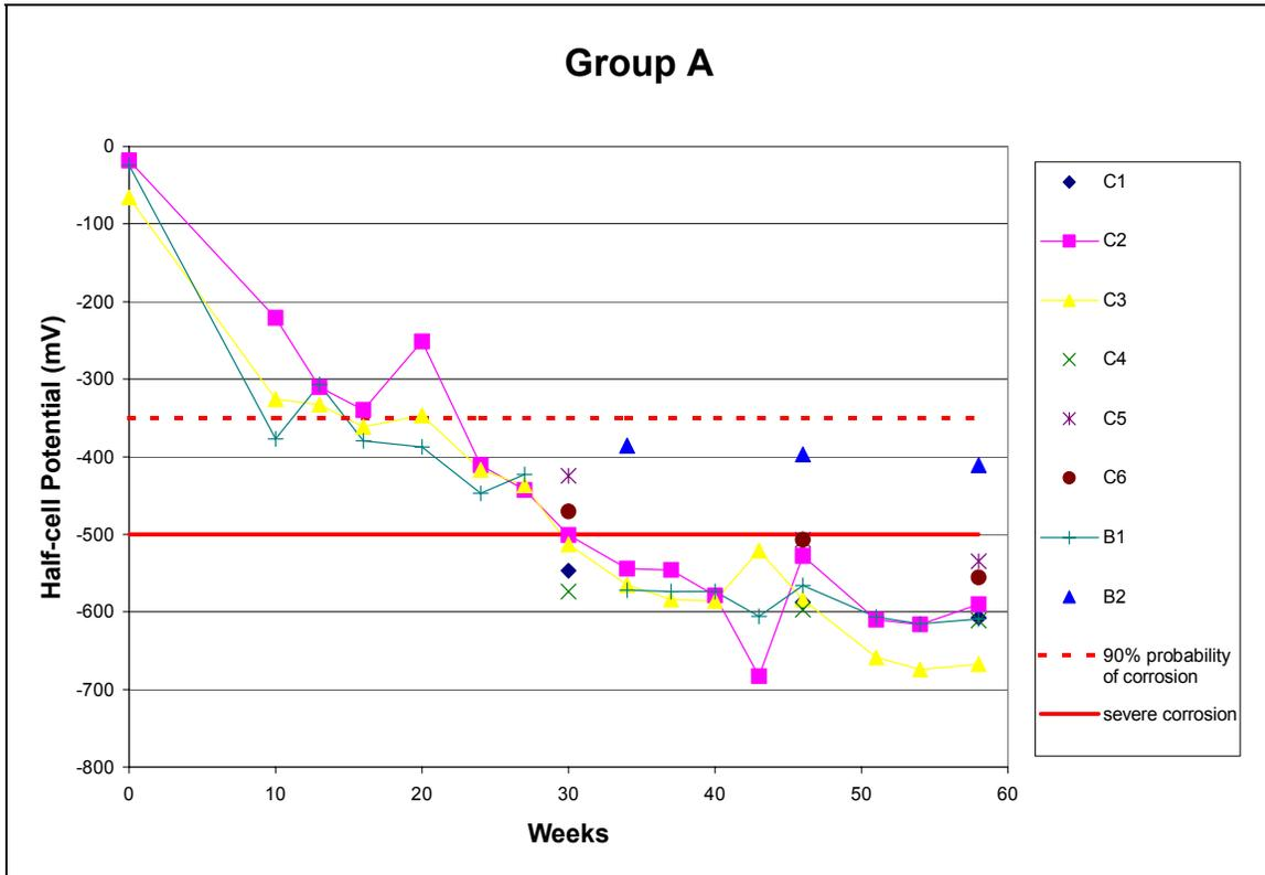
**Figure 1.** Half-cell potential readings for Group A.
