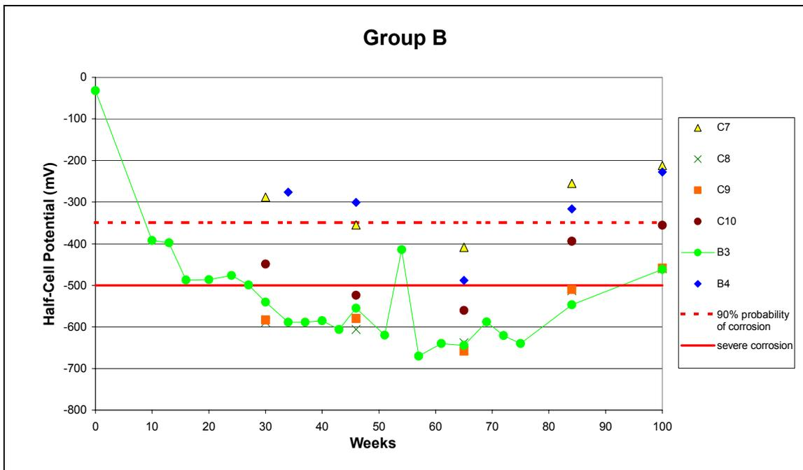
**Figure 2.** Half-cell potential readings for Group B.
