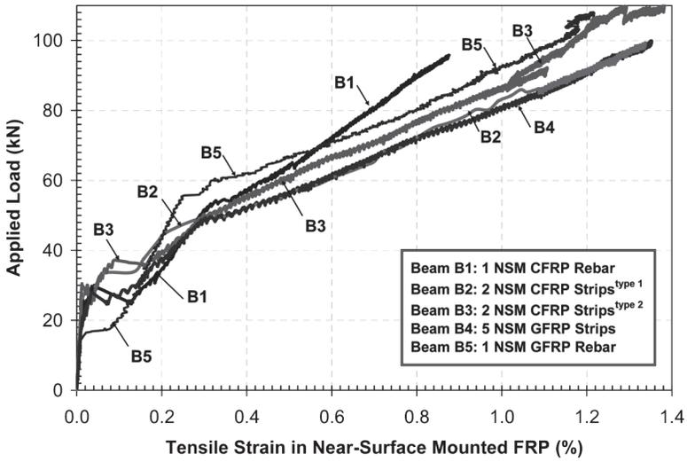
Figure 4 - Load - Tensile Strain in the various NSM FRP Reinforcements at Midspan for the Beams Strengthened with NSM FRP Reinforcements [5,6]
