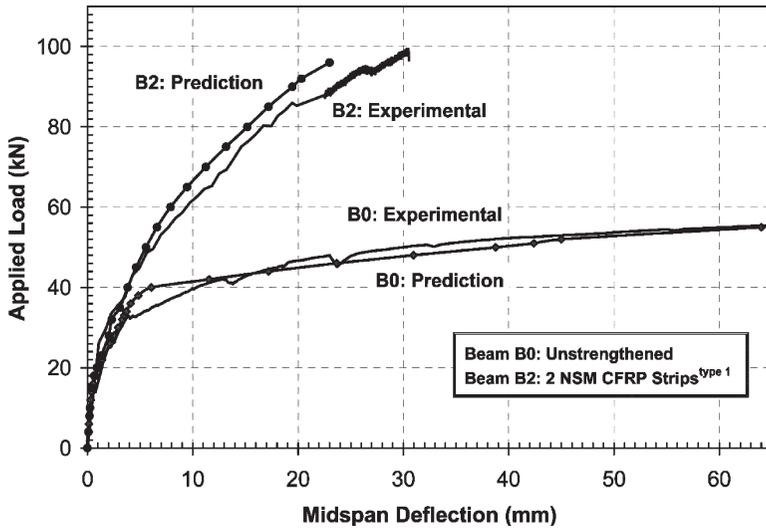
Figure 8 (b) - Load-Midspan Deflection Curves for Beams B0 and B2
