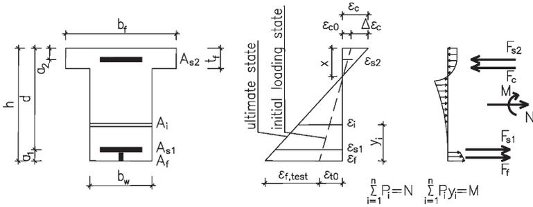
Figure 7 (a) - Calculation Model for a Specimen Strengthened with NSM FRP
