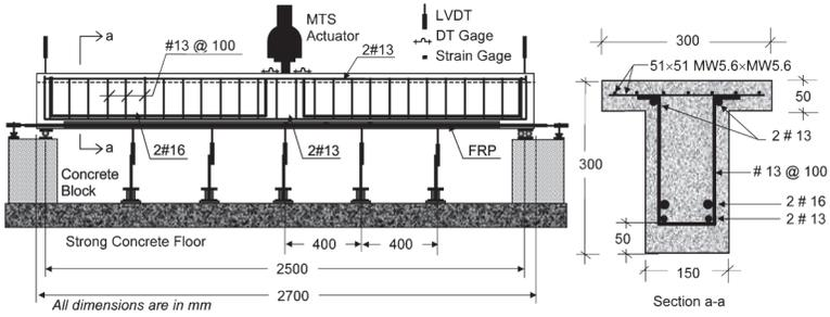
Figure 1 - Beam Details and Test Set-Up [6]
