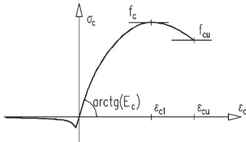
Figure 7 (b) - Stress-Strain Relationship for Concrete
