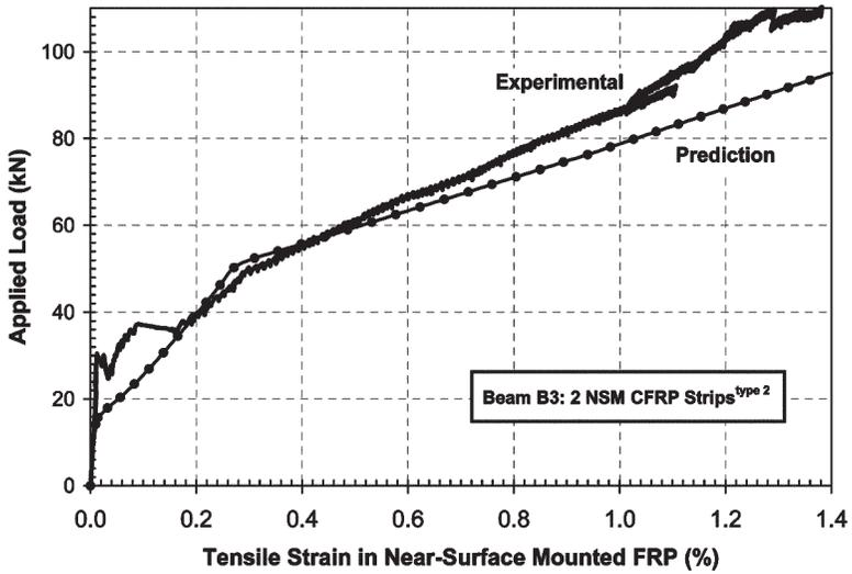
Figure 9 (c) - Load-FRP Tensile Strain Curves for Beam B3
