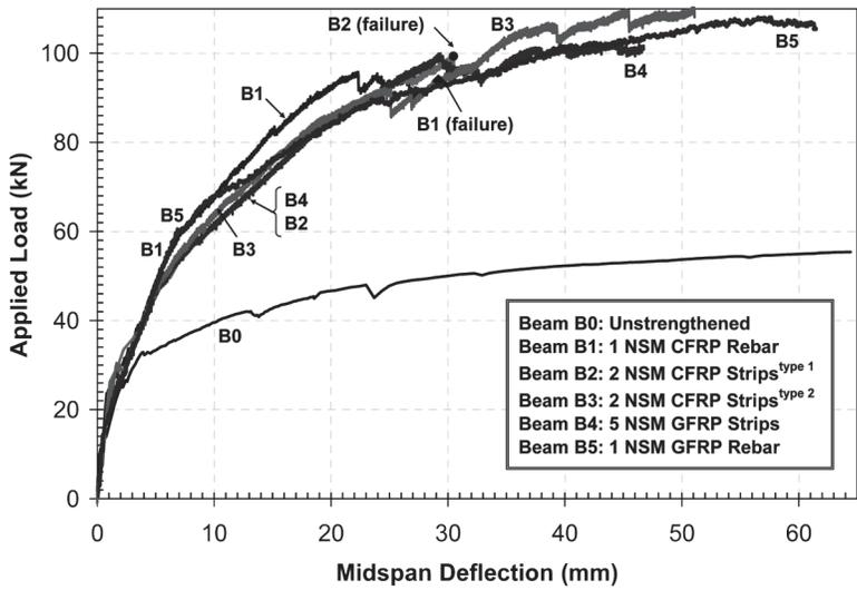
Figure 3 - Load - Midspan Deflection of the Beams Strengthened with various NSM FRP Reinforcements [5,6]
