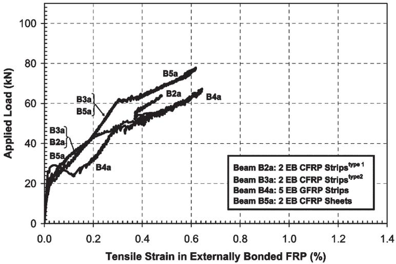
Figure 6 - Load-Tensile Strain in the various EB FRP Reinforcements at Midspan for the Beams Strengthened with EB FRP Reinforcements [5,6]
