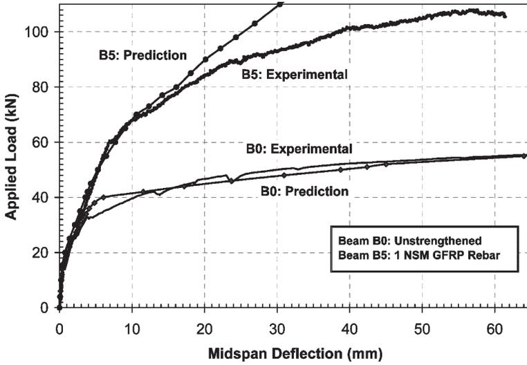
Figure 8 (e) - Load-Midspan Deflection Curves for Beams B0 and B5
