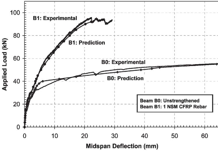
Figure 8 (a) - Load-Midspan Deflection Curves for Beams B0 and B1
