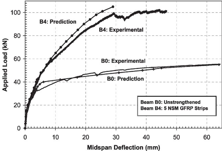
Figure 8 (d) - Load-Midspan Deflection Curves for Beams B0 and B4
