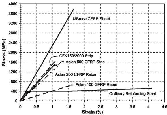
Figure 7 (c) - Stress-Strain Relationships for various FRP reinforcements and Reinforcing Steel
