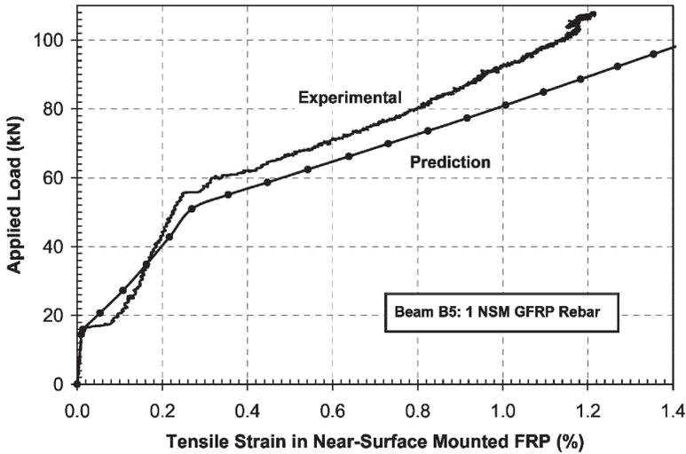
Figure 9 (e) - Load-FRP Tensile Strain Curves for Beam B5
