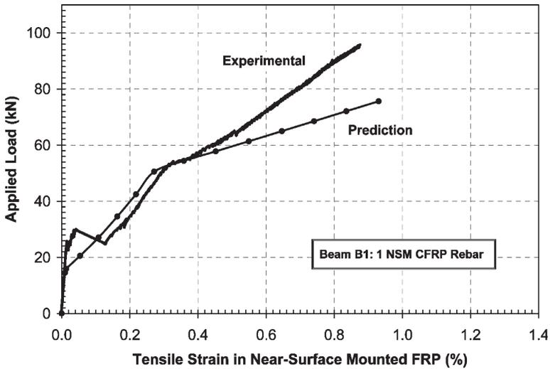
Figure 9 (a) - Load-FRP Tensile Strain Curves for Beam B1
