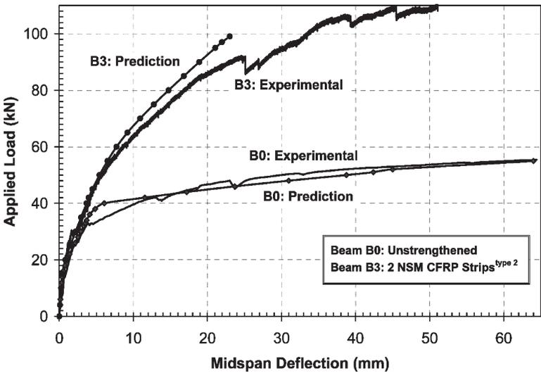
Figure 8 (c) - Load-Midspan Deflection Curves for Beams B0 and B3
