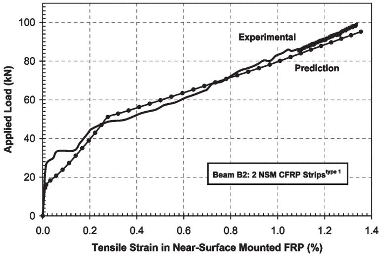
Figure 9 (b) - Load-FRP Tensile Strain Curves for Beam B2
