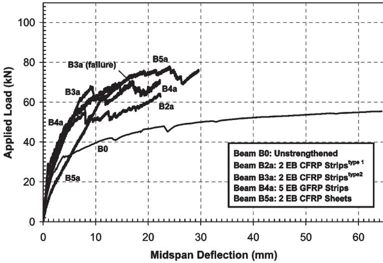
Figure 5 - Load-Midspan Deflection of the Beams Strengthened with various EB FRP Reinforcements [5,6]
