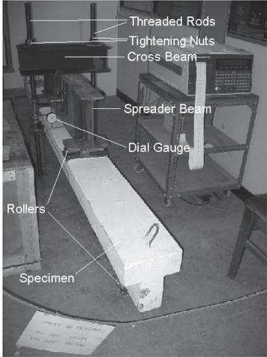
Figure 6 – Long-term beam test set-up
