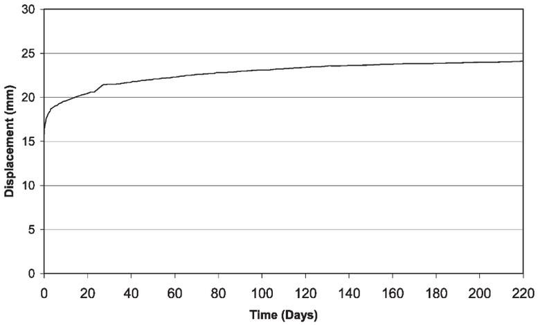
Figure 10 – Long-term midspan deflection vs. time
