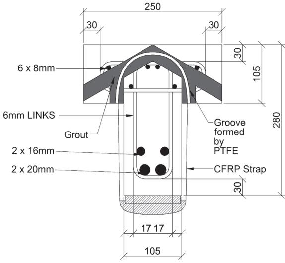
Figure 3 – Beam cross-section
