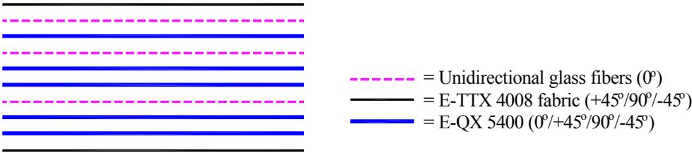
**Figure 2.** Schematic of Ply Lay-Up for Top Plate of 5” Deck. The bottom layer of E-QX 5400 could be replaced by a band of unidirectional glass if more longitudinal stiffness is required.
