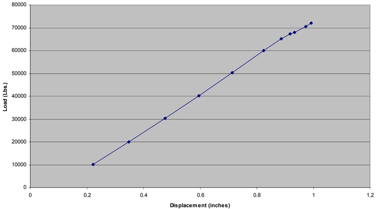
**Figure 9.** Two 5” Deck Specimens Bonded Together. July 2001 test at CFL (NCSU).
