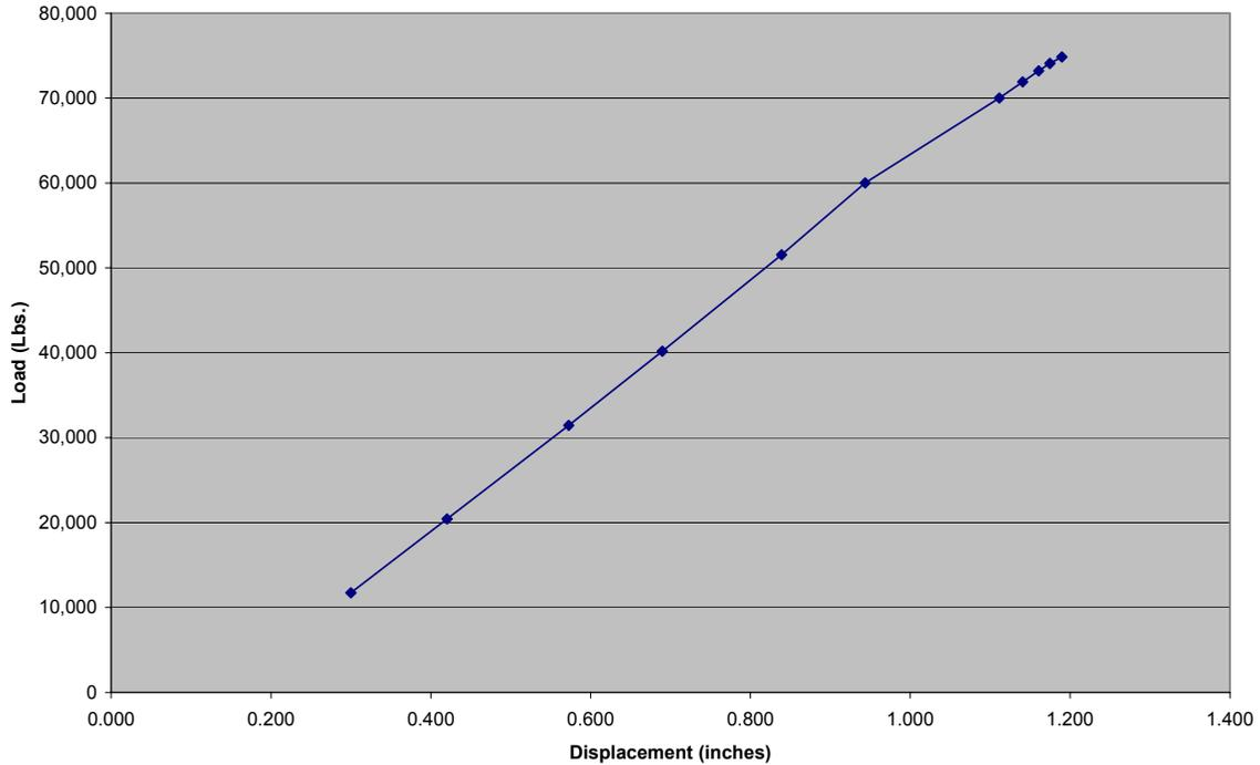
**Figure 8.** Plot of Load Versus Displacement for the 5” Deck Specimen. Single tube only.
