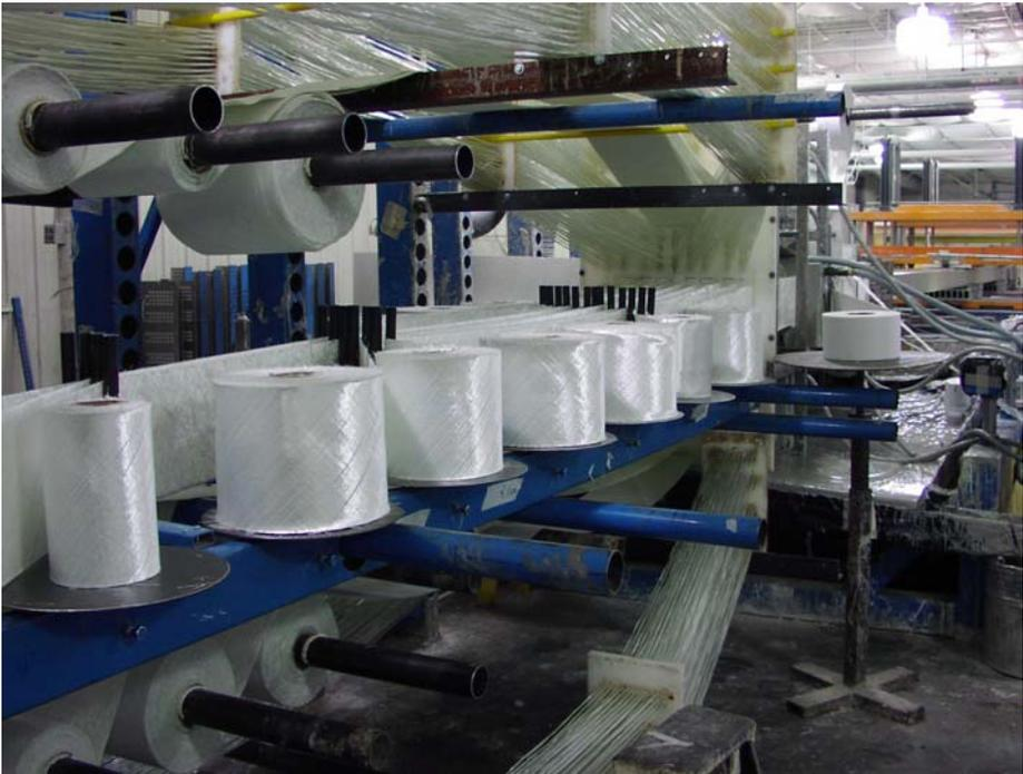
**Figure 4.** Fabrics and Unidirectional Fibers Being Pulled Into the Mold.
