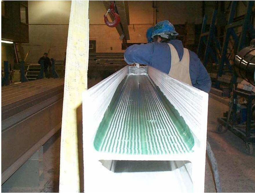
**Figure 10.** Adhesive Being Applied to the Female Part of the Bond Line Joint in the 5” Deck.
