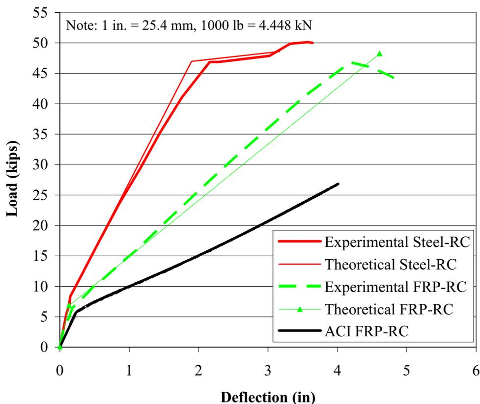
**Figure 6.8 Experimental and Theoretical Load-Deflection Relationships for the Steel-RC and FRP-RC Panels**
