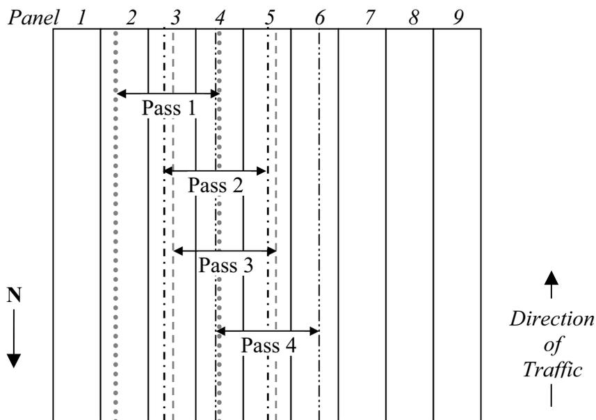
**Figure 7.36 Lateral Location of Truck Passes 1 through 4**
