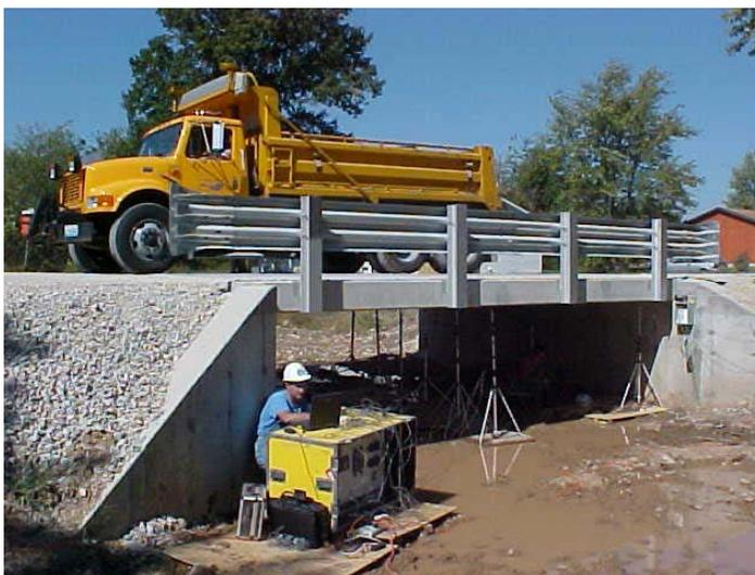
**Figure 7.37 In-situ Bridge Load Test – Walters Street**
