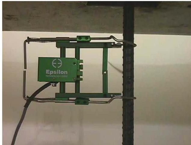
**Figure 6.1 Extensometer Utilized During Tensile Testing**
