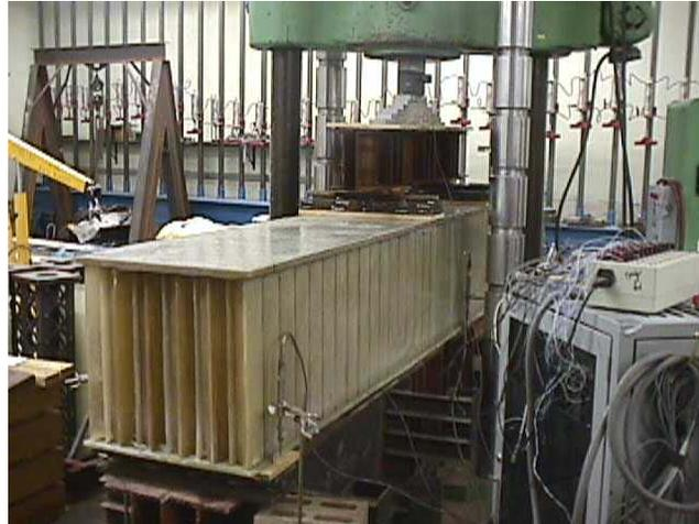
**Figure 5.3 Flexural Test Setup – SF-2-1 and SF-2-2**
