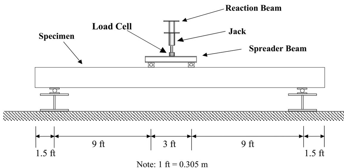
**Figure 6.5 Test Schematic for the RC Specimens**
