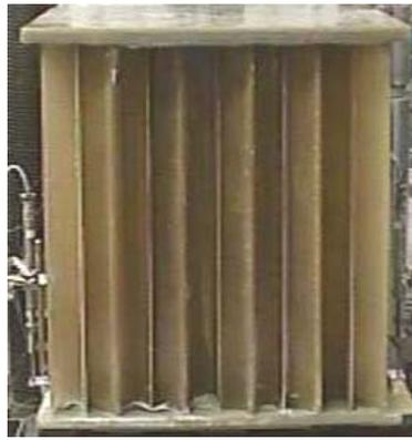
**Figure 3.2 FRP Sandwich Panel Structure**
