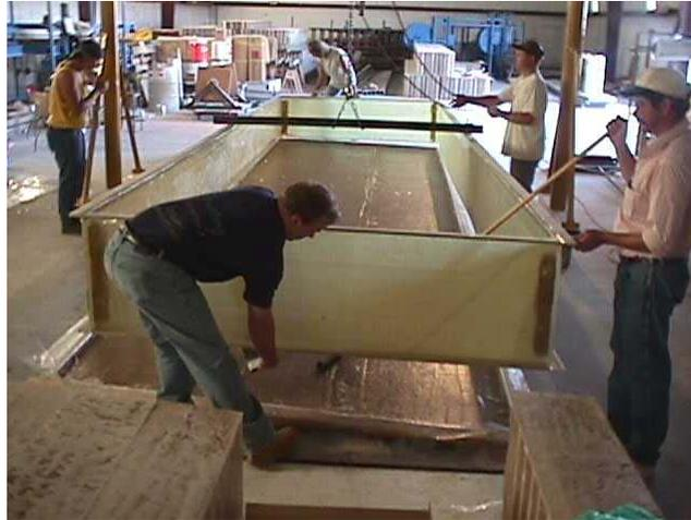
**Figure A.3 Installation of the Panel Edges**
