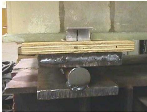
**Figure 5.2 Specimen Support Detail**
