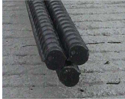
(b) Bundled CFRP Bars
