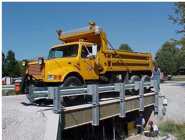
**Figure 7.27 In-situ Bridge Load Test – St. Francis Street**
