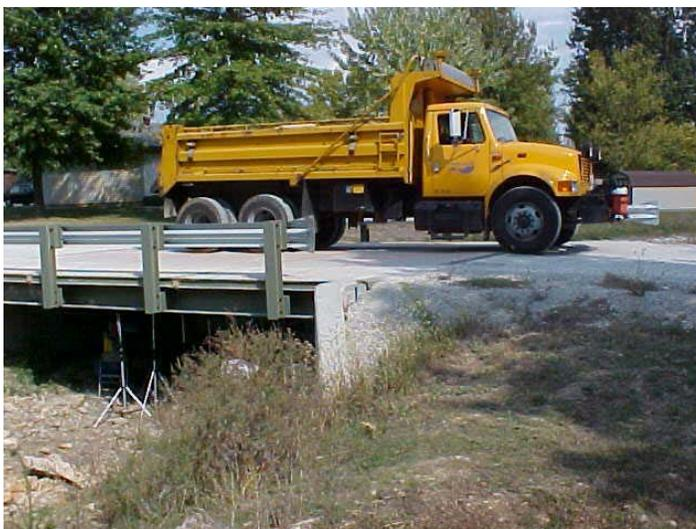
**Figure 7.3 In-situ Bridge Load Test – St. Johns Street**
