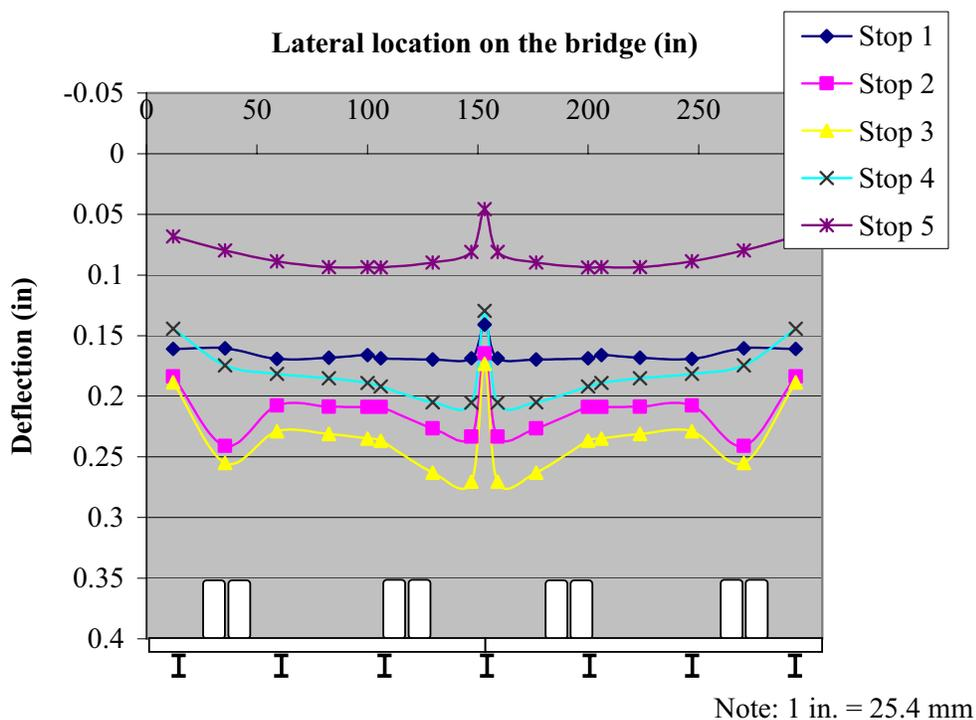
**Figure 7.12 Deflected Shape – Superposition of Pass 1 – St. Johns Street**
