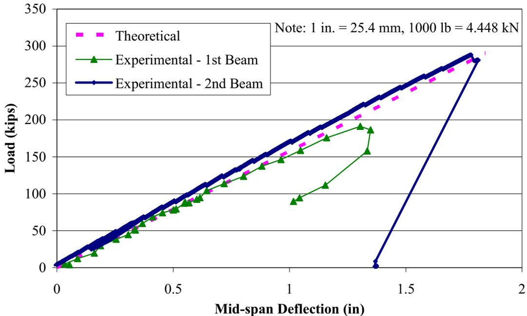
**Figure 5.5 Load vs. Deflection Results – SF-2-1 and SF-2-2**
