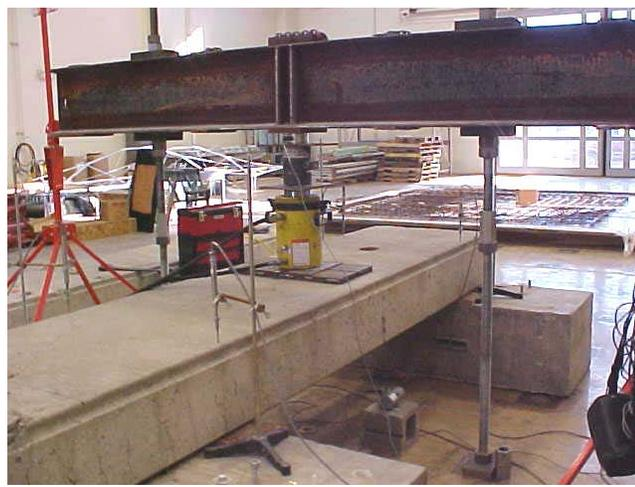
**Figure 6.14 Test Setup for Shear Testing**
