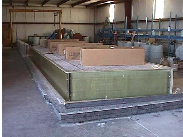
**Figure A.5 Weighting of the Core Sections**
