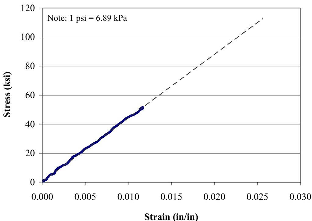
**Figure 6.2 FRP Bar – Typical Tensile Test Result**
