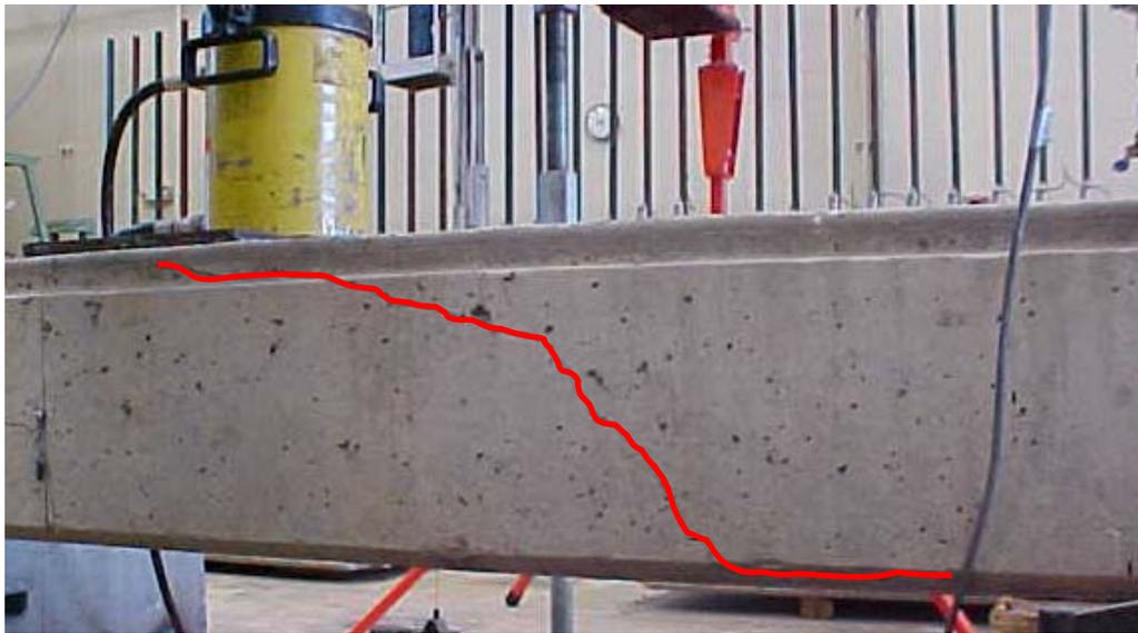
**Figure 6.16 Shear Failure of the Steel-RC Panel**
