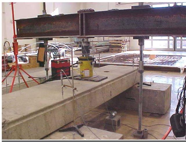
**Figure 6.14 Test Setup for Shear Testing**
