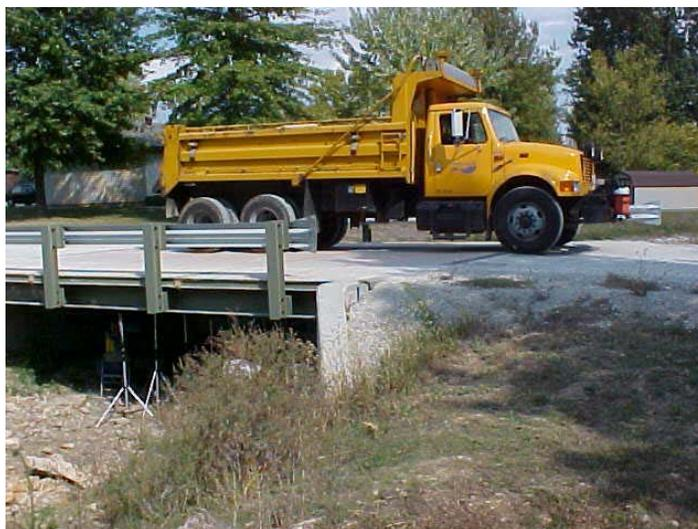
**Figure 7.3 In-situ Bridge Load Test – St. Johns Street**
