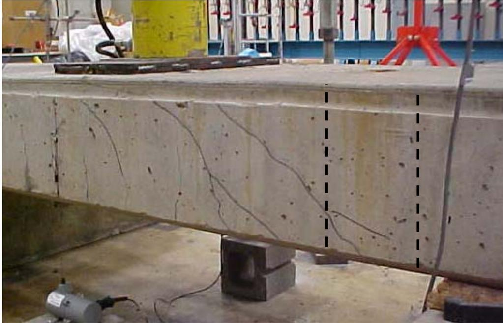
**Figure 6.17 Shear Failure of the FRP-RC Panel**
