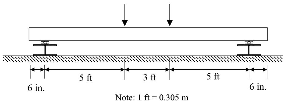
**Figure 5.1 Flexural Test Schematic - SF-2-1 and SF-2-2**
