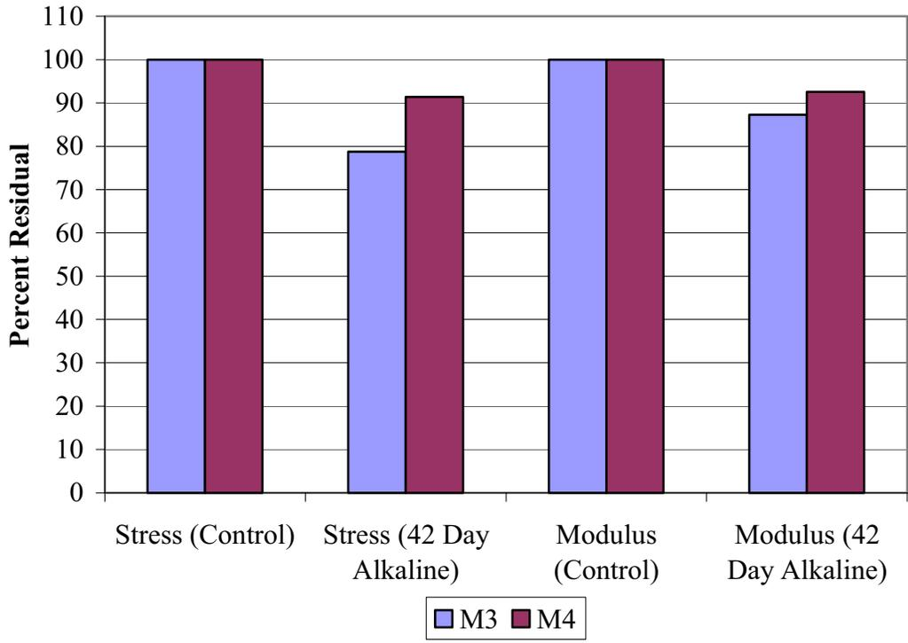
**Figure 6.19 Residual Tensile Properties for GFRP Bars**
