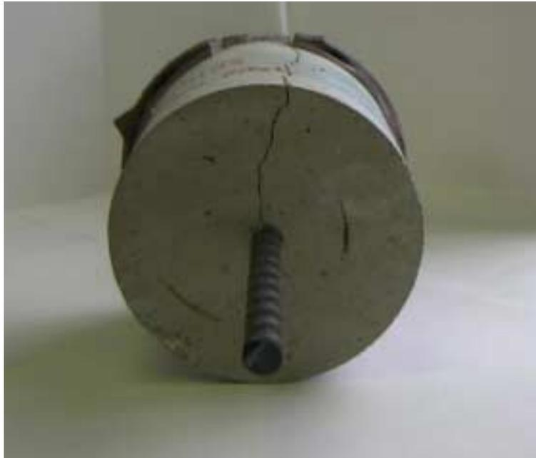
**Figure 3.** Concrete splitting failure.
