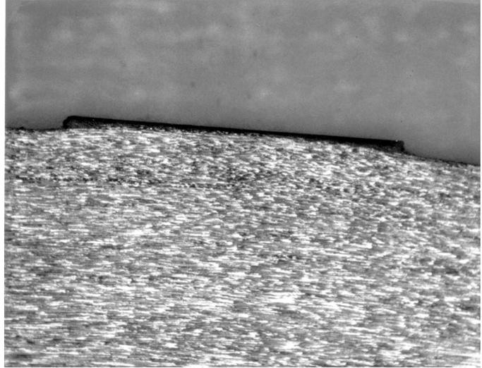
**Figure 7.** Micrograph showing resin rich region between spiral indentations.
