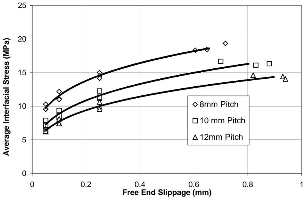
Figure 6. Average interfacial stress vs. free end slippage.
