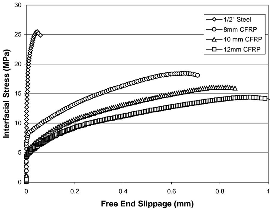
Figure 5. Interfacial stress vs. free end slippage.
