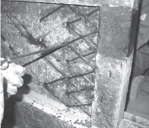
Fig.6—A zigzag sewing path
