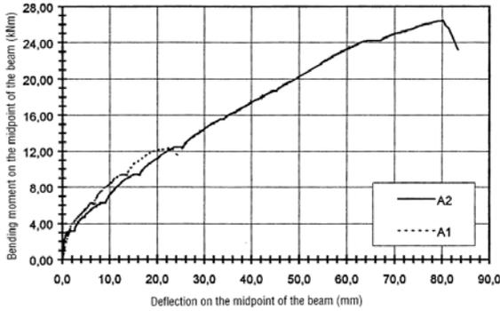
• The load-deflection curves of test beams A1 and A2
