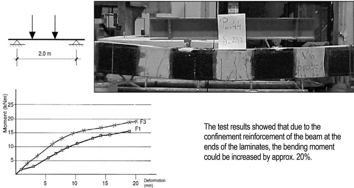
The test results showed that due to the confinement reinforcement of the beam at the ends of the laminates, the bending moment could be increased by approx. 20%.
