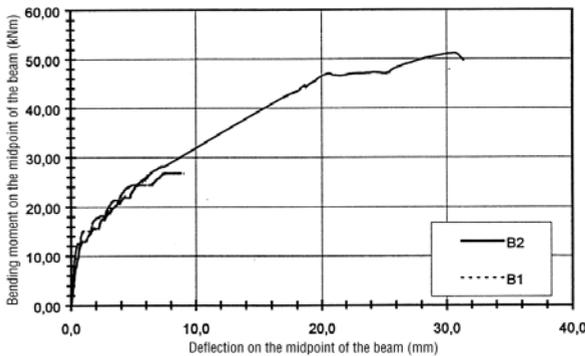
• The load-deflection curves of test beams B1 and B2
