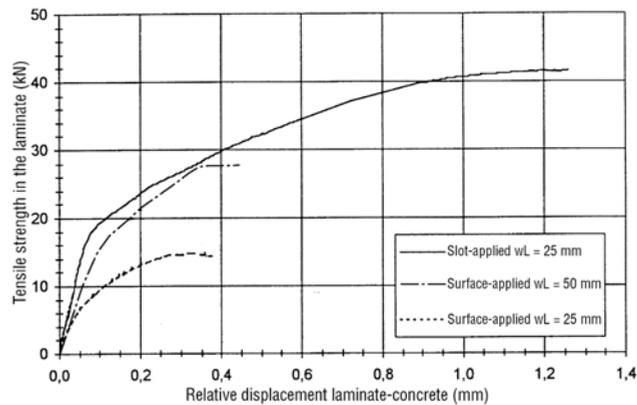
The illustration above shows the relative displacement in the static tensile strength test. It clearly shows the considerably more ductile behavior of the slot-applied CFRP laminate.
