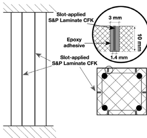
Column with slot-applied laminates
