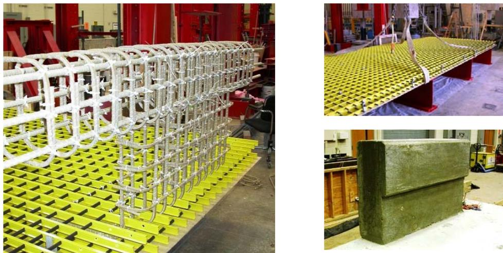
Figure 1 - Strategy for pultruded GFRP internal reinforcement system for concrete deck and railings: 3-D stay-in-place gratings (deck) and GFRP reinforcing bars (rail)
