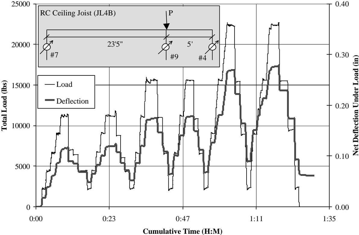
**Figure A.23: Time history of rapid load test for JL4B**
