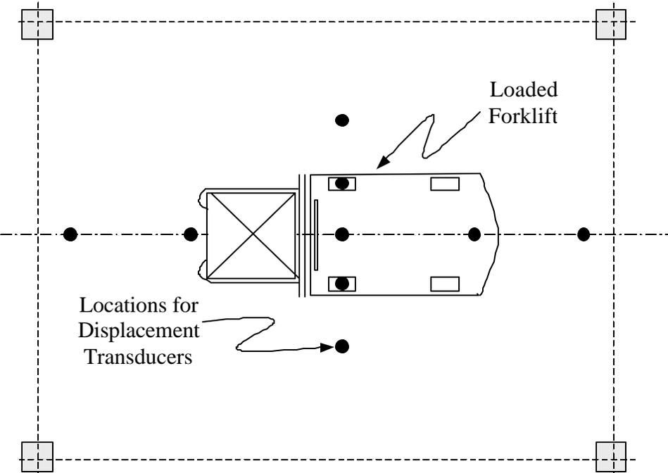
Figure 2.11: Plan view of vehicle loaded test method
