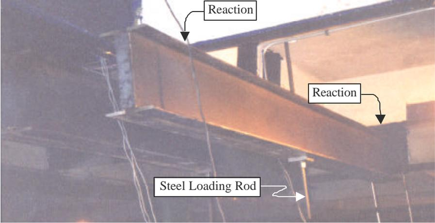
**Figure B.11: Loading apparatus used for Load Configuration 1**
