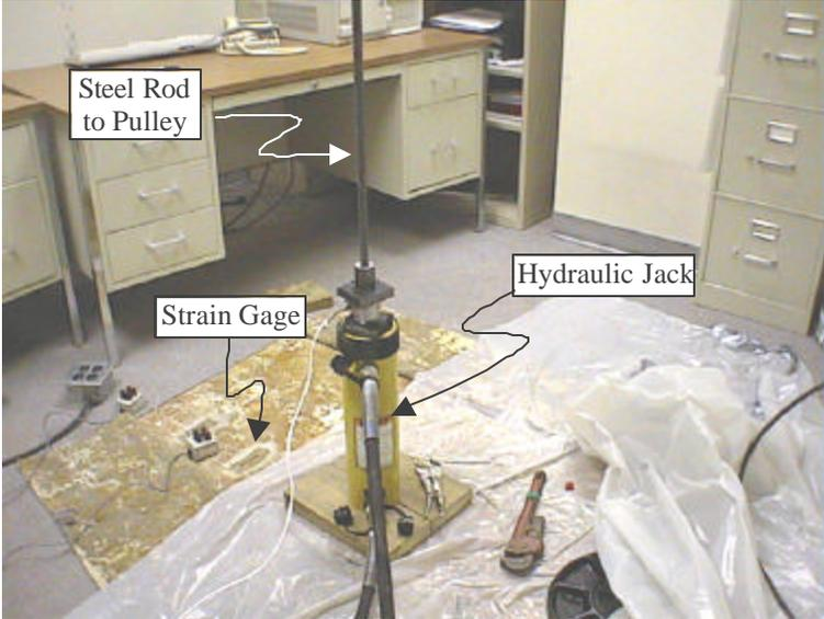
**Figure B.6: Hydraulic jack used to apply load**
