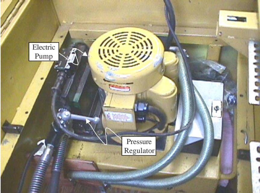
**Figure 2.16: Electrical pump used to supply fluid to hydraulic jacks**
