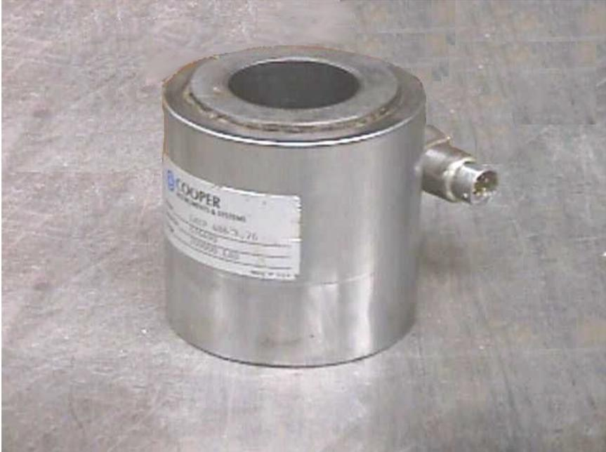
**Figure 2.24: Load cells used to measure applied load**
