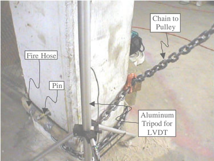
**Figure B.8: Detail showing reaction provided by the column**
