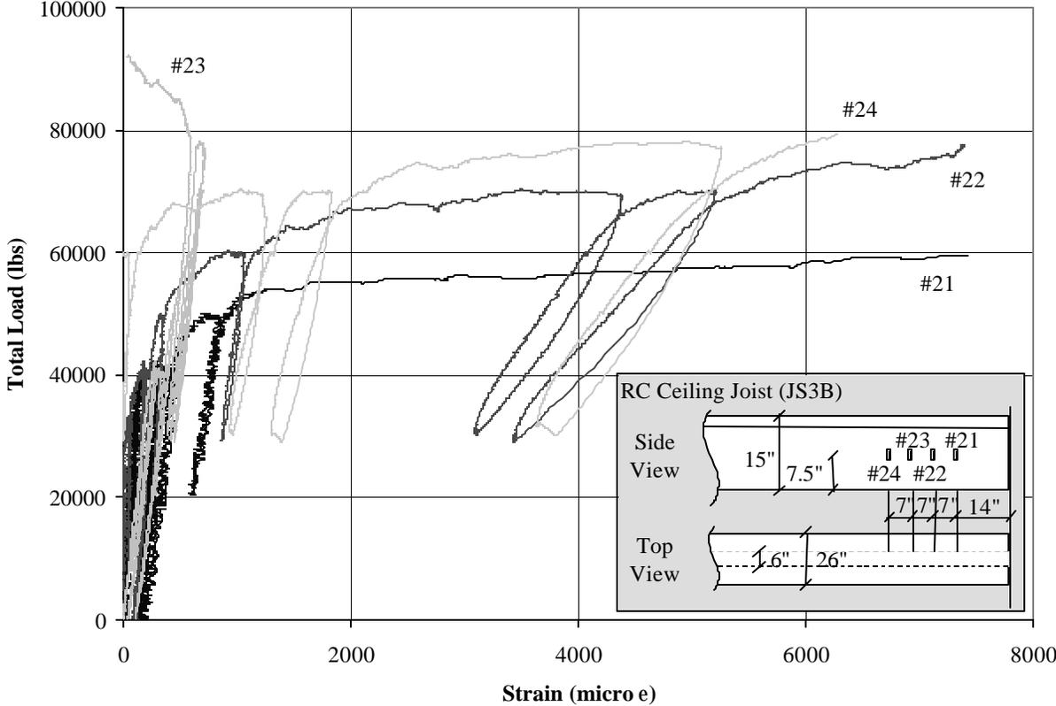
**Figure A.15: Load versus strain for JS3B**
