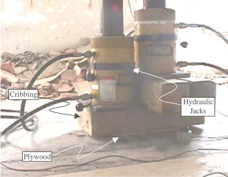
**Figure A.8: Typical load setup on top of test member**
