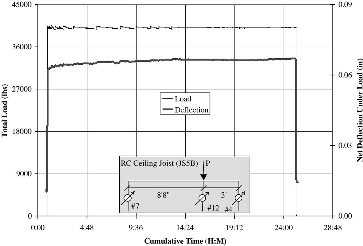
**Figure A.18: Time history of 24-hour load test for JS5B**
