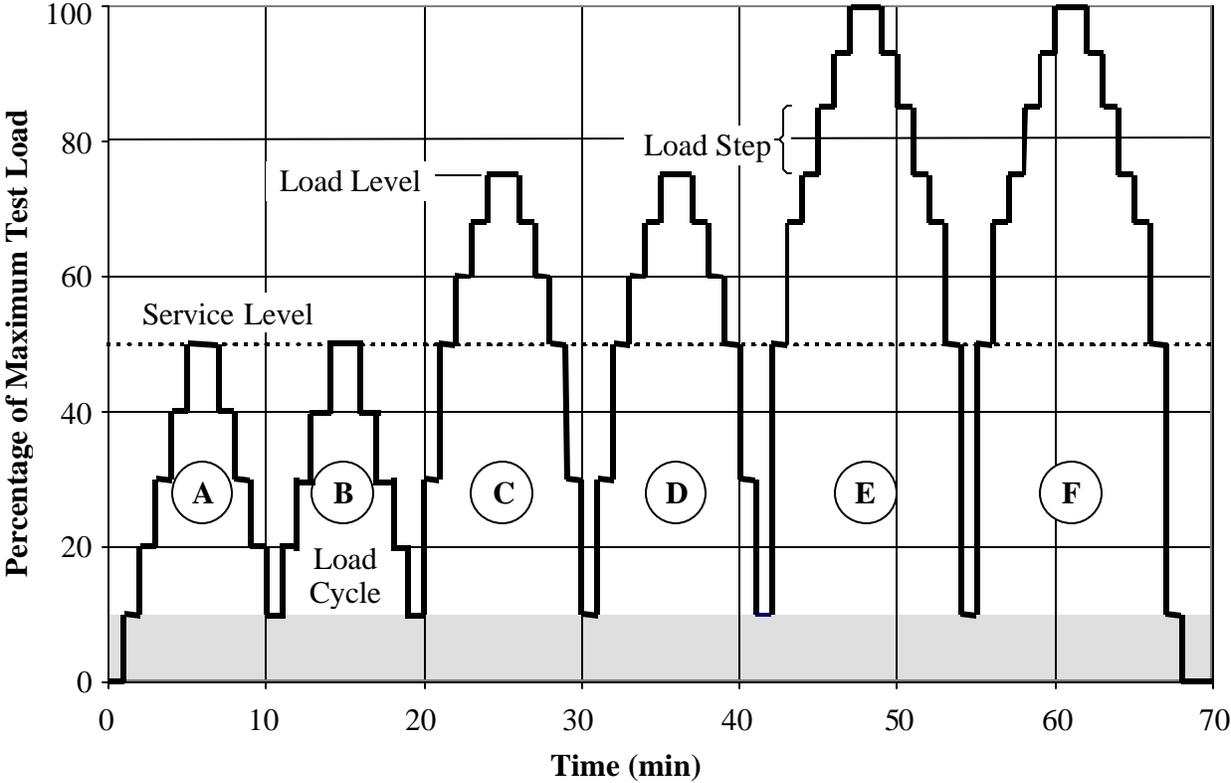
Figure 3.1: Load steps and cycles for a rapid load test
