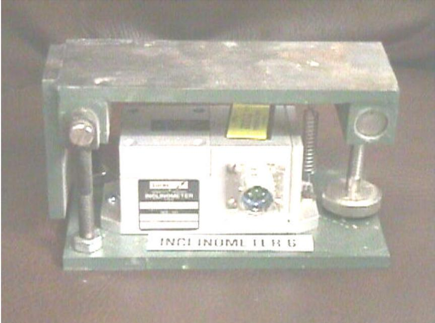
**Figure 2.20: Inclinometers used to measure slope**
