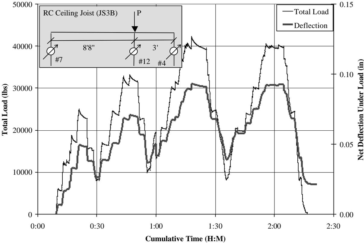
Figure A.11: Time history of rapid load test for JS3B
