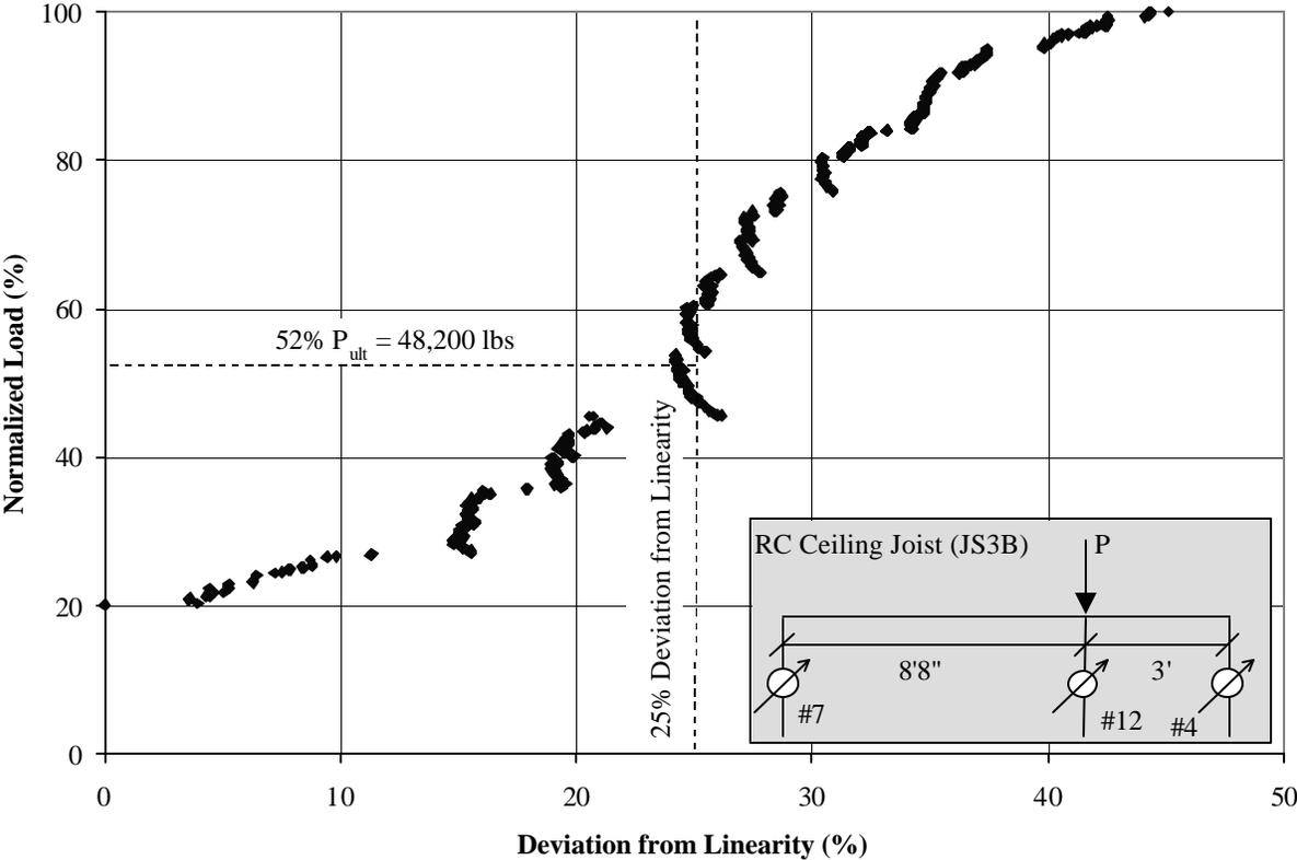
**Figure A.14: Normalized load versus deviation from linearity for JS3B**
