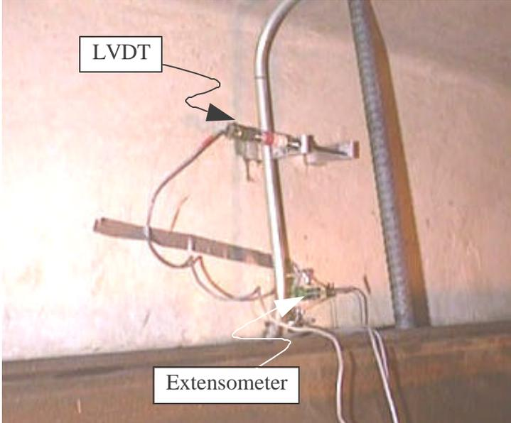
Figure B.12: LVDT and extensometer measuring elongation
