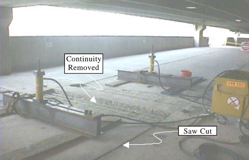
**Figure 2.14: Removing continuity allows for true simply supported condition**
