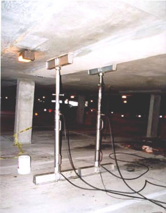
**Figure B.1: Load applied by hydraulic jacks**
