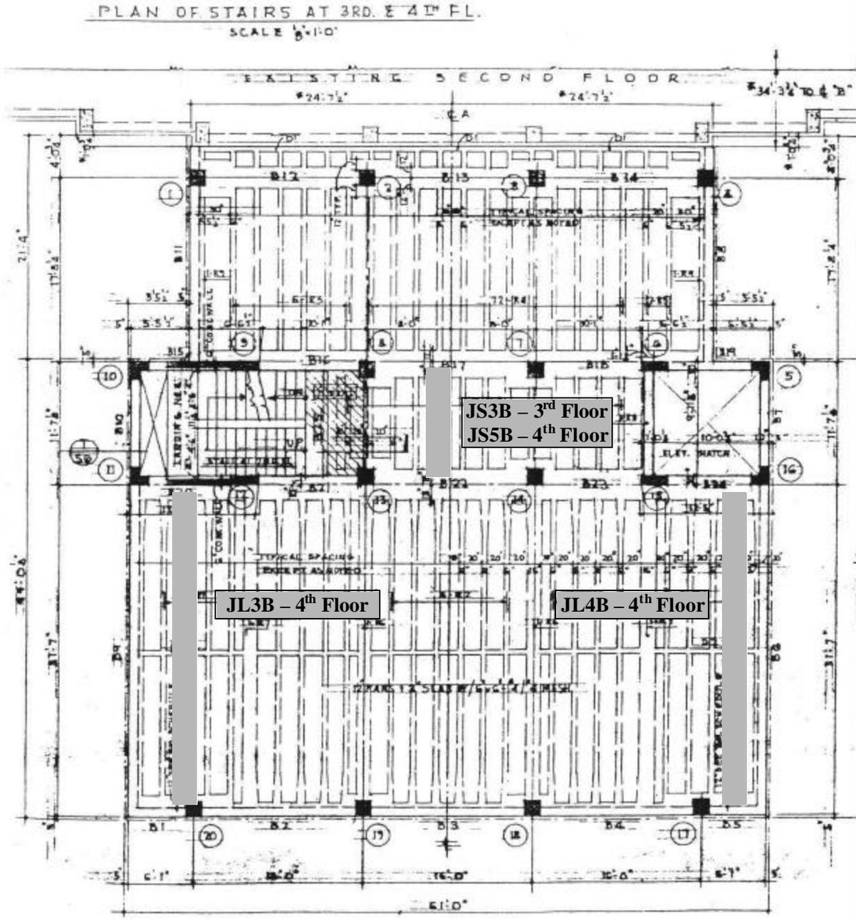
Figure A.7: Plan view shows locations of tested members
