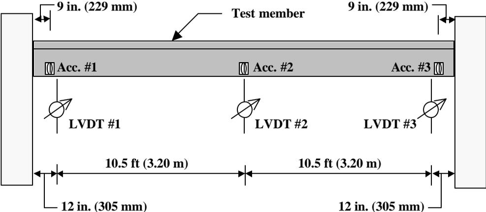
Figure B.22: Schematic drawing shows location of LVDTs and accelerometers
