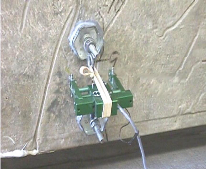
Figure 2.22: Extensometers used to measure the strain across a crack and crack widths
