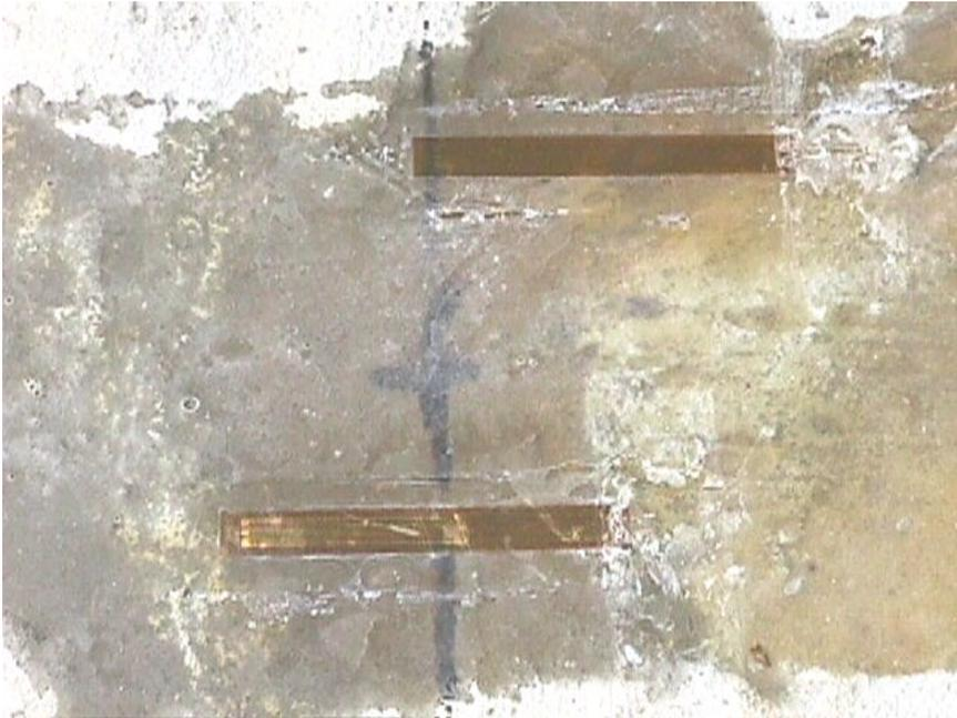
**Figure 2.21: Strain gages used to measure the compression strain in concrete**
