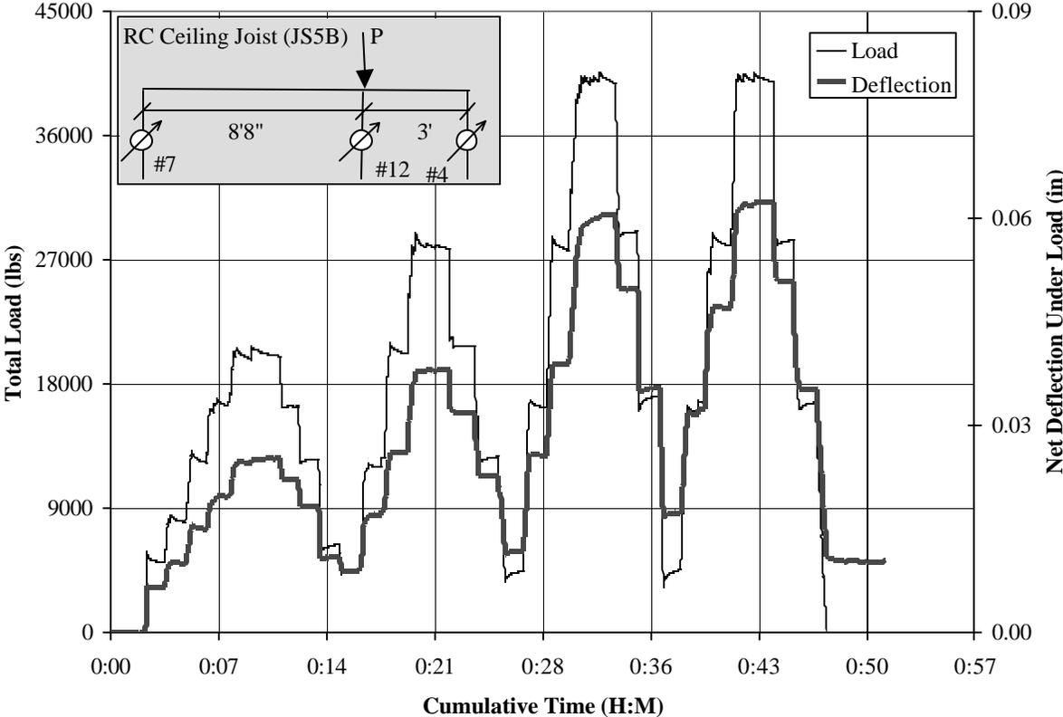
**Figure A.17: Time history of rapid load test for JS5B**
