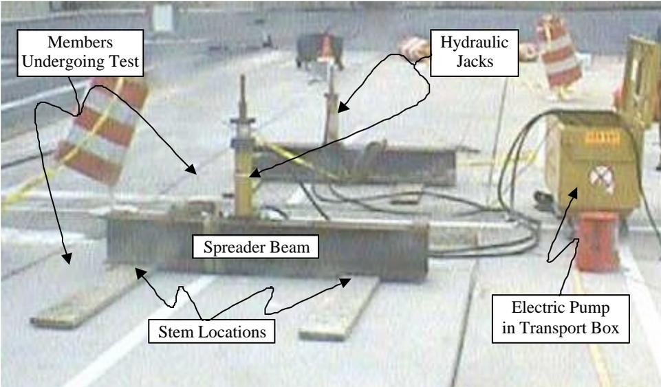
Figure B.17: Closed loop method from above the test members
