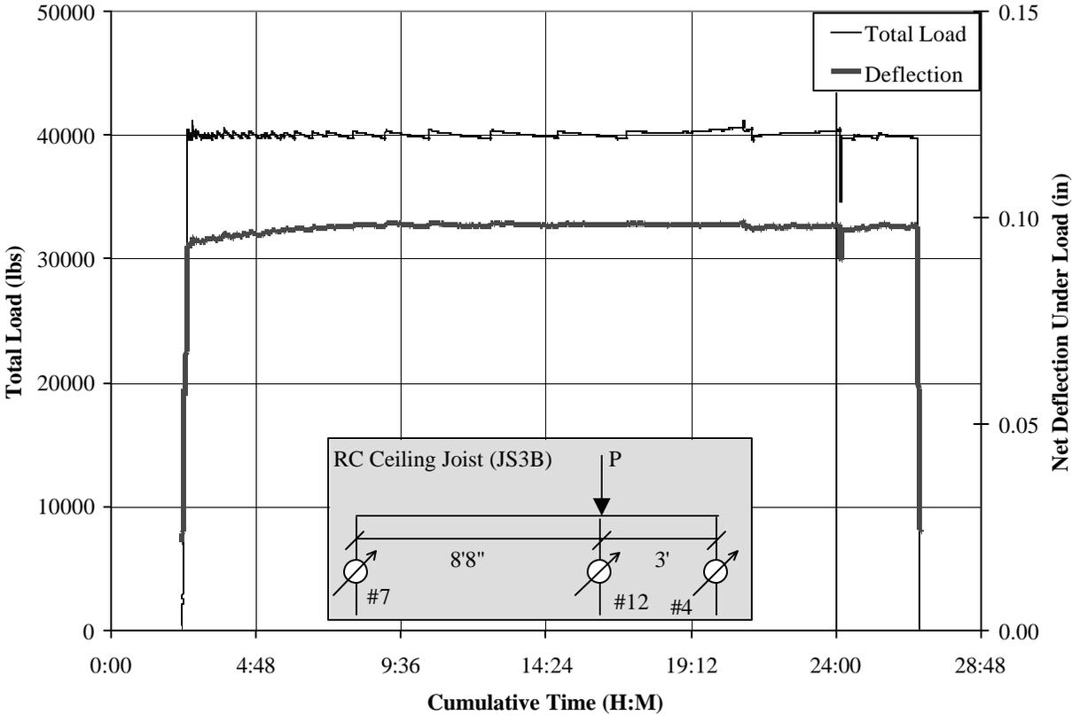
**Figure A.12: Time history of 24-hour load test for JS3B**
