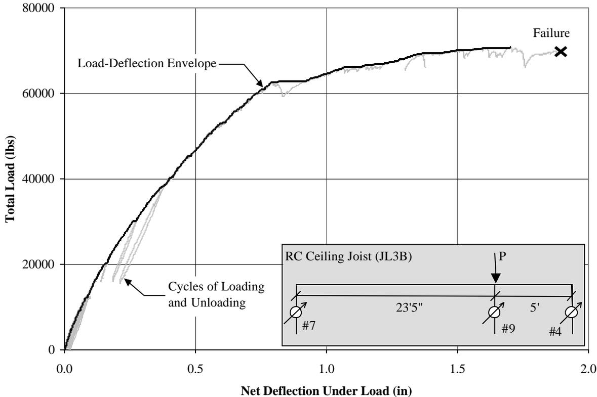
**Figure A.22: Load versus deflection curve for JL3B**
