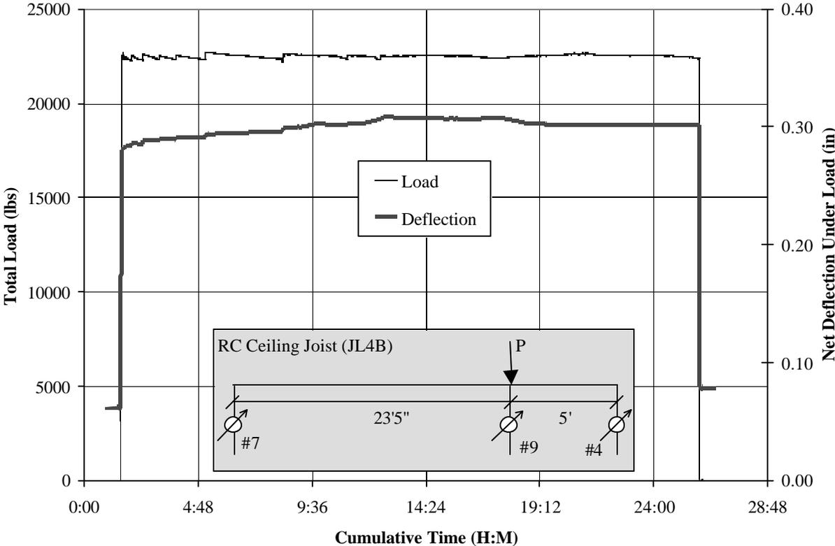
**Figure A.24: Time history of 24-hour load test for JL4B**
