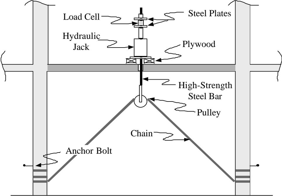
Figure 2.4: Detail of pull-down test method with a fixed reaction
