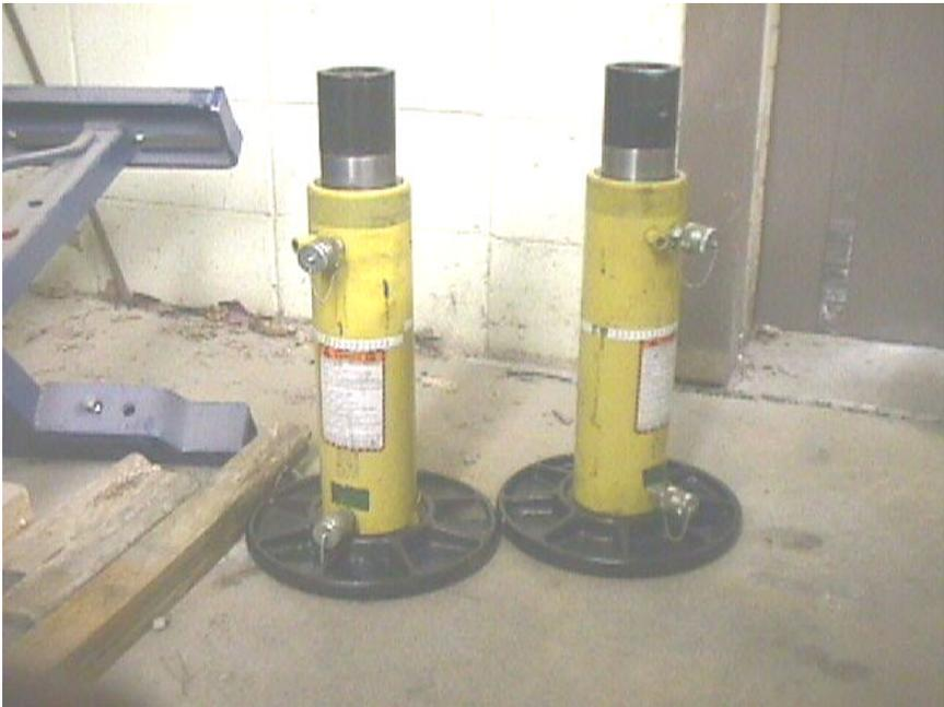
**Figure 2.15: Hydraulic jacks used to apply load**
