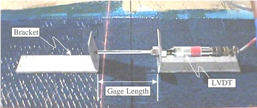
Figure 2.23: LVDT used to measure the average strain over a gage length
