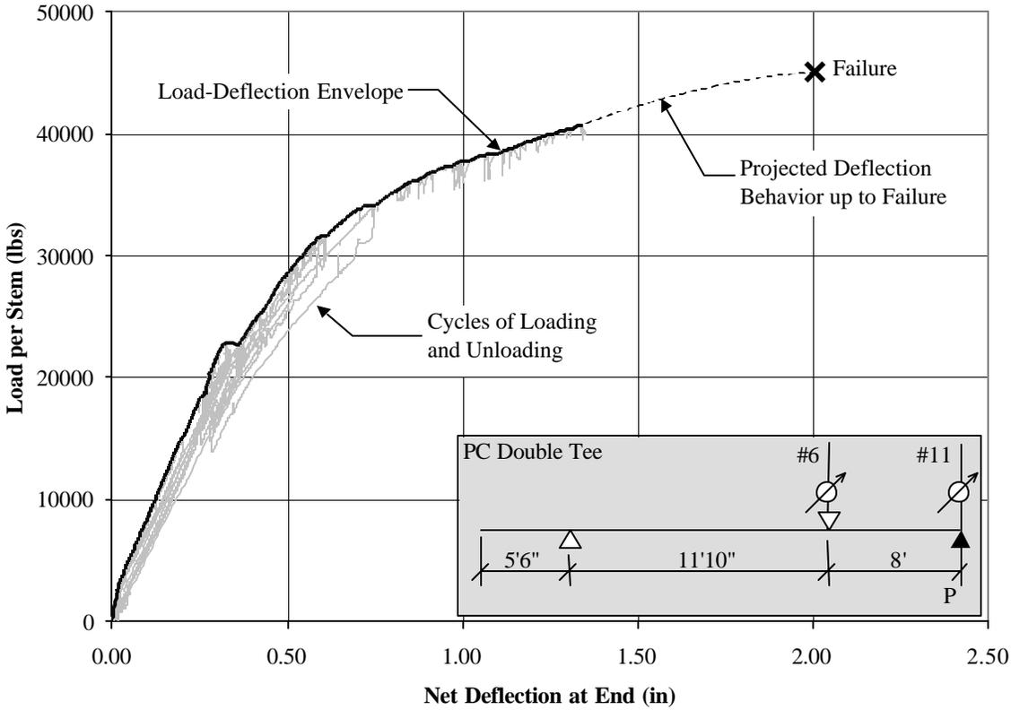
**Figure A.5: Load versus deflection curve for PC double tee**
