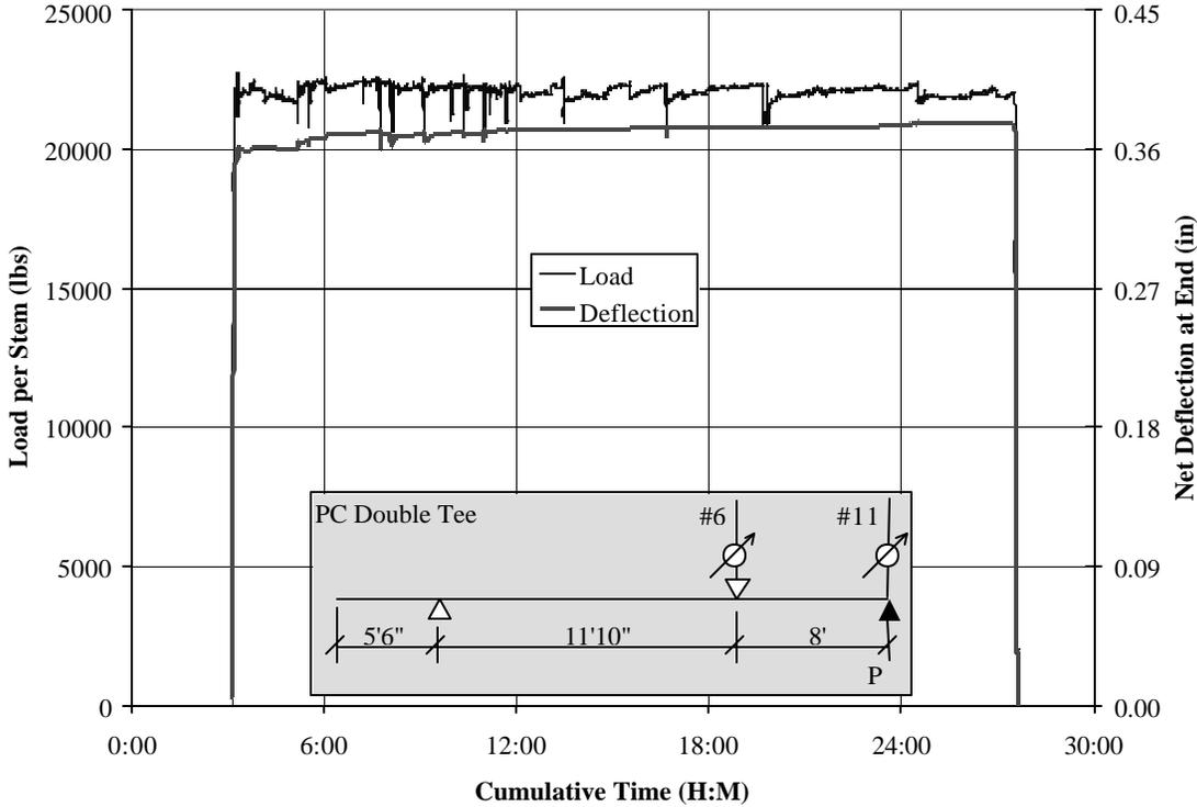
**Figure A.4: Time history of 24-hour test of PC double tee**
