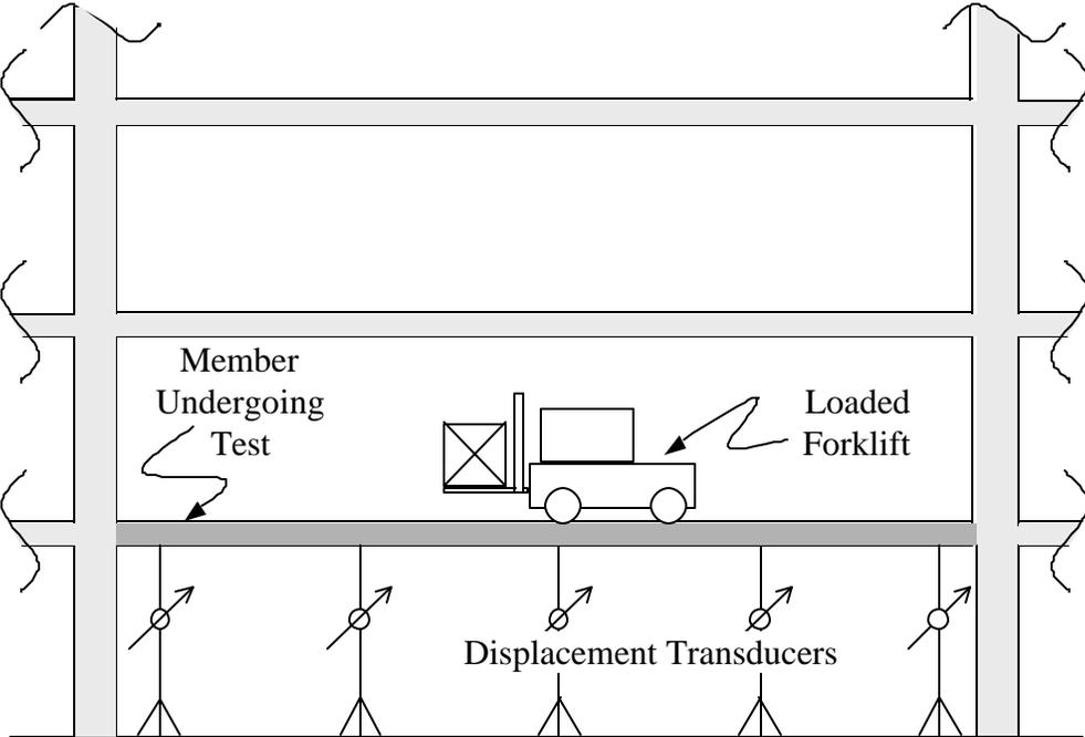
Figure 2.10: Vehicle loaded test configuration
