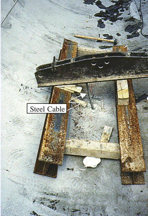
**Figure B.9: Spreader beam used to apply the load**
