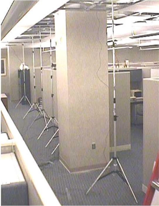
**Figure B.5: LVDTs mounted on aluminum tripods**
