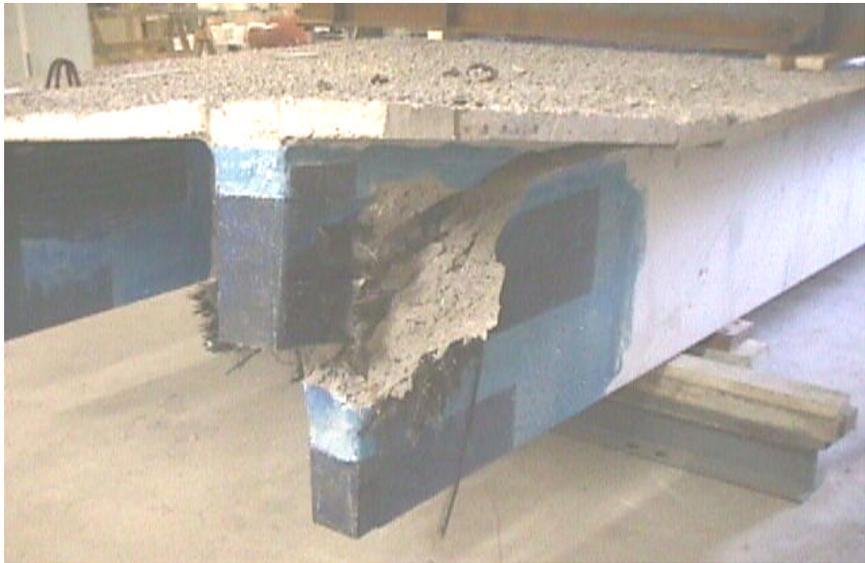
**Figure A.6: Shear failure in the dap end of the externally strengthened PC double tee**
