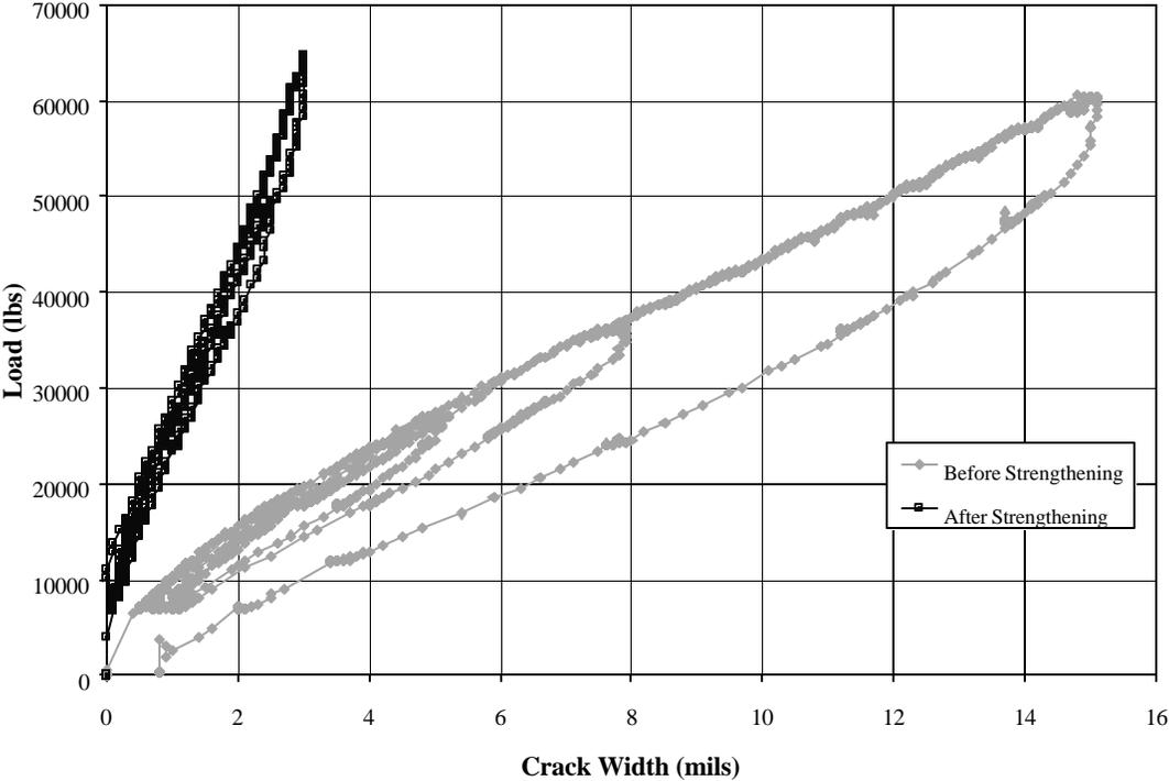
Figure B.14: Load versus crack width at joist mid-span before and after strengthening [Load Test A-1 and B-1] (1 mils = 0.001 in. = 0.0254 mm, 1 lbs. = 4.45 N)
