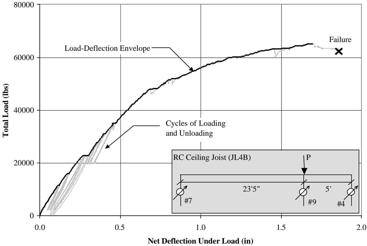
**Figure A.25: Load versus deflection curve for JL4B**
