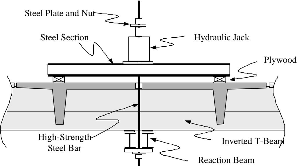
**Figure 2.9: The closed loop method can be used to apply loads to both stems of a double tee**
