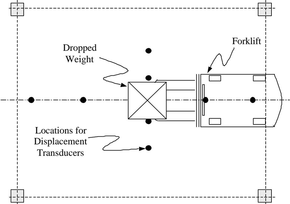
Figure 2.13: Plan view of dropped weight test method
