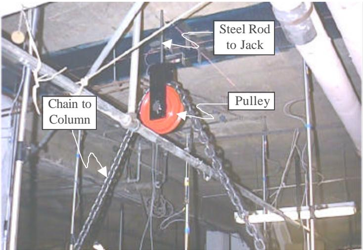
**Figure B.7: Apparatus for providing reaction for hydraulic jacks**
