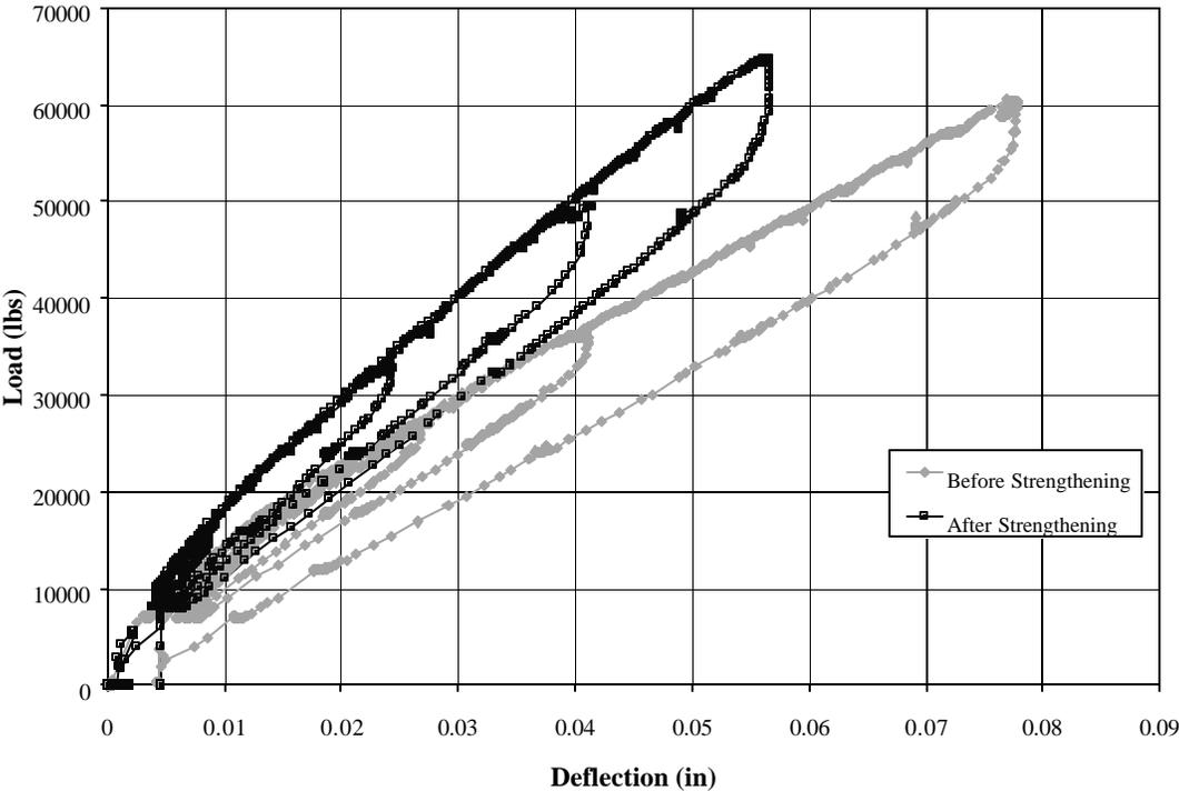
Figure B.13: Load versus deflection of joist mid-span before and after strengthening [Load Test A-1 and B-1] (1 in. = 25.4 mm, 1 lbs. = 4.45 N)
