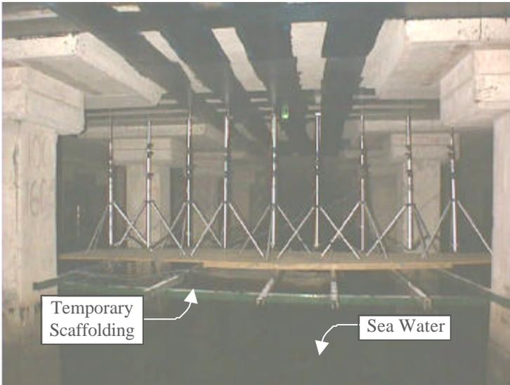
**Figure B.21: LVDTs mounted on tripods sitting on temporary scaffolding below pier**
