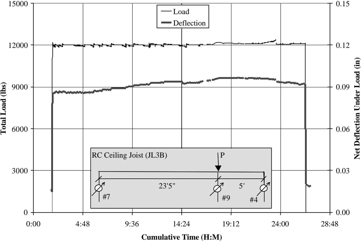
**Figure A.21: Time history of 24-hour load test for JL3B**
