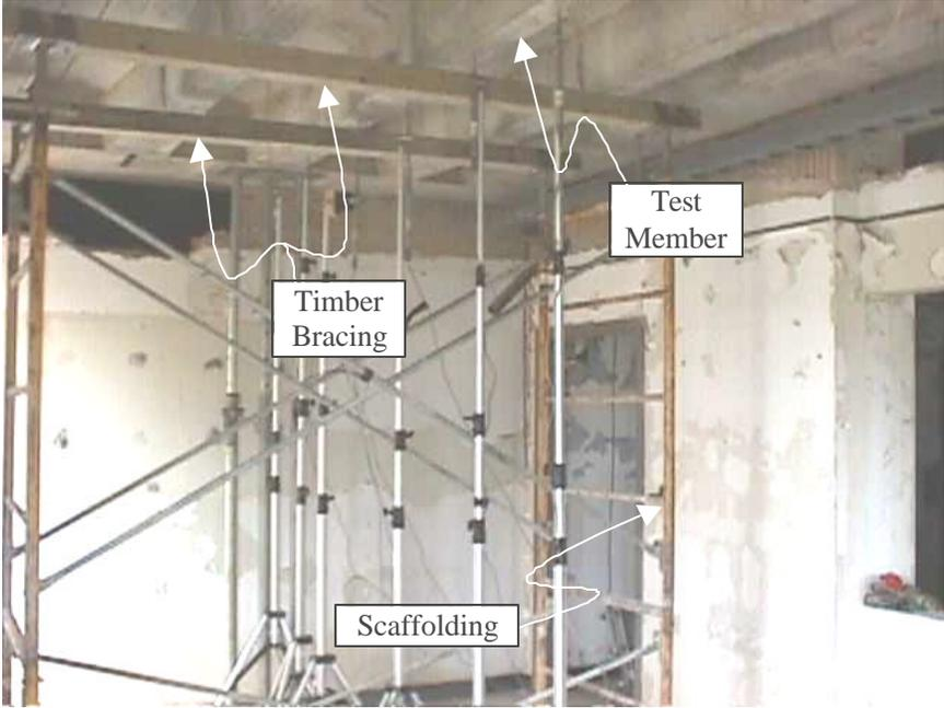
**Figure 2.26: Scaffolding used to prevent total collapse of tested member**
