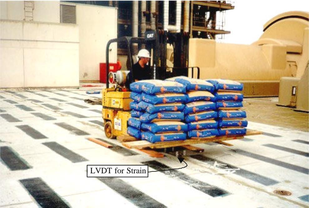
**Figure B.19: Forklift loaded with 36-100 lbs. (0.44 kN) sandbags**
