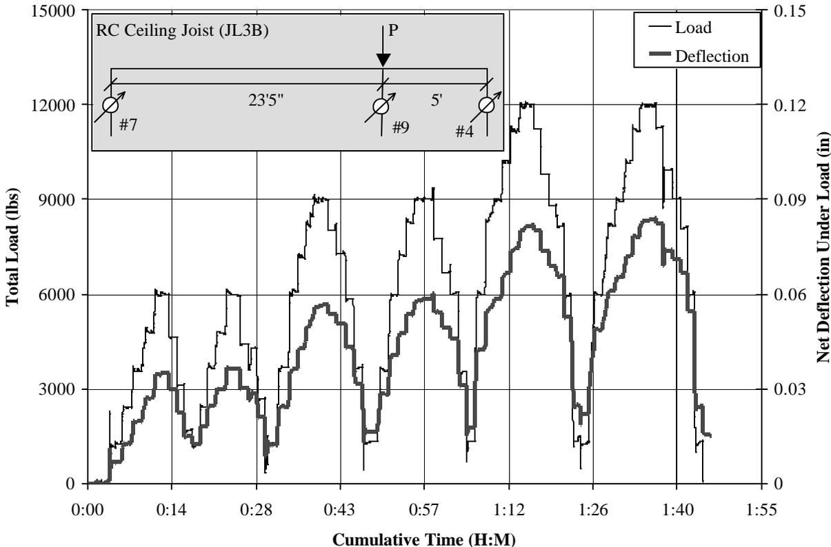
**Figure A.20: Time history of rapid load test for JL3B**
