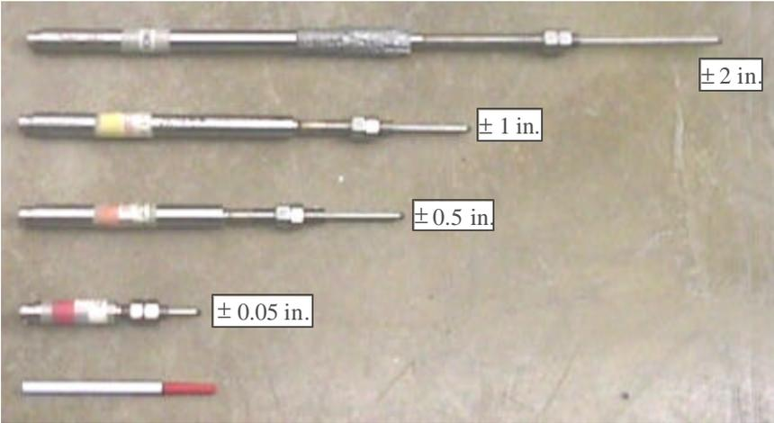
**Figure 2.19: LVDTs used to measure deflection**
