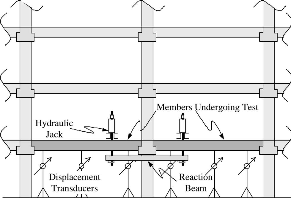
Figure 2.7: Closed loop test configuration
