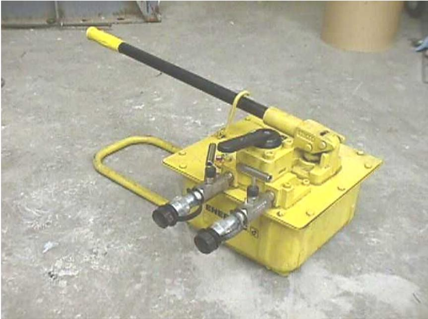
**Figure 2.17: Manual pump used to supply fluid to hydraulic jacks**
