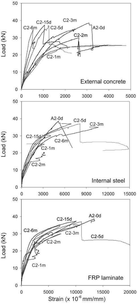
Figure 7 – Strains in G2 FRP-bonded beams
