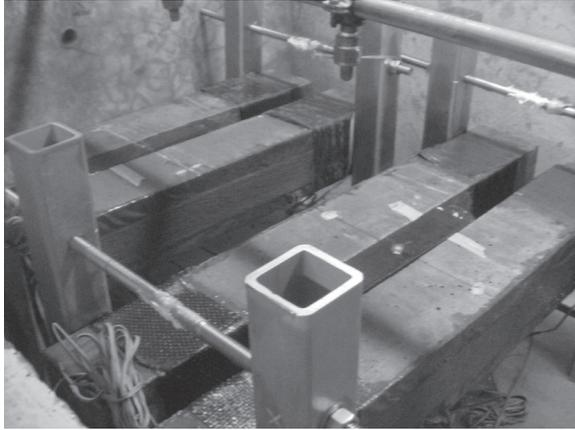
Figure 2 – Beams subjected to sustained loading inside weathering chamber
