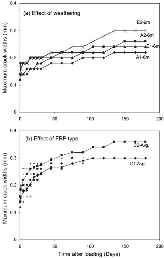
Figure 4 – Long-term crack widths
