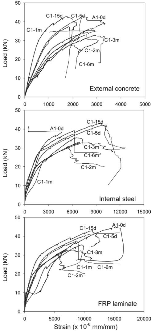
Figure 6 – Strains in G<sub>1</sub> FRP-bonded beams
