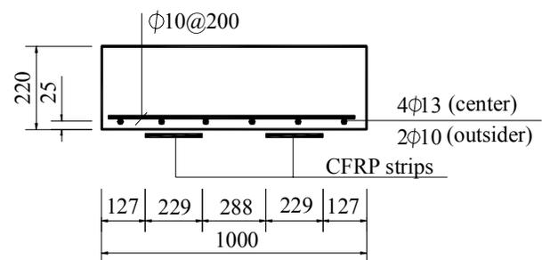
Figure 6. Slab cross-section A-A
