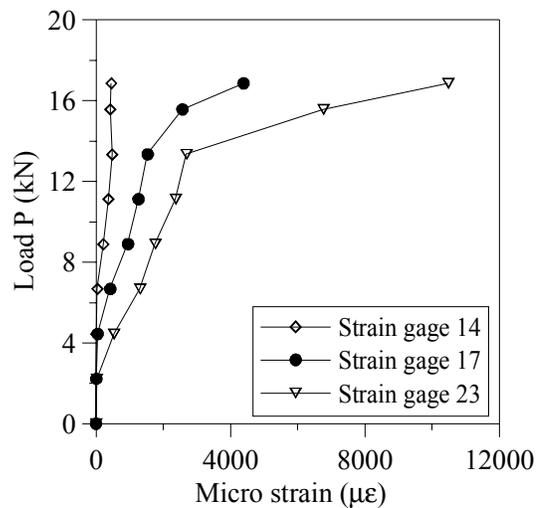
Figure 13. Strain of steel bars when testing to
