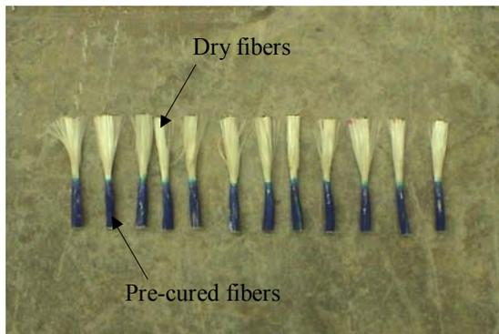
Figure 7. GFRP anchor spikes
