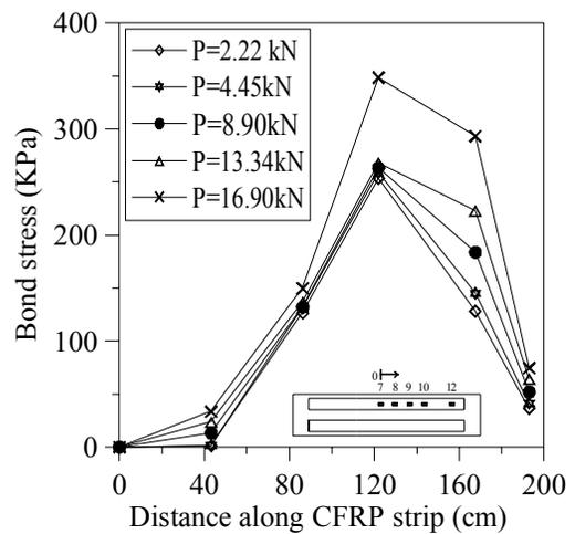
Figure 12. Bond stress along CFRP strip
