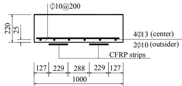
Figure 6. Slab cross-section A-A
