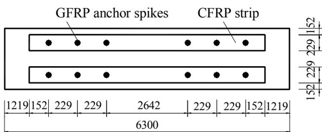
Figure 4. Location of GFRP anchor spikes
