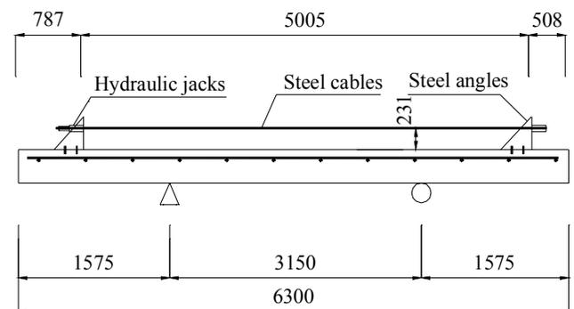
Figure 1. Test setup for prestressing
