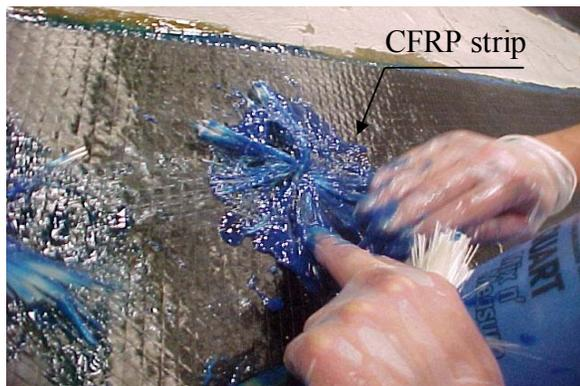
Figure 3. Splitting GFRP fibers
