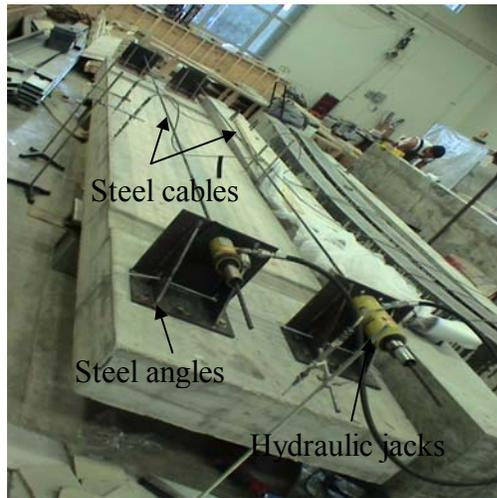
Figure 2. Concrete slab under prestressing
