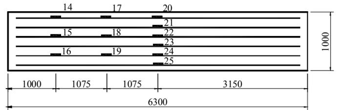
Figure 8. Location of strain gages on steel bars
