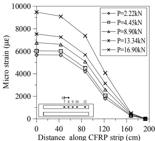
Figure 11. Strains of CFRP strip during testing to fail-
