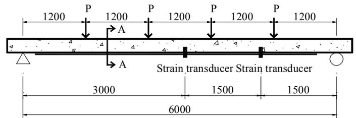
Figure 5. Test setup and location of strain transducers
