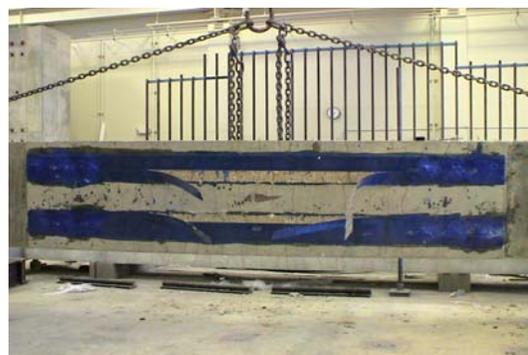
Figure 10. Rupture of CFRP strips at mid-span
