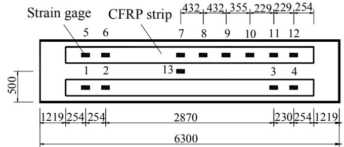
Figure 9. Location of strain gages on CFRP strips and concrete surface
