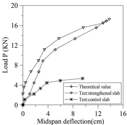
Figure 14. Comparison of mid-span deflection
