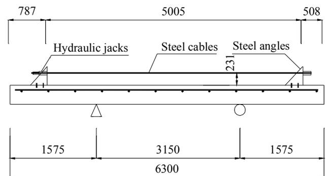
Figure 1. Test setup for prestressing
