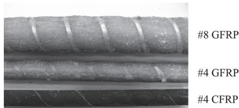
Fig. 1—Various FRP rods used in this study
