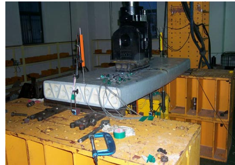
Figure 20. Deck under 3-point bending test
