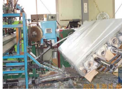
Figure 15. Filament winding process for face sheet
