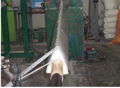
Figure 14. Filament winding process for triangular tube
