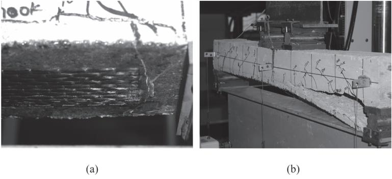
Figure 7 — Damage progression in specimen B-2-2-70; (a) crack initiation at end of CFRP laminate, and (b) concrete cover failure
