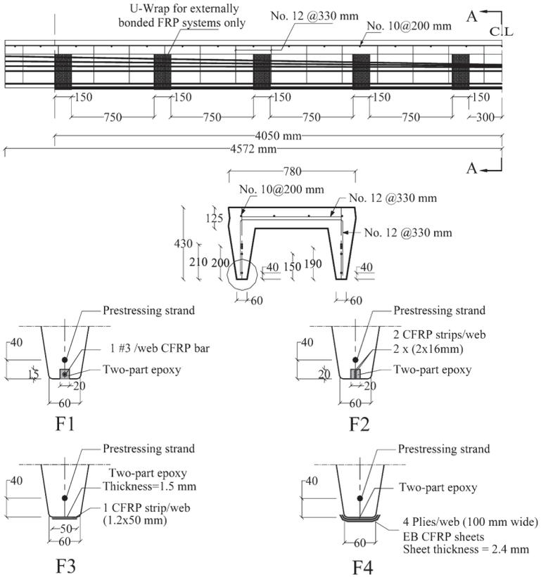
Figure 1 – Reinforcement and strengthening details of the C-Channel girders
