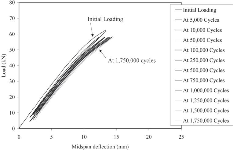
Figure 6 – Load versus deflection for girder strengthened with NSM bars (F1)
