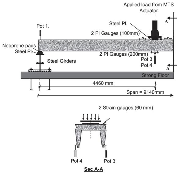
Figure 2 – Test setup for girders tested under fatigue loading conditions
