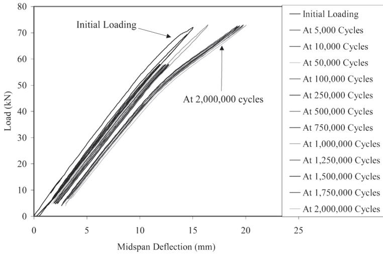
Figure 10 – Load versus deflection for girder strengthened with externally bonded sheets (F<sub>4</sub>)
