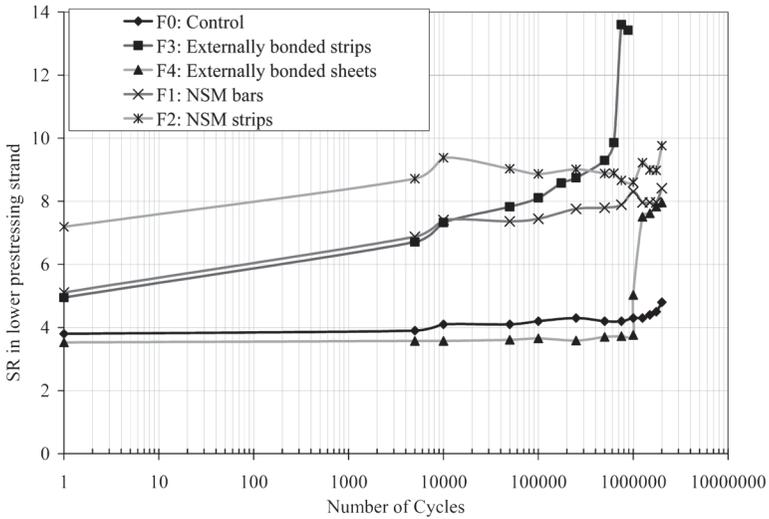
Figure 5 – Stress range versus the log of the number of cycles for girders tested in fatigue
