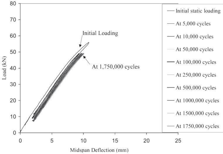
Figure 4 – Load versus deflection for control girder (Fo)
