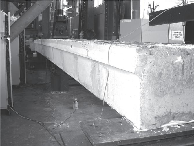
Figure 3 – Typical test setup for girders tested in fatigue
