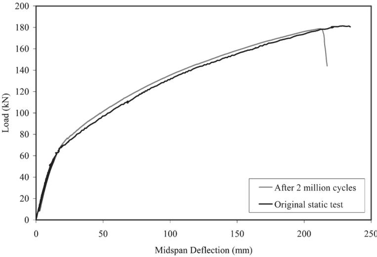
Figure 7 – Static test after two million cycles of girder F1
