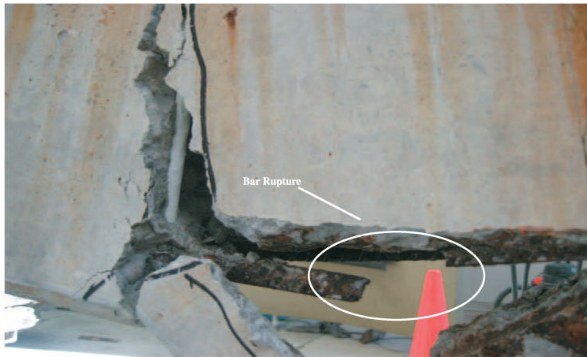
Fig. 6. Typical bar rupture of beams in group F (beam F-CD-72).
