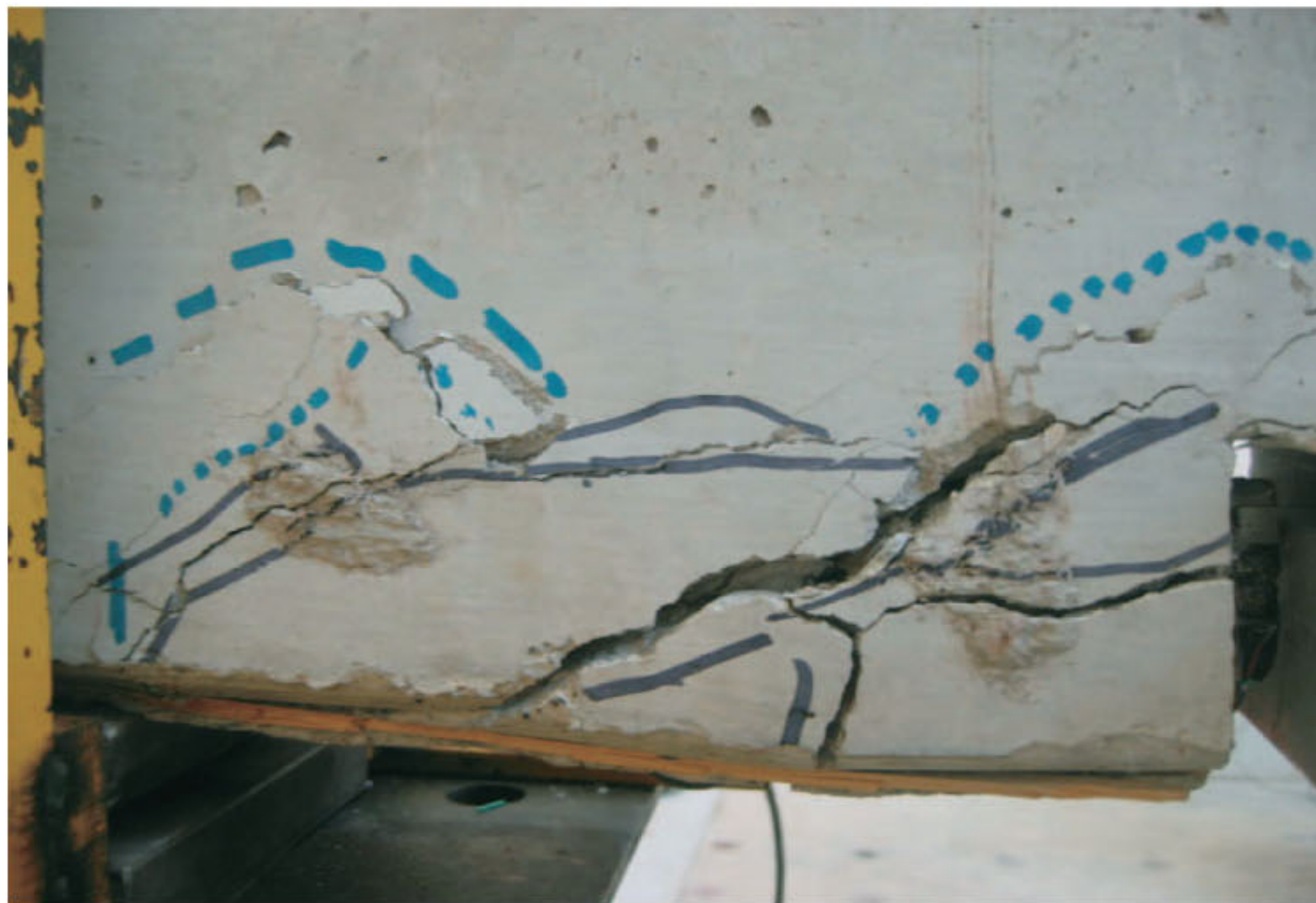
Fig. 7. Typical bond failure of beams in group B (beam B-C-55).
