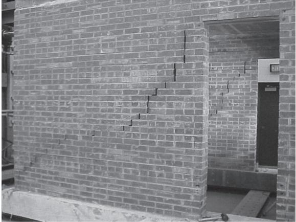
Figure 7 – Damaged incurred during experimental testing of the symmetric unreinforced brick structure.
