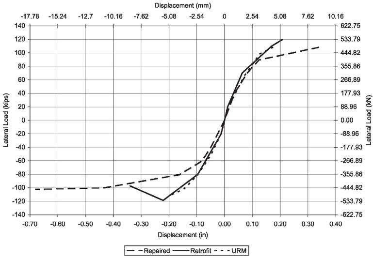
Figure 8 – Backbone curves for unreinforced, repaired and retrofitted symmetric brick structures.
