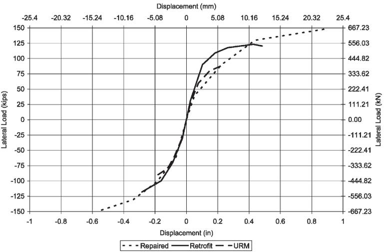
Figure 6 – Idealized backbone curve for the unreinforced, repaired and retrofitted symmetric CMU structures.
