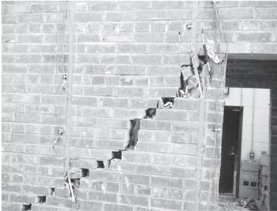
Figure 9 – Diagonal tension failure and GFRP NSM rod rupture of the symmetric retrofitted brick structure.
