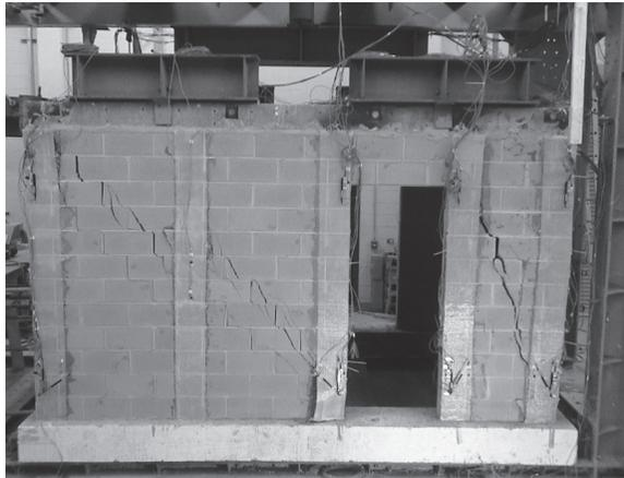
Figure 5 – Damage sustained during experimental load testing of the symmetric retrofitted CMU structure.
