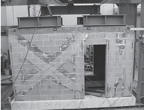
Figure 4 – GFRP composite layout for the repaired symmetric CMU structure.
