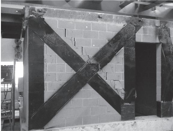
Figure 10 – Damaged induced by an applied 556 kN (125 kips) lateral force to a repaired asymmetric CMU structure.
