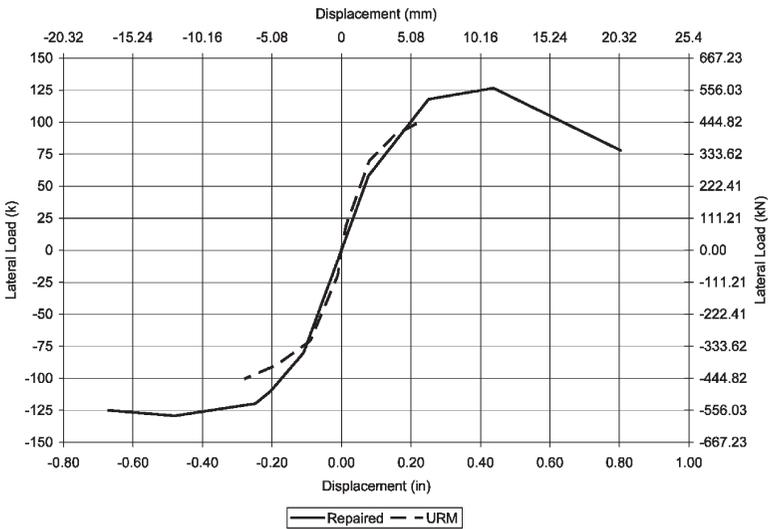
Figure 11 – Backbone curve comparison for asymmetric CMU structure in unreinforced and repaired condition.
