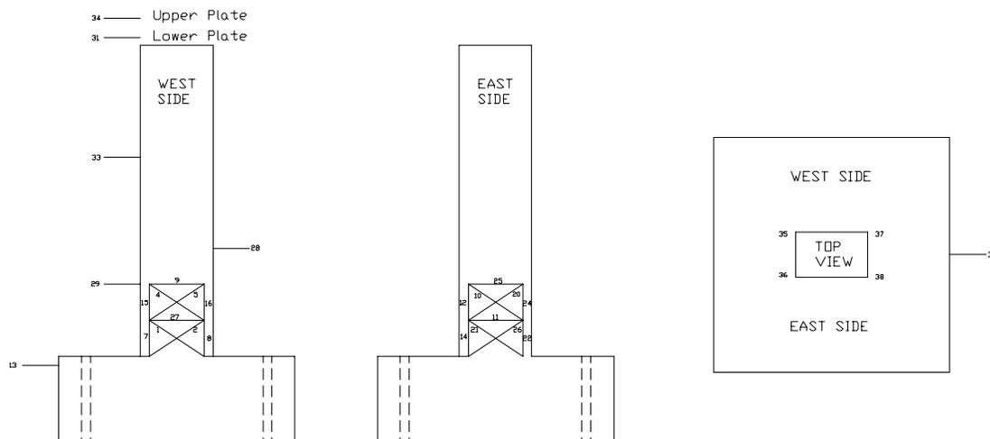
Figure 6: LVDTs location in the test specimen (PO1)
