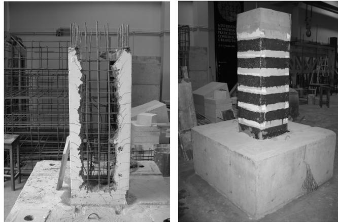
Figure 10: Hollow square section pier (PO1) before and after the shear retrofitting with CFRP sheet.
