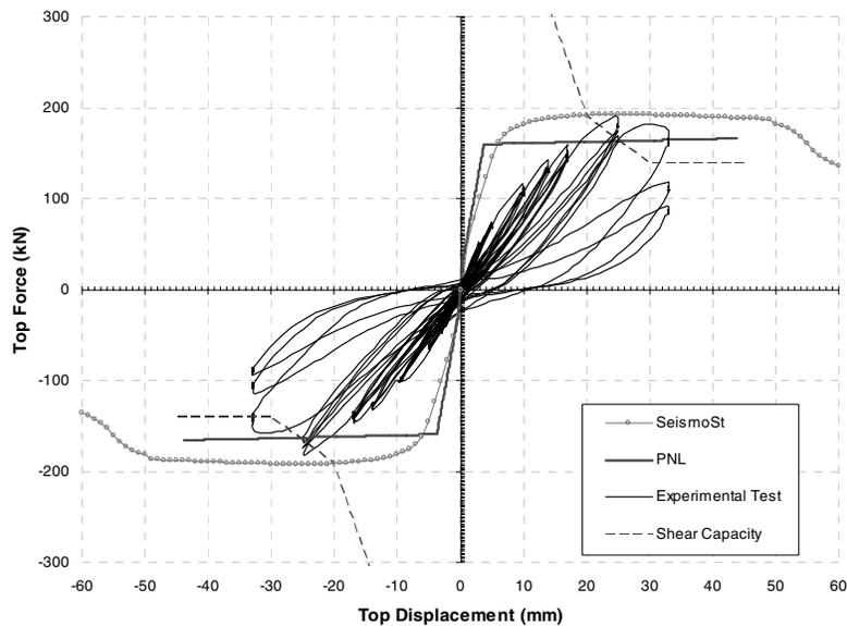
Figure 9: Experimental results and Seismostruct and PNL models monotonic predictions.
