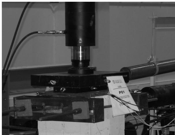
Figure 4: The slide device used to apply axial load
