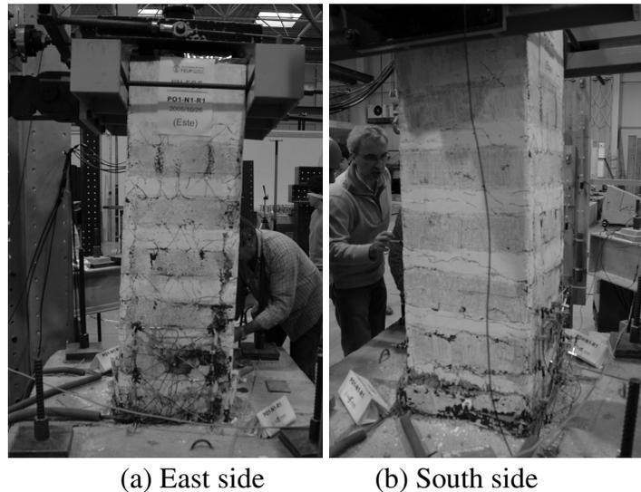
Figure 12: Final damage of the retrofitted pier PO1 for 3.2% drift.
