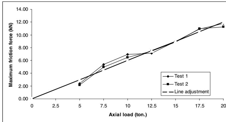
Figure 5: Relationship between the applied axial load and the maximum frictional force
