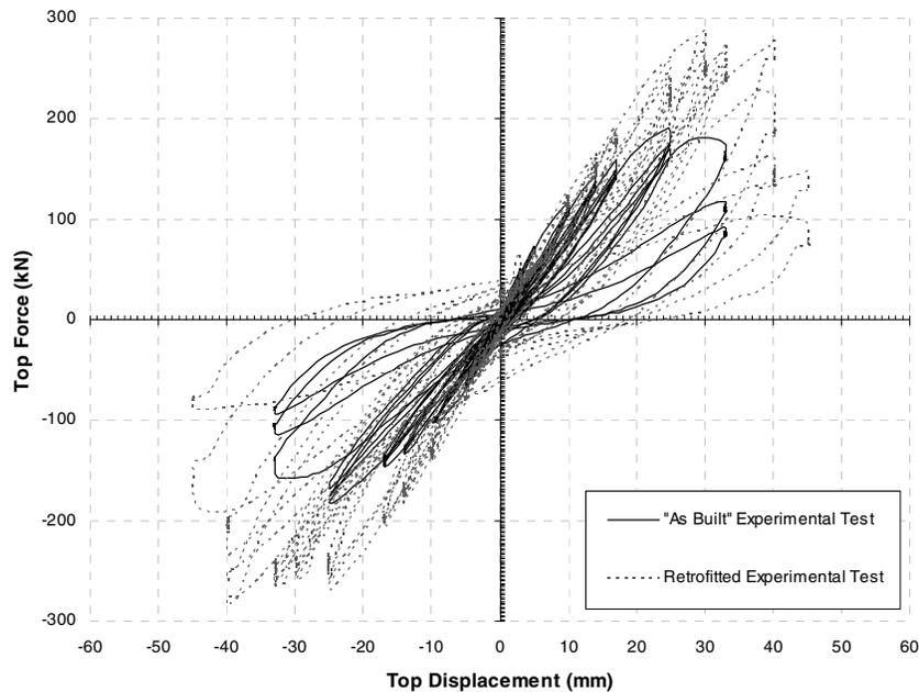
Figure 14: Experimental results of pier PO1 before and after retrofit.
