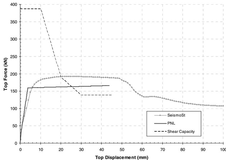
Figure 7: Monotonic numerical curves prediction.
