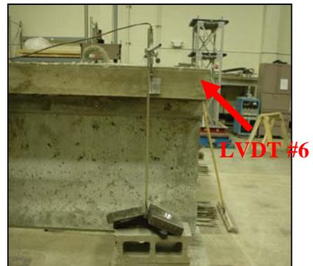
**Figure III-6-4- Stringer LVDTs and LVDTs positions**
