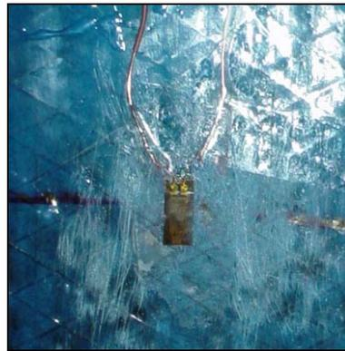
**Figure III-6-5 – Strain gage on CFRP detail**
