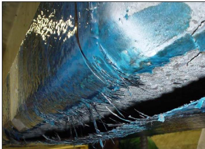
**Figure III-7-9** – *CFRP failure*
