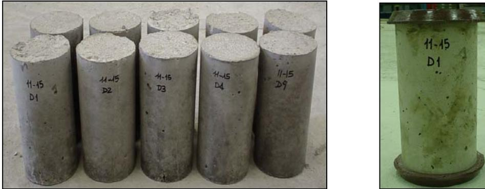
**Figure III-4-3** -Deck concrete cylinders
