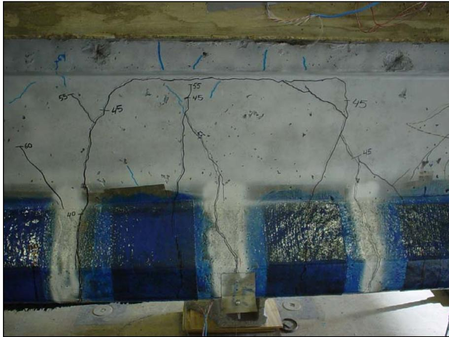
**Figure III-7-8**– *Cracks pattern*
