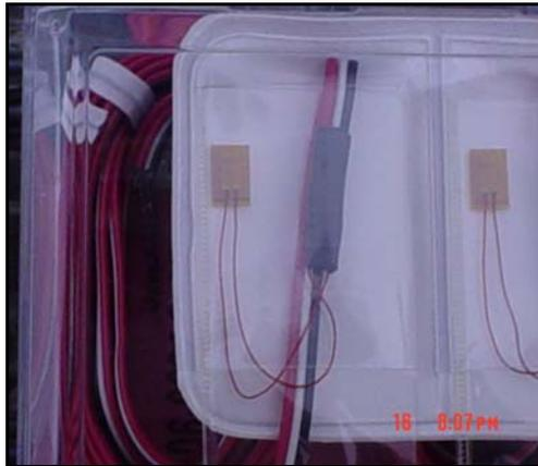
**Figure B-1-** *Strain gages characteristics: resistance  $350 \pm 0.5\%$ ; gage factor  $2.105 \pm 0.5\%$  transverse sensitivity at  $24^\circ \text{C} + 0.9 \pm 0.2\%$*
