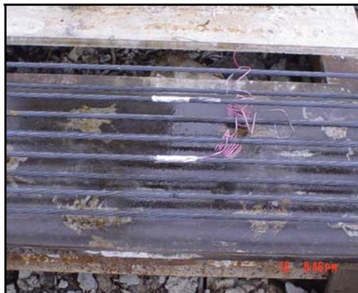
**Figure B-8-** *Location of strain gage applied on the undamaged girder*
