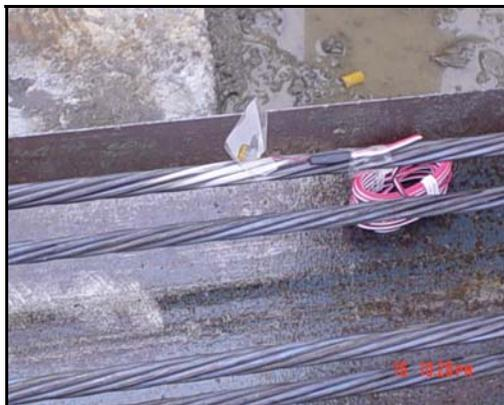
**Figure B-2-** *Application strain gages on the strands*
