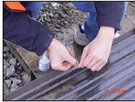
**FigureB-4-** *Strain gage installation*
