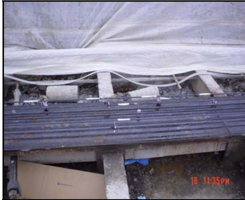
**Figure B-9-** *Location of strain gages applied on the intentionally damaged and repair girder*
