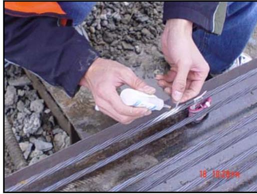
**Figure B-3-** *Strain gage installation*
