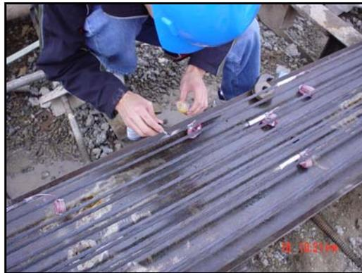
**Figure B 5-** *Strain gage installation*
