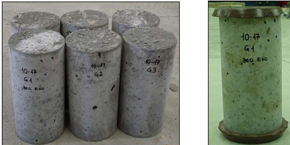
**Figure III-4-1-** *Girder Concrete cylinders*
