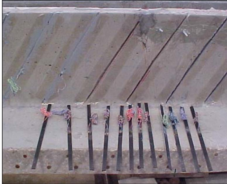
**Figure IV-2-4** – Instrumented bars for shear strengthening
