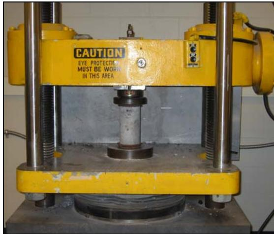
**Figure 4-2-** *Compression test under a Tinius Olsen Test machine*
