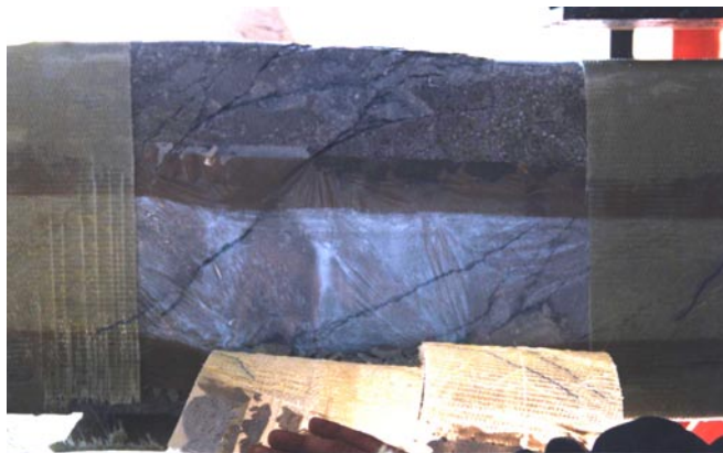
Figure 7: The beam ST2a at collapse
