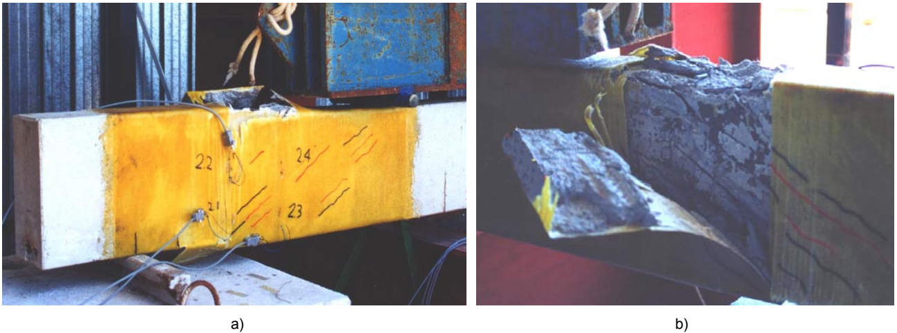
Figure 9: The beam ST3b at failure a) front view b) back view
