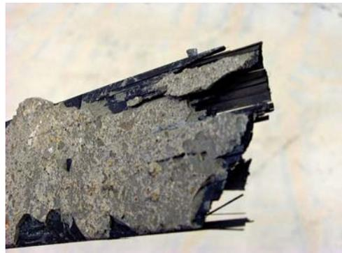
(e) Rupture of CFRP plate
