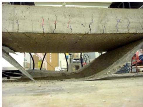
(a) Rupture of Carbon fiber sheet
