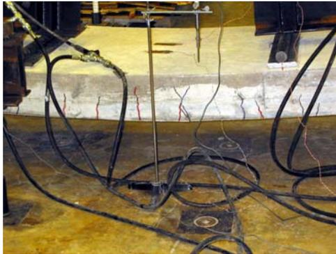
(a) Flexural failure
