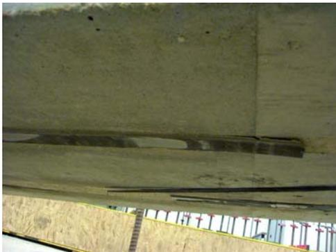
(c) Rupture of CFRP plates
