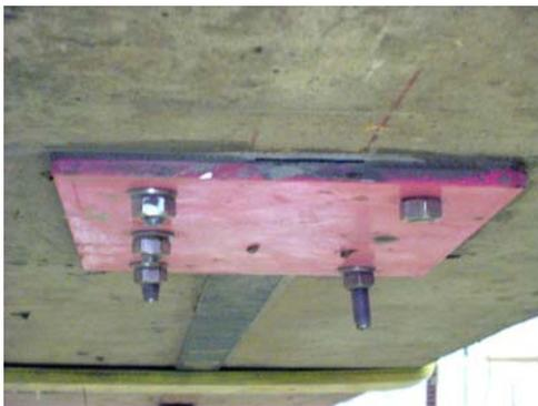
(a) Anchorage failure
