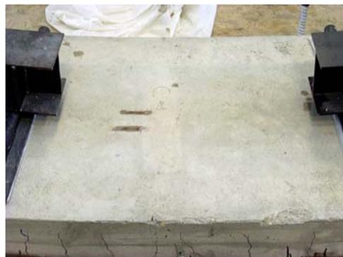
(b) No sign of concrete crushing
