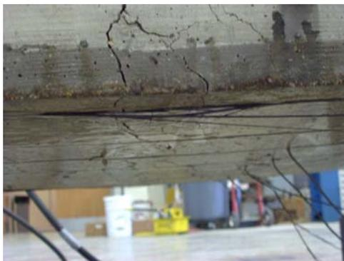
(c) Rupture of CFRP bars
