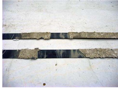
(b) A relatively layer of concrete attached to the plates
