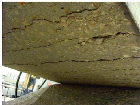
(b) Cracks at the substrate of the slab
