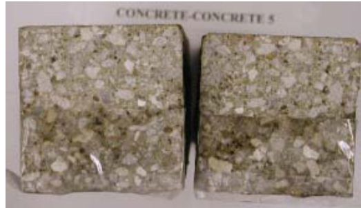
Figure 12. Fractured surfaces of concrete-concrete bonded interface
