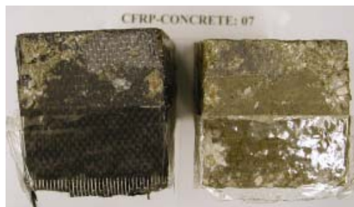
Figure 10. Fractured surfaces of concrete-CFRP bonded interface
