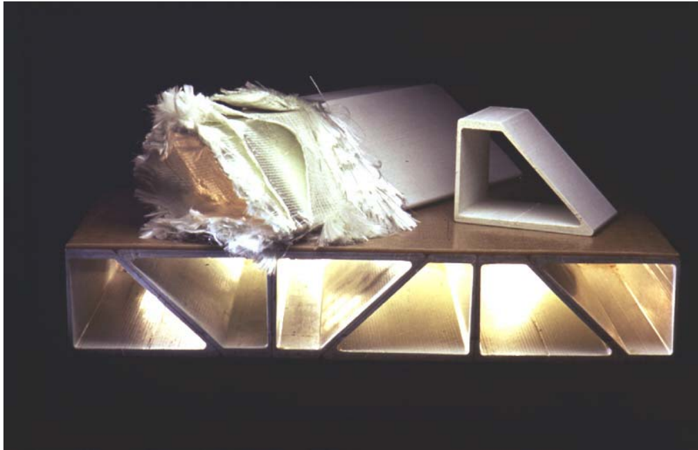
Figure 1: Trapezoidal tubes used to form FRP deck
