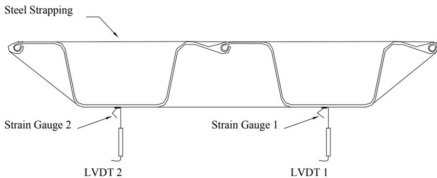
Figure 2: Cross section of connected double panels
