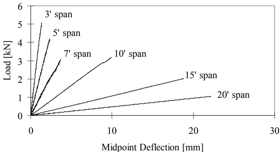
Figure 3: Typical load-deflection curves at the midpoint for four-point bending linear tests (single panel, 1' = 0.3048m)
