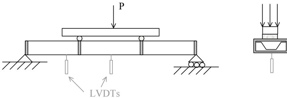
(b) Four-point bending set-up for both single and double panel tests
