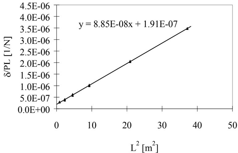
Fig. 4: Straight line used to determine the flexural rigidity from four-point bending based on the midpoint deflection (single panel)
