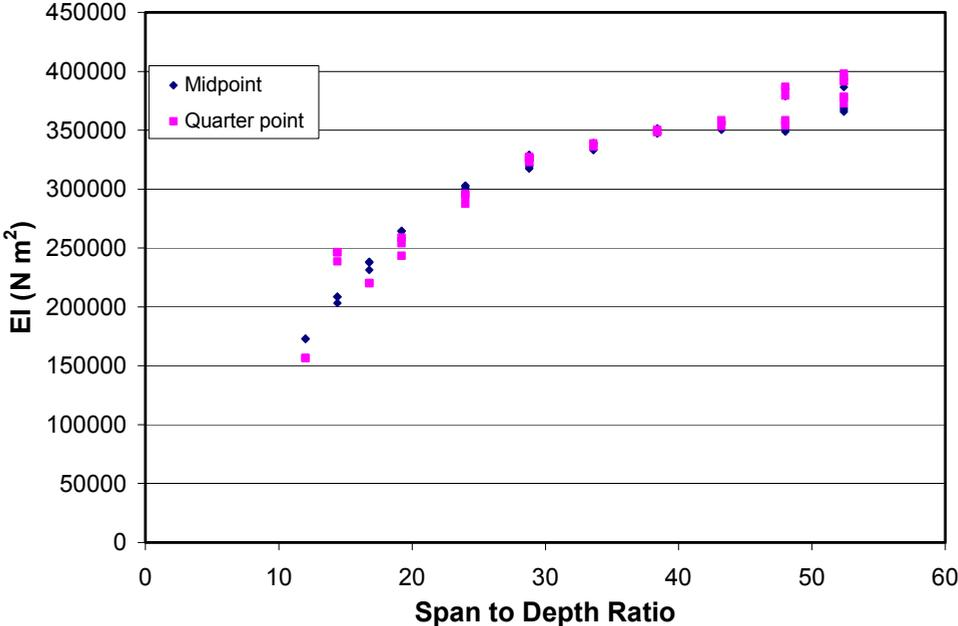
Fig. 7: Apparent flexural rigidities versus span-to-depth ratio (connected panels)
