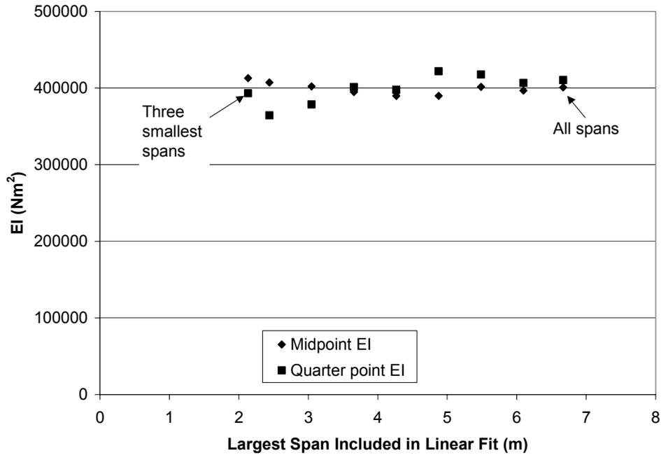
Figure 8: Sensitivity of EI on largest span included in linear fit (connected panels)
