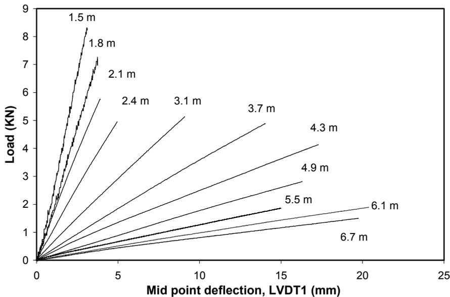
Figure 5: Typical load – deflection curves at the midpoint for four-point bending linear tests (LVDT 1, connected double panels)
